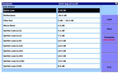
Figure 5.2.6.1-1 Thresholds Screen (Auto Detect)
