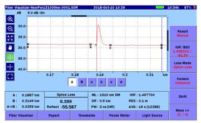
Figure 5.6.1-4 Fiber Visualizer Trace Screen (Manual)
