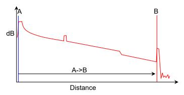
Figure 8.1.1.1-1 Location of Cursors for Fiber Length Measurement
