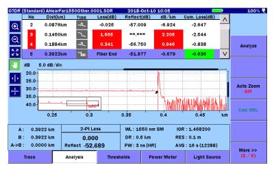
Figure 4.6-1 OTDR (Standard) Analysis Screen
