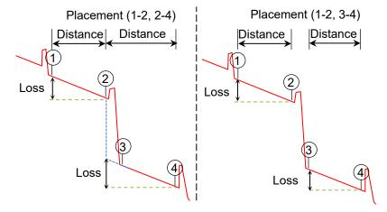
Figure 5.2.3-4 Display of Distance and Loss Between Markers
