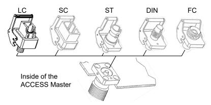
Figure 2.6.1-2 Connector Types
