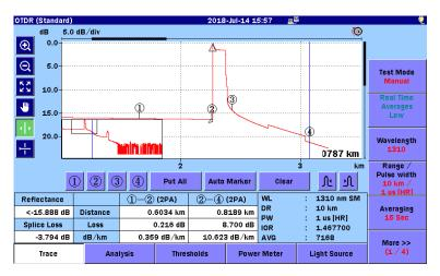
Figure 8.2.3-3 Reflectance Measurements (Points Before and After Reflectance)
