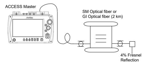
Figure 15.3.4-1 Connection Diagram
