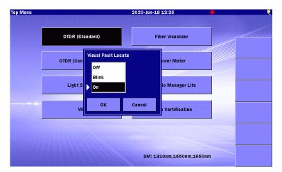
Figure 1.2.9-1 Visual Fault Locate Dialog Box
