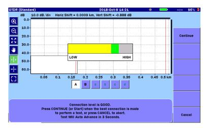
Figure 4.5.6-1 Connection Check Screen
