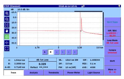
Figure 8.1.2.5-1 dB/km Loss Measurement Screen
