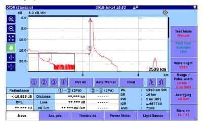
Figure 8.2.3-1 Reflectance Measurements (Rising Point Only)
