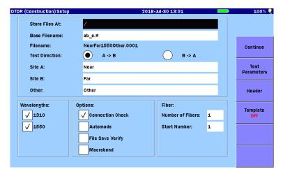
Figure 6.1-1 OTDR (Construction) Setup Screen
