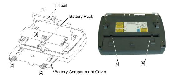
Figure 2.2.1-1 Installing the Battery Pack
