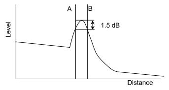
Figure 15.3.6-2 Cursor Position to Measure Fresnel Dead Zone
