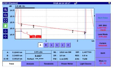
Figure 8.1.2.4-1 2-Pt LSA Measurement Screen
