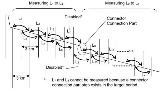
Figure 15.3.5-2 How to Measure Linearity
