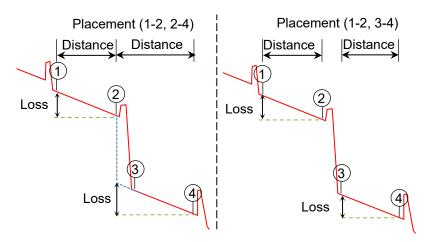
Figure 7.2.3-4 Display of Distance and Loss Between Markers
