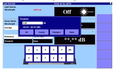
Figure 9.4.2-3 Entering Threshold
