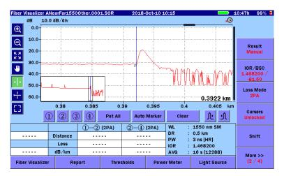
Figure 5.4-2 Fiber Visualize Trace Screen (Manual)
