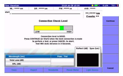
Figure 5.4.1-1 Connection Check Screen
