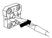
Figure 16.1-3 Cleaning the Ferrule End Surface
