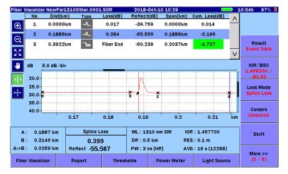
Figure 5.6.1-3 Fiber Visualizer Trace Screen
