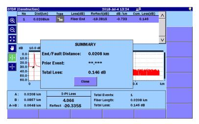
Figure 1.2.4-1 OTDR (Construction) Analysis Screen
