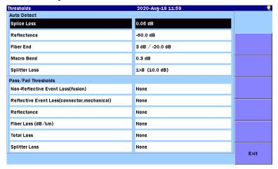
Figure 4.2.7-1 Thresholds Screen
