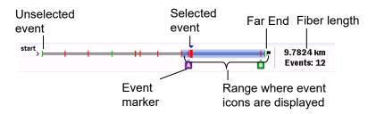
Figure 5.3.1-1 Fiber Schematic
