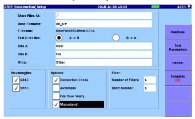
Figure 6.3-1 OTDR (Construction) Setup Screen
