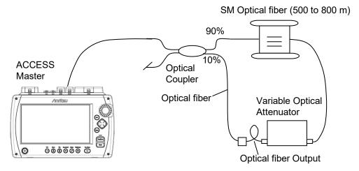
Figure 15.3.6-1 Connection Diagram
