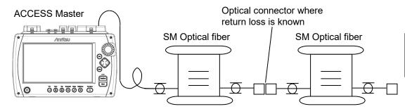
Figure 15.4.1-1 Connection Diagram
