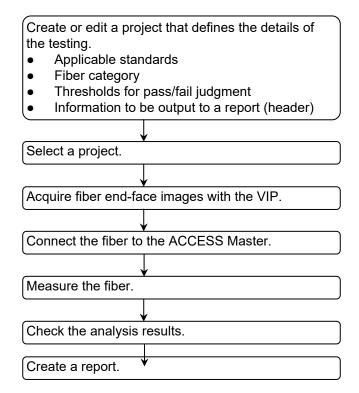
Figure 7.1-1 Flow of Cable Certification Testing
