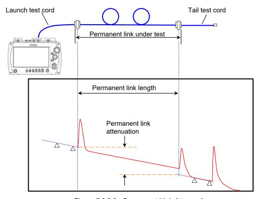
Figure 7.3.2-3 Permanent Link Attenuation
