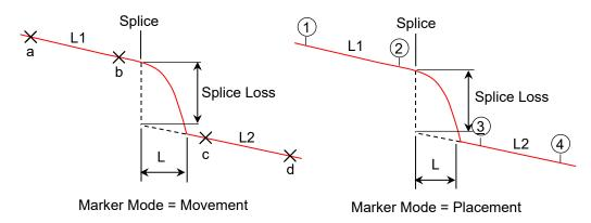
Figure B.2-2 Measurement Principle of Splice Loss
