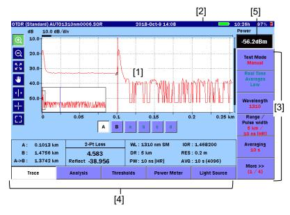
Figure 4.5-1 OTDR (Standard) Trace Screen
