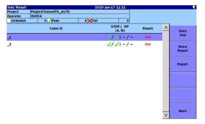
Figure 1.2.5-2 Test/Result Screen of Cable Certification
