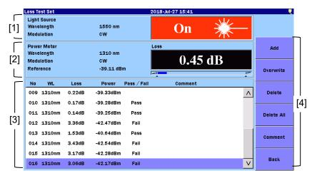
Figure 9.5-1 Loss Table Screen (Loss Test Set)
