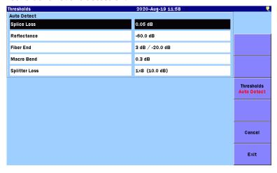
Figure 7.3.5.1-1 Thresholds Screen (Auto Detect, Applicable Standards: Manual)
