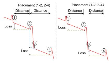
Figure 6.2.3-4 Display of Distance and Loss Between Markers
