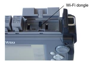
Figure 12.2.2-1 Dongle Connection
