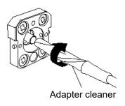
Figure 16.1-2 Cleaning the Ferrule End Surface
