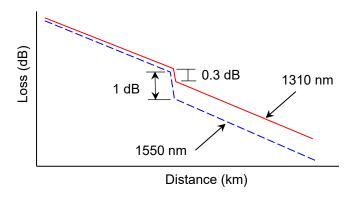
Figure 4.10.1-2 Example of Macro bend Detection
