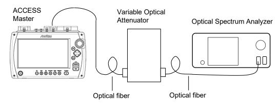
Figure 15.3.1-1 Connection Diagram
