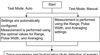
Trace processing and fault locating (Auto detection of events) The ACCESS Master averages the trace, locates faults, calculates data of faults, and then displays the event table on the screen.
