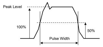
Figure 15.3.2-2 Pulse Width Measurement
