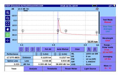
Figure 8.2.2-1 Splice Loss Measurements
