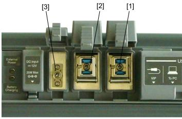
Figure 1 Locations of Laser Beam Apertures
