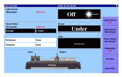
Figure 1.2.6-1 Loss Test Set Screen
