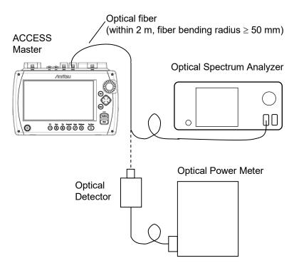
Figure 15.3.8-1 Connection Diagram
