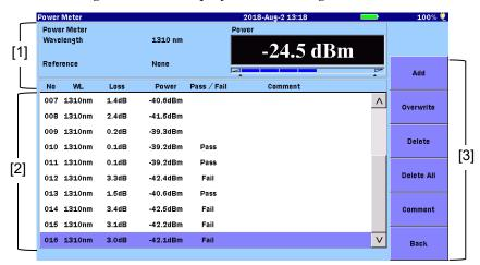
Figure 10.2-1 Loss Table Screen (Power Meter)
