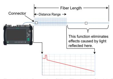
Figure 6.2.2-2 Processing of When Fiber Length Check is On
