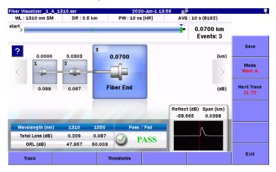
Figure 7.4.1-4 OTDR Test Results
