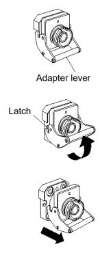
Figure 16.1-1 Removing the Optical Adapter
