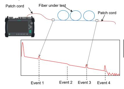
Figure 5.2.3-5 Auto Patch-cord Removal Example
