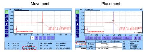
Figure 15.4.1-3 Reflectance Location on the Screen
