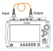
Figure 9.6.1-1 Connection to Verify Patch Cord
