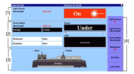
Figure 9.4-1 Loss Test Set Screen
