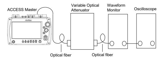
Figure 15.3.2-1 Connection Diagram
