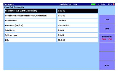
Figure 5.2.6.2-1 Thresholds Screen (Pass/Fail Thresholds)
