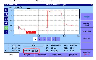
Figure 8.1.3.2-2 Manual Reflectance Calculation Screen
