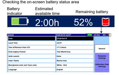
Figure 2.2.3-2 Checking the Remaining Battery
