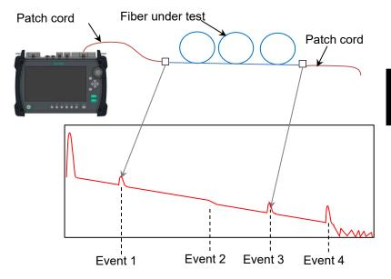
Figure 4.2.3-5 Auto Patch-cord Removal Example
