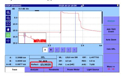
Figure 8.1.3.1-2 Auto Reflectance Measurement Screen
