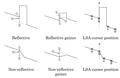
Figure 8.1.2.2-1 Points to Measure Splice Loss
