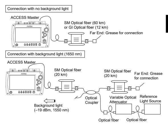
Figure 15.3.3-1 Connection Diagram
