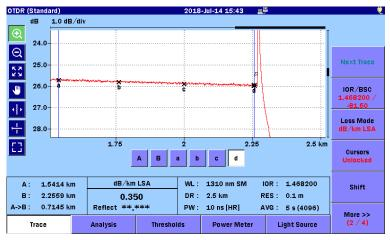
Figure 8.1.2.6-1 dB/km LSA Measurement
