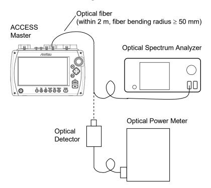
Figure 15.3.7-1 Connection Diagram
