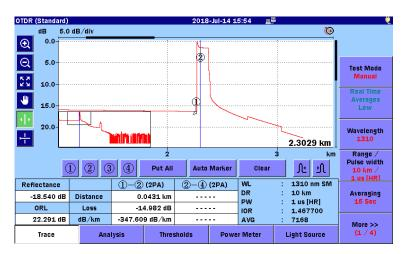
Figure 8.2.3-2 Reflectance Measurements (Rising Point and Peak Point)
