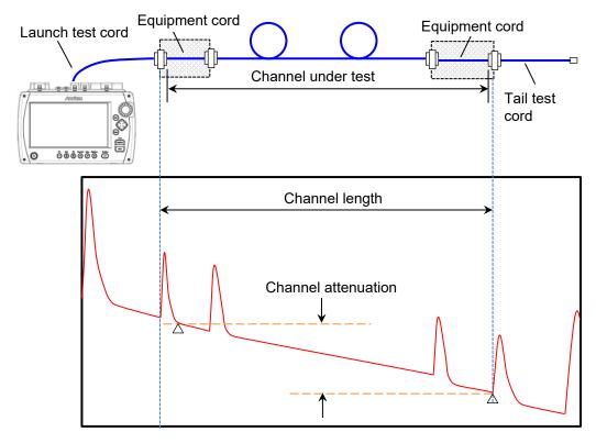
Figure 7.3.2-2 Channel Attenuation
