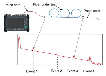
Figure 7.2.3-5 Auto Patch-cord Removal Example
