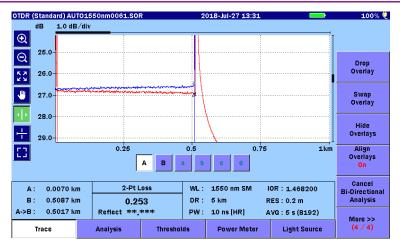
Figure 4.11.3-2 Example of Bi-Directional Analysis Results
