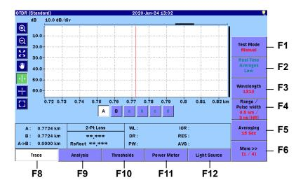
Figure 2.7.2-1 Mapping Between Softkeys and USB Keyboard Keys
