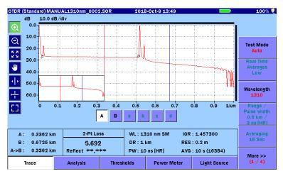
Figure 1.2.2-1 OTDR (Standard) Trace Screen
