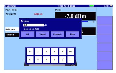
Figure 10.3.3-1 Entering Threshold
