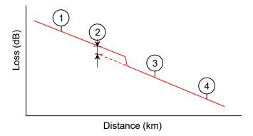
Figure 4.5.5-2 Splice Loss
