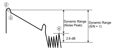
Figure 15.3.3-2 How to Measure Dynamic Range
