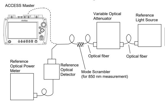
Figure 15.3.9-1 Connection Diagram
