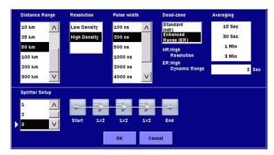
Figure 5.5.1-4 Test Parameters Dialog Box
