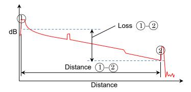
Figure 8.2.1-1 Distance and Loss Measurement between Two Points
