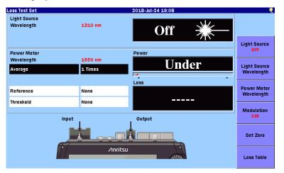
Figure 9.2-1 Initial Loss Test Set Screen
