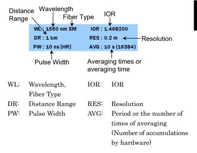
Test parameters for the primary trace are displayed for a trace recalled from a file.
