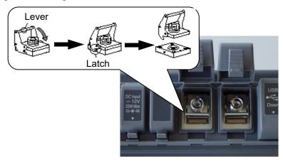
Figure 2.6.1-1 Replaceable Connector
