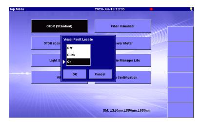
Figure 1.2.9-1 Visual Fault Locate Dialog Box
