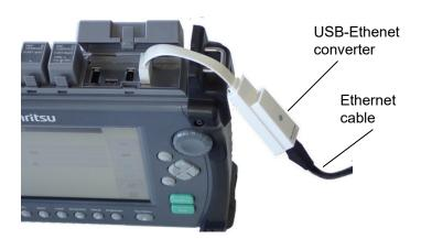
Figure 12.2.1-1 Ethernet Cable Connection
