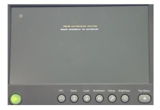
Figure 3.3.4-3 Touch Panel Calibration Screen
