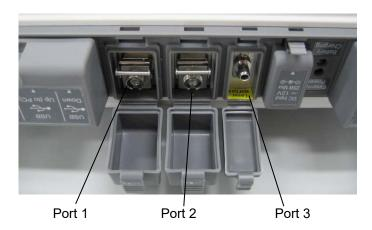
Figure 2.4-1 Connecting the Optical Fibers
