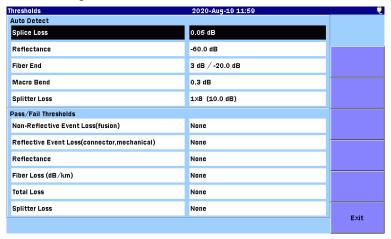
Figure 4.2.7-1 Thresholds Screen
