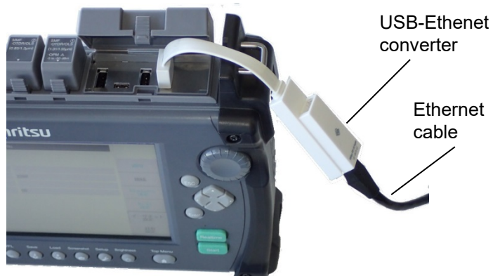
Figure 12.2.1-1 Ethernet Cable Connection
