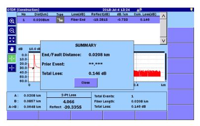
Figure 1.2.4-1 OTDR (Construction) Analysis Screen
