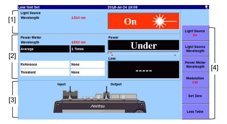
Figure 8.4-1 Loss Test Set Screen
