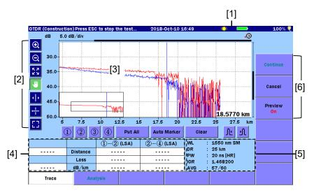
Figure 6.5-2 Test In Progress Screen
