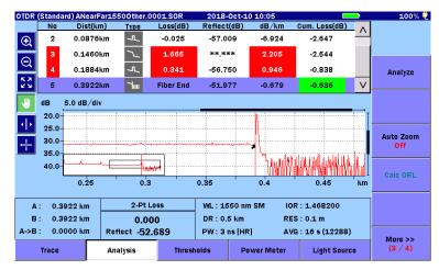
Figure 4.6-1 OTDR (Standard) Analysis Screen
