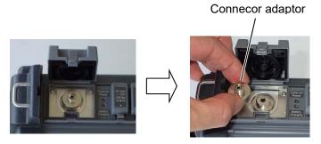
Figure 2.6.2-1 Optical Connector Part
