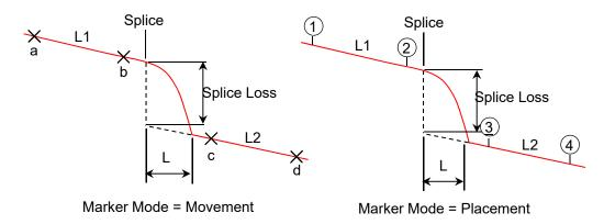
Figure B.2-2 Measurement Principle of Splice Loss
