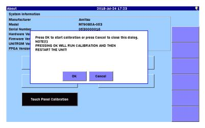
Figure 3.3.4-2 Confirmation Dialog Box for Touch Panel Calibration
