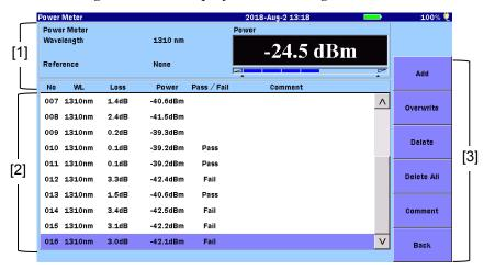
Figure 9.2-1 Loss Table Screen (Power Meter)
