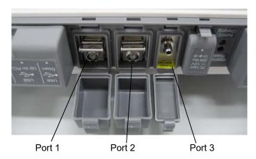
Figure 2.4-1 Connecting the Optical Fibers
