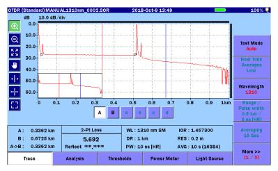
Figure 1.2.2-1 OTDR (Standard) Trace Screen
