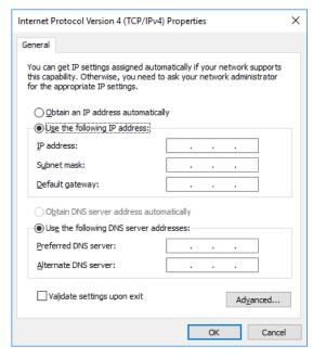
6. Assign an IP address that is different from the one set for the ACCESS Master. Here, configure as follows and click **OK**:
