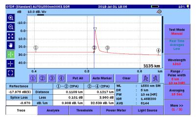
Figure 7.2.2-1 Splice Loss Measurements
