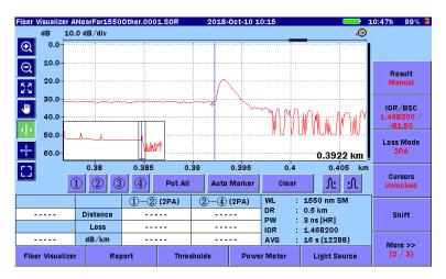
Figure 5.4-2 Fiber Visualize Trace Screen (Manual)
