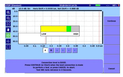
Figure 4.5.6-1 Connection Check Screen
