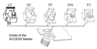
Figure 2.6.1-2 Connector Types
