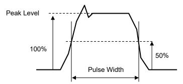
Figure 14.3.2-2 Pulse Width Measurement
