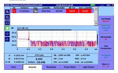
Figure 4.10.2-1 Analysis Screen for All Wavelengths
