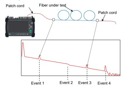
Figure 5.2.3-5 Auto Patch-cord Removal Example
