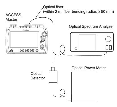
Figure 14.3.8-1 Connection Diagram
