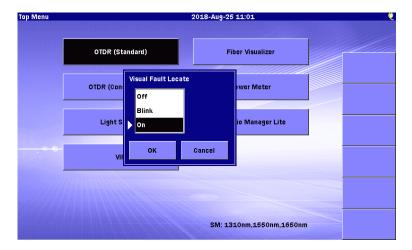
Figure 1.2.8-1 Visual Fault Locate Dialog Box
