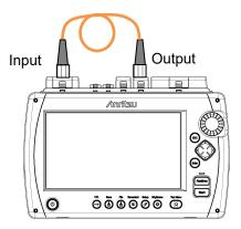
Figure 8.6.1-1 Connection to Verify Patch Code
