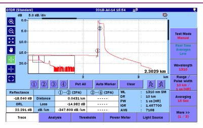
Figure 7.2.3-2 Reflectance Measurements (Rising Point and Peak Point)
