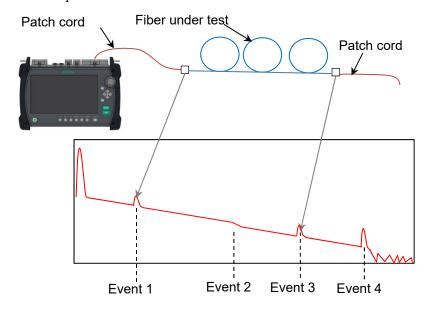
Figure 6.2.3-5 Auto Patch-cord Removal Example
