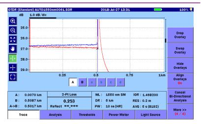
Figure 4.11.3-2 Example of Bi-Directional Analysis Results
