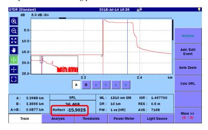
Figure 7.1.3.1-2 Auto Reflectance Measurement Screen
