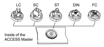
Figure 2.6.2-2 Connector Types
