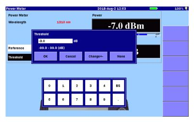
Figure 9.3.3-1 Entering Threshold
