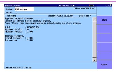
After the update is complete successfully, the ACCESS Master restarts automatically. Make sure that the firmware has been updated on the **About** screen described in Figure 3.3.4-1 "About Screen".
