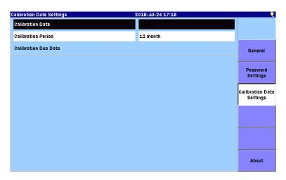
Figure 3.3.3-1 Calibration Date Settings Screen
