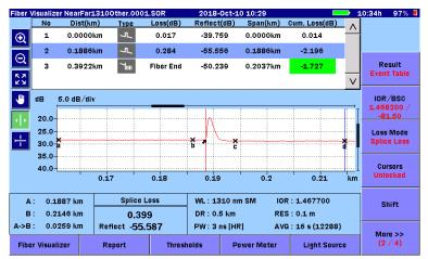
Figure 5.6.1-3 Fiber Visualizer Trace Screen
