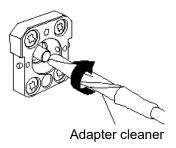
Figure 15.1-2 Cleaning the Ferrule End Surface
