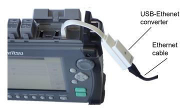
Figure 11.2.1-1 Ethernet Cable Connection
