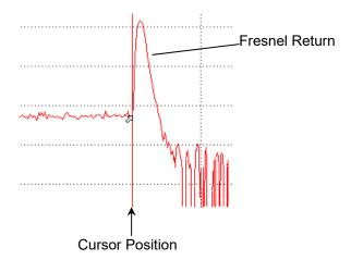
Figure 14.3.4-2 Cursor Placement for Distance Measurement Accuracy Test
