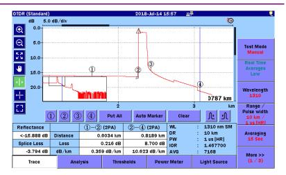
Figure 7.2.3-3 Reflectance Measurements (Points Before and After Reflectance)
