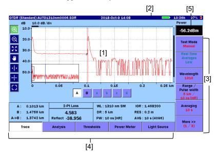
Figure 4.5-1 OTDR (Standard) Trace Screen
