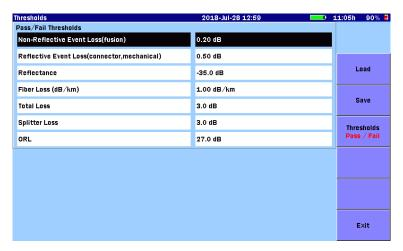
Figure 5.2.6.2-1 Thresholds Screen (Pass/Fail Thresholds)
