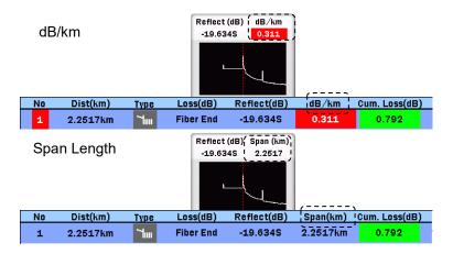
Figure 5.2.3-6 Display of Event Table Span Calculation
