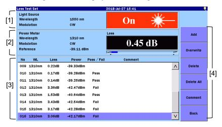
Figure 8.5-1 Loss Table Screen (Loss Test Set)
