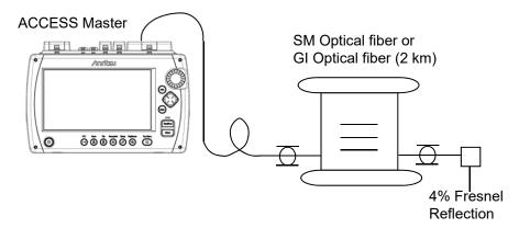
Figure 14.3.4-1 Connection Diagram
