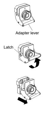
Figure 15.1-1 Removing the Optical Adapter
