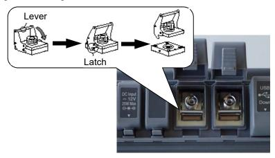
Figure 2.6.1-1 Replacable Connector
