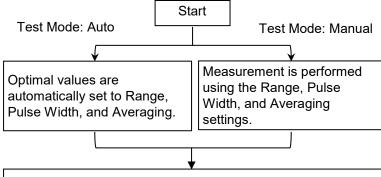
Trace processing and fault locating (Auto detection of events) The ACCESS Master averages the trace, locates faults, calculates data of faults, and then displays the event table on the screen.
