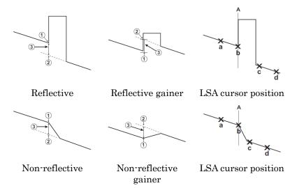
Figure 7.1.2.2-1 Points to Measure Splice Loss
