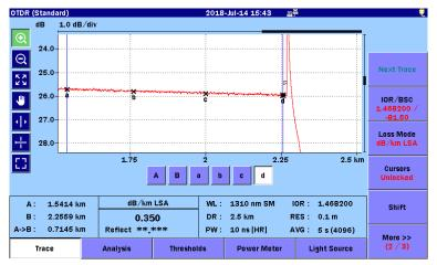
Figure 7.1.2.6-1 dB/km LSA Measurement
