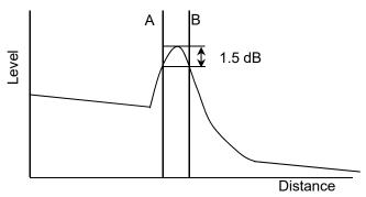
Figure 14.3.6-2 Cursor Position to Measure Fresnel Dead Zone
