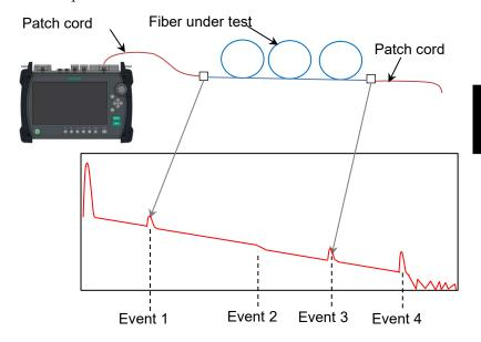
Figure 4.2.3-5 Auto Patch-cord Removal Example
