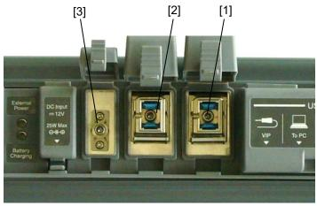
Figure 1 Locations of Laser Beam Apertures
