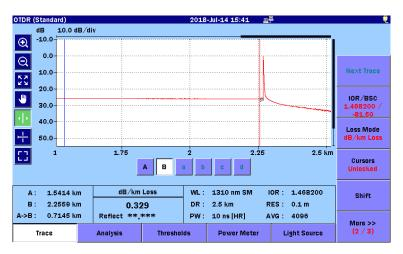
Figure 7.1.2.5-1 dB/km Loss Measurement Screen
