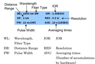
Test parameters for the primary trace are displayed for a trace recalled from a file.
