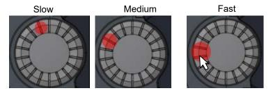
Figure 11.4.1-2 Rotary Knob Speed Display
