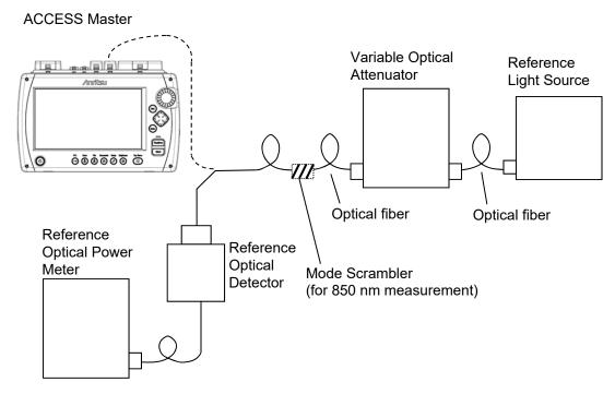
Figure 14.3.9-1 Connection Diagram
