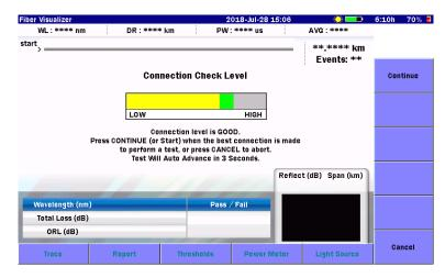
Figure 5.4.1-1 Connection Check Screen
