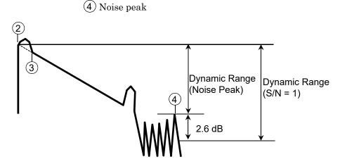
Figure 14.3.3-2 How to Measure Dynamic Range
