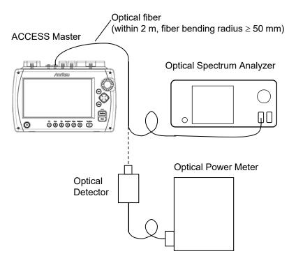
Figure 14.3.7-1 Connection Diagram
