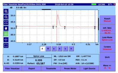
Figure 5.6.1-4 Fiber Visualizer Trace Screen (Manual)
