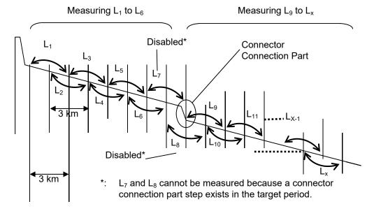
Figure 14.3.5-2 How to Measure Linearity
