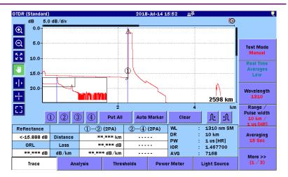
Figure 7.2.3-1 Reflectance Measurements (Rising Point Only)
