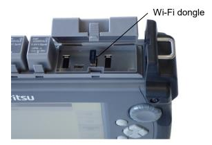
Figure 11.2.2-1 Dongle Connection
