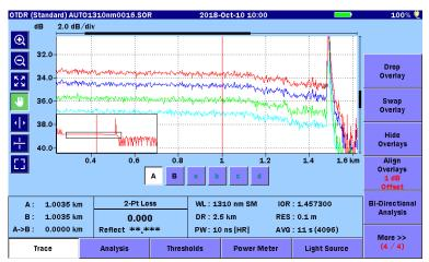
Figure 4.11.2-2 Align Overlays 1 dB Offset
