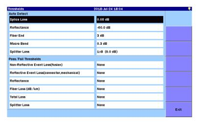
Figure 4.2.7-1 Thresholds Screen
