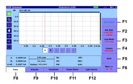
Figure 2.7.2-1 Mapping Between Softkeys and USB Keyboard Keys
