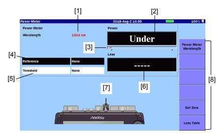
Figure 9.1.2-1 Power Meter Screen
