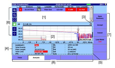
Figure 6.6-1 Test Results screen with Summary Closed
