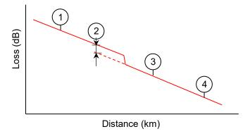
Figure 4.5.5-2 Splice Loss
