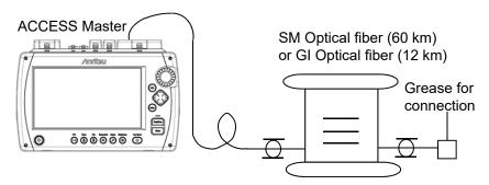
Figure 14.3.5-1 Connection Diagram
