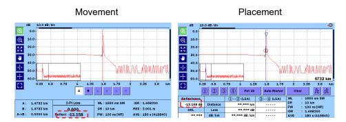
Figure 14.4.1-3 Reflectance Location on the Screen
