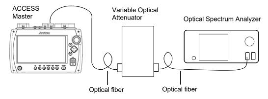
Figure 14.3.1-1 Connection Diagram
