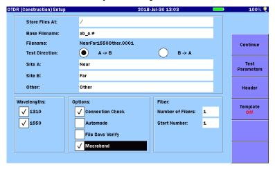
Figure 6.3-1 OTDR (Construction) Setup Screen
