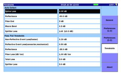
Figure 6.2.4-1 Thresholds Screen
