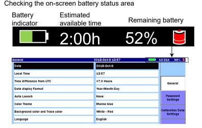
Figure 2.2.3-2 Checking the Remaining Battery
