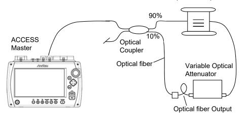
Figure 14.3.6-1 Connection Diagram
