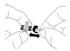
Figure 15.1-4 Cleaning an Optical Adapter
