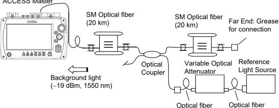
Figure 14.3.3-1 Connection Diagram
