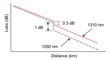
Figure 4.10.1-2 Example of Macro bend Detection
