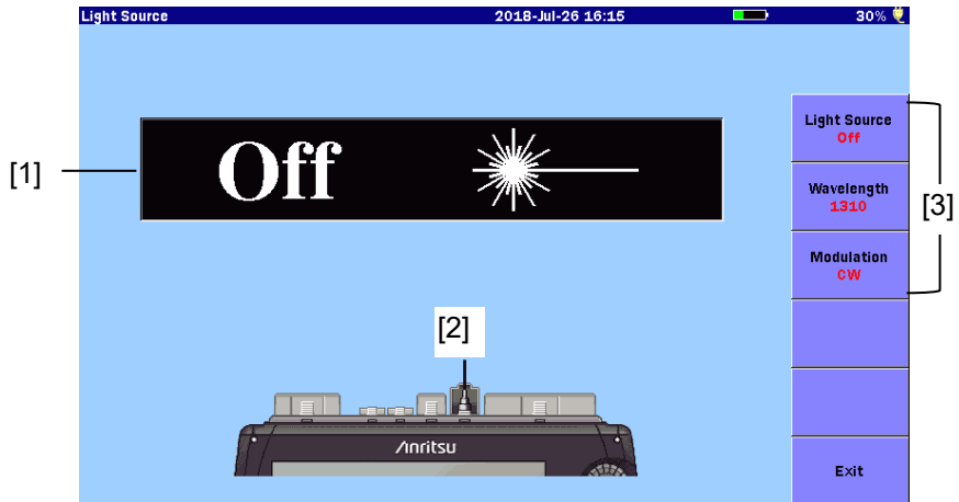
Figure 4.11.3-1 Light Source Screen
