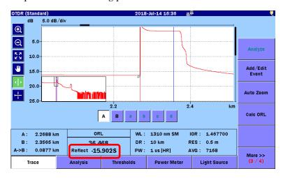
Figure 8.1.3.1-2 Auto Reflectance Measurement Screen
