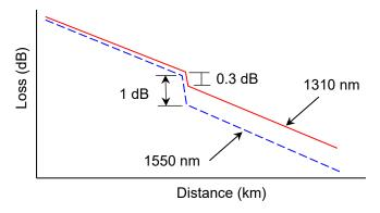
Figure 4.10.1-2 Example of Macro bend Detection
