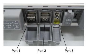
Figure 2.4-1 Connecting the Optical Fibers
