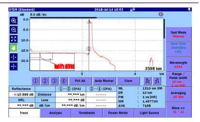
Figure 8.2.3-1 Reflectance Measurements (Rising Point Only)
