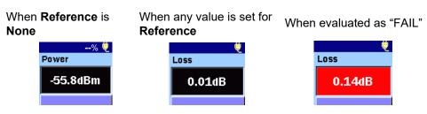
Figure 4.12-2 Display of Measured Power
