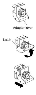
Figure 16.1-1 Removing the Optical Adapter
