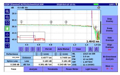
Figure 4.11-1 Trace Screen with Trace Overlay Softkeys
