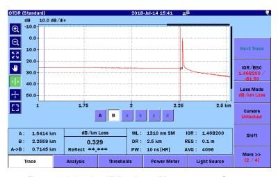
Figure 8.1.2.5-1 dB/km Loss Measurement Screen
