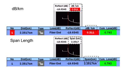
Figure 7.2.3-6 Display of Event Table Span Calculation
