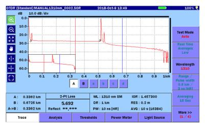
Figure 1.2.2-1 OTDR (Standard) Trace Screen
