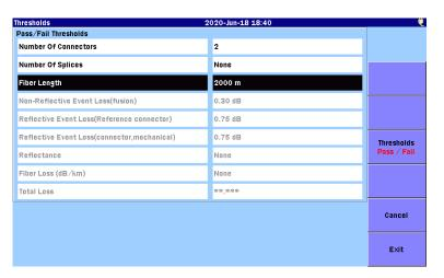
Figure 7.3.5.2-2 Thresholds Screen (Pass/Fail Thresholds, Applicable Standards: ISO/IEC 11801-3:2017)
