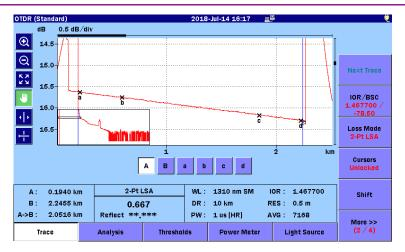
Figure 8.1.2.4-1 2-Pt LSA Measurement Screen
