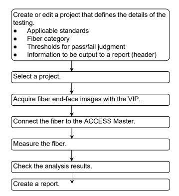
Figure 7.1-1 Flow of Cable Certification Testing
