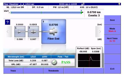
Figure 7.4.1-4 OTDR Test Results
