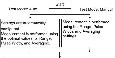
Trace processing and fault locating (Auto detection of events) The ACCESS Master averages the trace, locates faults, calculates data of faults, and then displays the event table on the screen.
