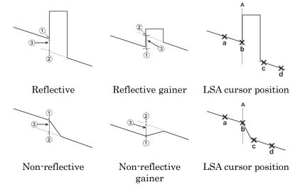
Figure 8.1.2.2-1 Points to Measure Splice Loss
