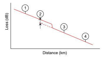
Figure 4.5.5-2 Splice Loss
