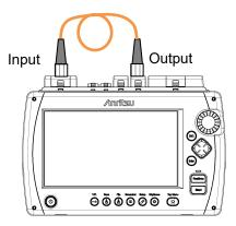
Figure 9.6.1-1 Connection to Verify Patch Code
