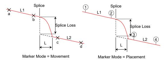
Figure B.2-2 Measurement Principle of Splice Loss
