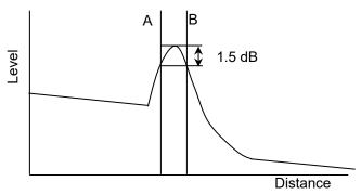
Figure 15.3.6-2 Cursor Position to Measure Fresnel Dead Zone
