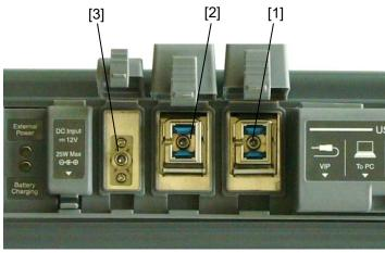
Figure 1 Locations of Laser Beam Apertures
