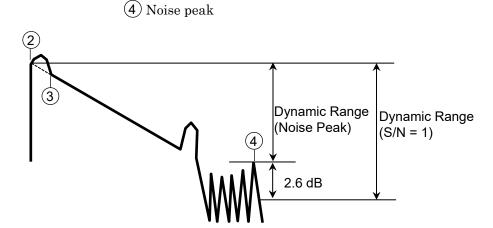
Figure 15.3.3-2 How to Measure Dynamic Range
