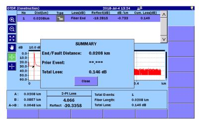
Figure 1.2.4-1 OTDR (Construction) Analysis Screen
