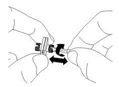
Figure 16.1-4 Cleaning an Optical Adapter
