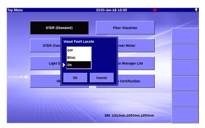
Figure 1.2.9-1 Visual Fault Locate Dialog Box
