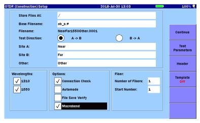
Figure 6.3-1 OTDR (Construction) Setup Screen
