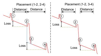
Figure 4.2.3-4 Display of Distance and Loss Between Markers
