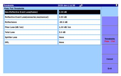
Figure 7.3.5.2-1 Thresholds Screen (Pass/Fail Thresholds, Applicable Standards: Manual)
