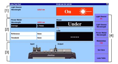
Figure 9.4-1 Loss Test Set Screen
