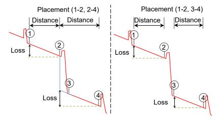
Figure 6.2.3-4 Display of Distance and Loss Between Markers
