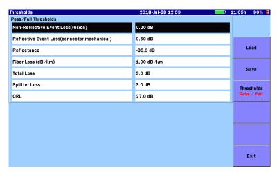
Figure 5.2.6.2-1 Thresholds Screen (Pass/Fail Thresholds)
