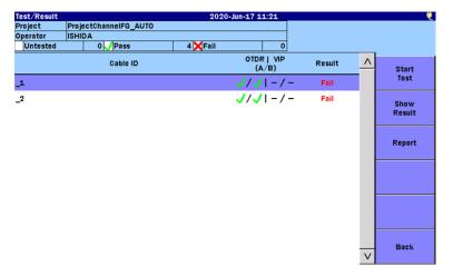
Figure 1.2.5-2 Test/Result Screen of Cable Certification
