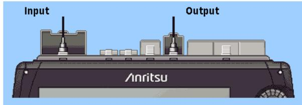
Figure 9.4.3-1 Port Connection Indicator (Loss Test Set)
