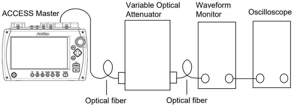
**Figure 15.3.2-1 Connection Diagram**
