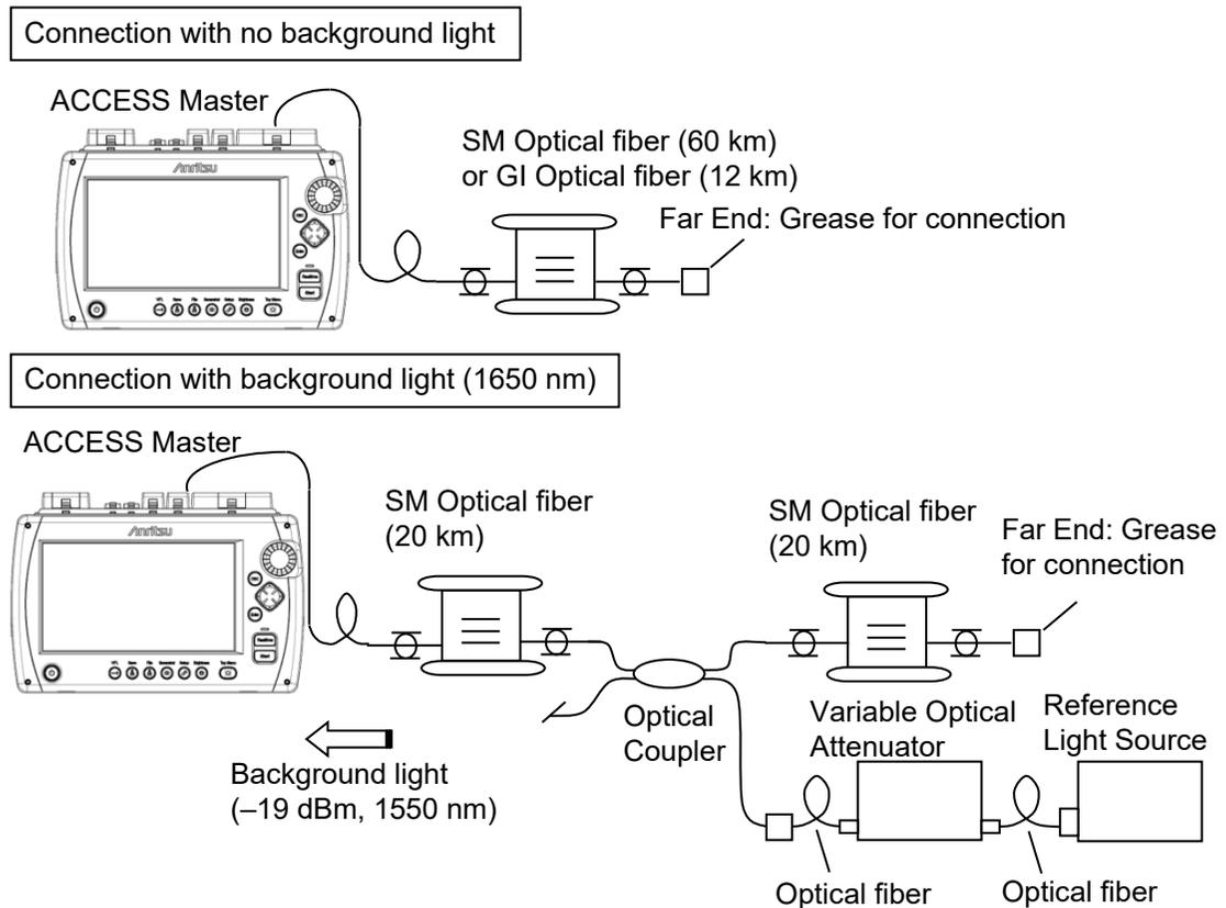
Figure 15.3.3-1 Connection Diagram
