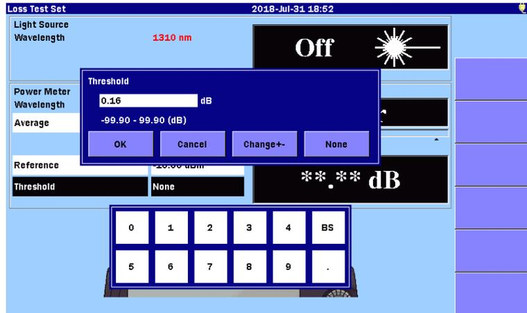
Figure 9.4.2-3 Entering Threshold
