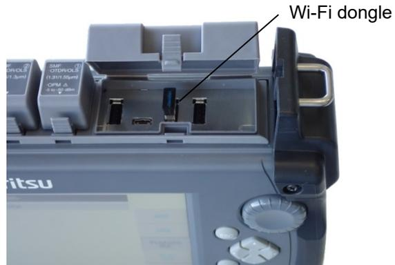
Figure 12.2.2-1 Dongle Connection
