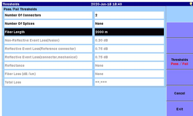
Figure 7.3.5.2-2 Threshholds Screen (Pass/Fail Thresholds, Applicable Standards: ISO/IEC 11801-3:2017)
