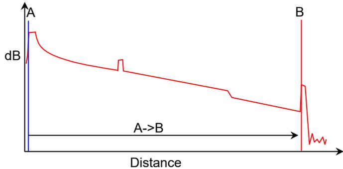
**Figure 8.1.1.1-1 Location of Cursors for Fiber Length Measurement**
