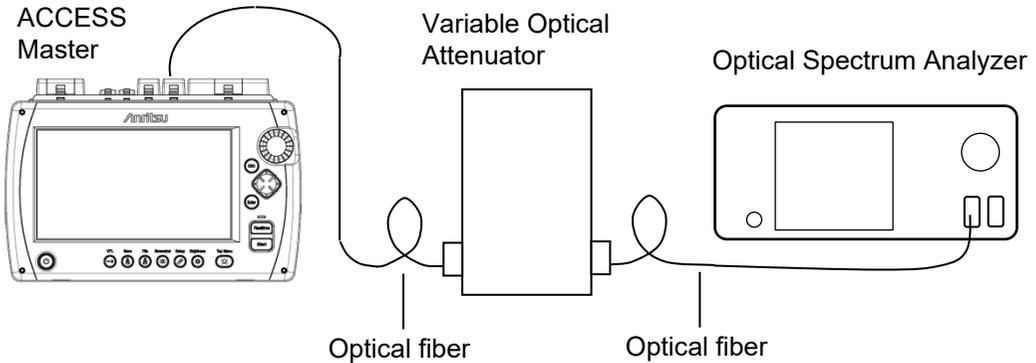
Figure 15.3.1-1 Connection Diagram
