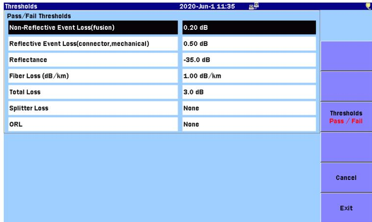
Figure 7.3.5.2-1 Threshholds Screen (Pass/Fail Thresholds, Applicable Standards: Manual)
