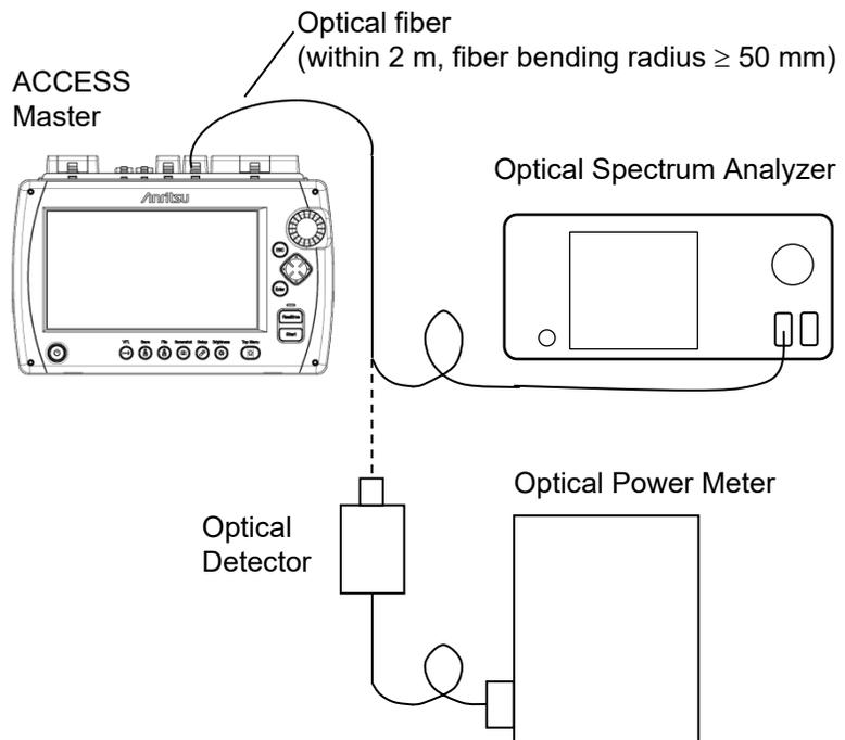
**Figure 15.3.8-1 Connection Diagram**
