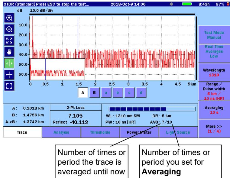
Figure 4.4-1 OTDR (Standard) Mode Screen—Measurement In Progress
