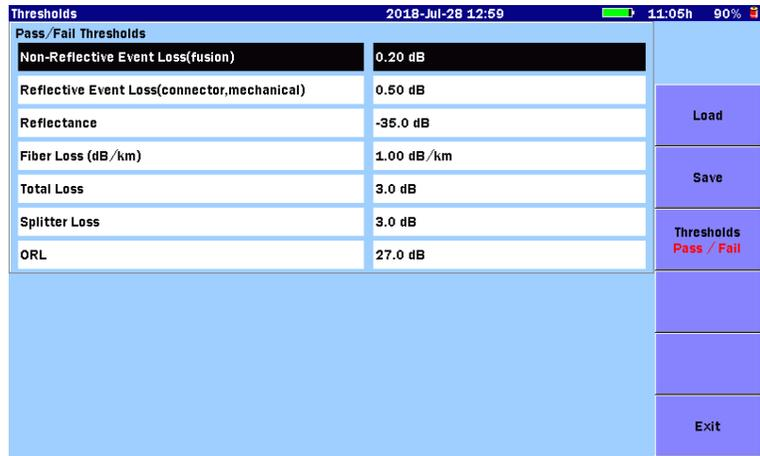
Figure 5.2.6.2-1 Thresholds Screen (Pass/Fail Thresholds)
