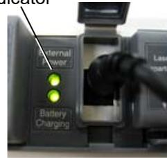
4. Leave the AC adapter connected until the battery is fully charged. Charging ends in about 6 hours and the Battery Charging lamp goes off. The battery is, however charged 90% or more after 5 hours.
