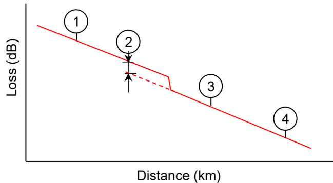
**Figure 4.5.5-2 Splice Loss**
