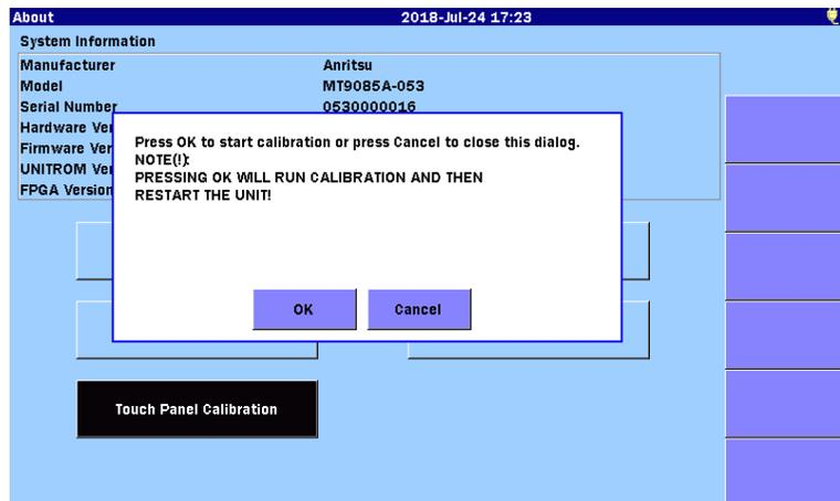
Figure 3.3.4-2 Confirmation Dialog Box for Touch Panel Calibration
