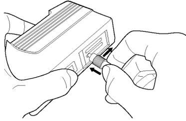
**Figure 16.1-6** Cleaning the Optical Fiber Ferrule End Surface
