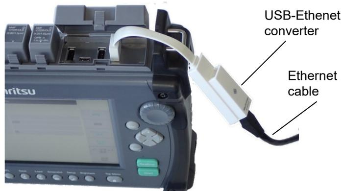
Figure 12.2.1-1 Ethernet Cable Connection
