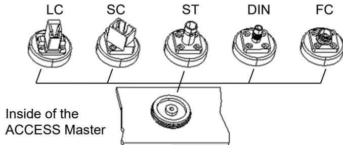
**Figure 2.6.2-2 Connector Types**
