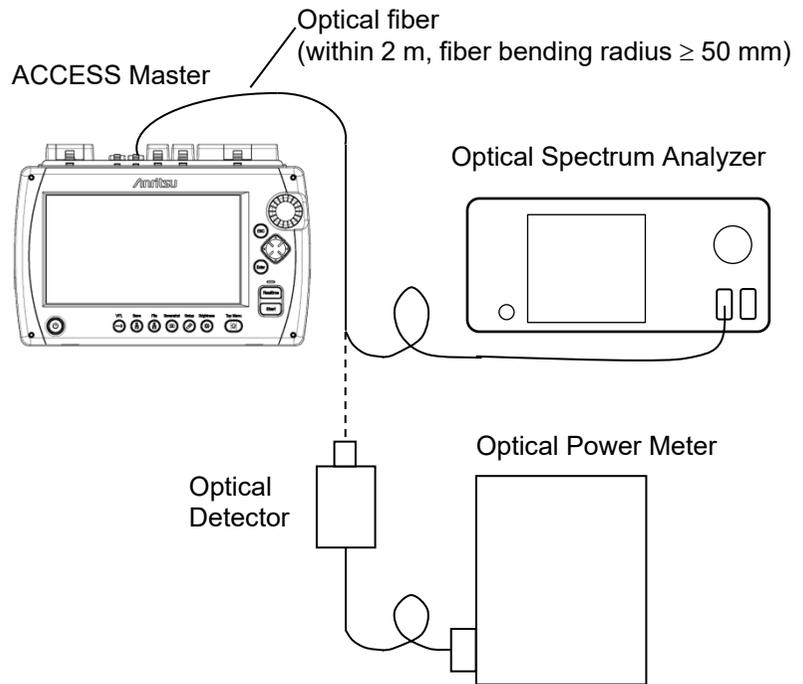
Figure 15.3.7-1 Connection Diagram
