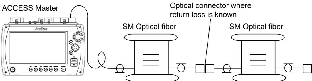
Figure 15.4.1-1 Connection Diagram
