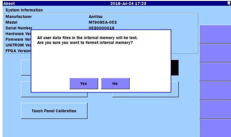
Figure 3.3.4-4 Confirmation Dialog Box for Format Internal Memory
