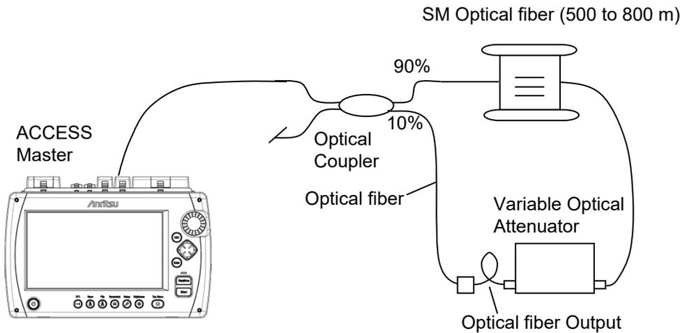
**Figure 15.3.6-1 Connection Diagram**
