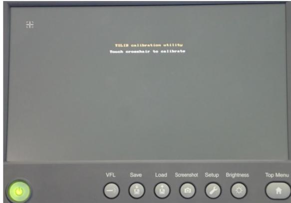
**Figure 3.3.4-3 Touch Panel Calibration Screen**
