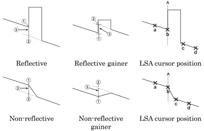
**Figure 8.1.2.2-1 Points to Measure Splice Loss**
