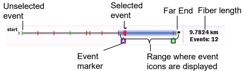
Figure 5.3.1-1 Fiber Schematic
