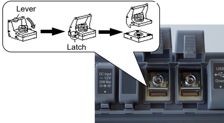
Figure 2.6.1-1 Replaceable Connector
