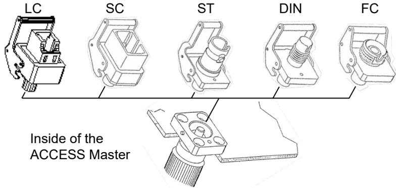
Figure 2.6.1-2 Connector Types
