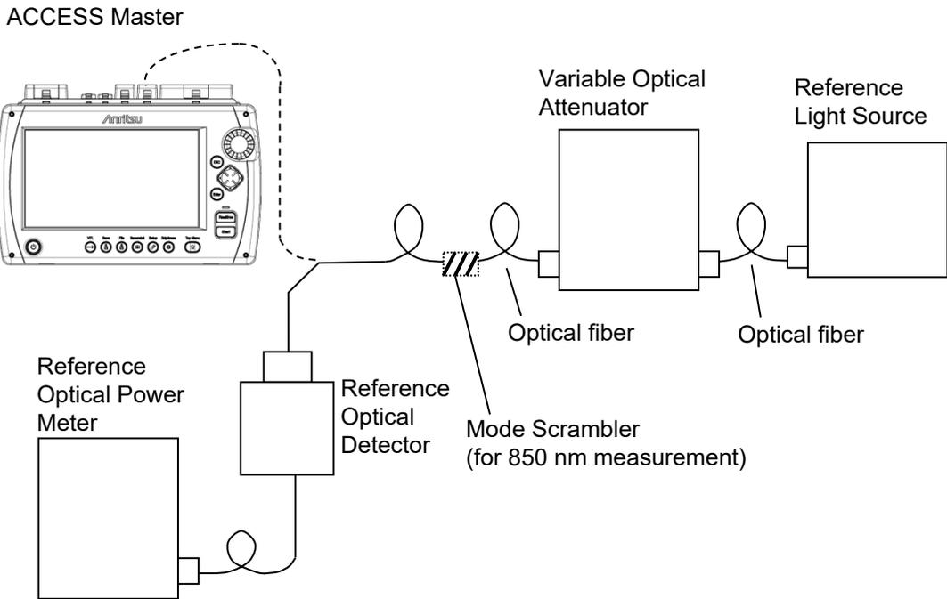
Figure 15.3.9-1 Connection Diagram
