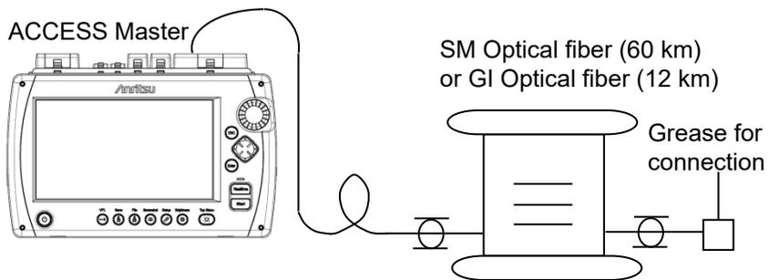
Figure 15.3.5-1 Connection Diagram
