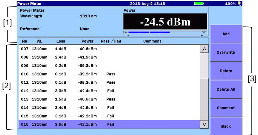
Figure 10.2-1 Loss Table Screen (Power Meter)
