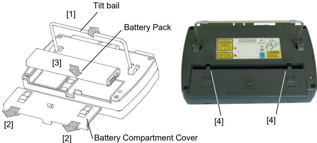
**Figure 2.2.1-1 Installing the Battery Pack**
