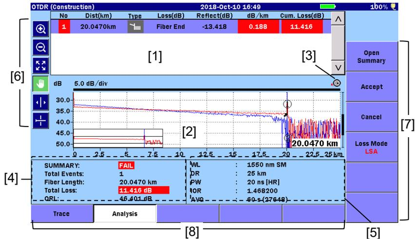
Figure 6.6-1 Test Results screen with Summary Closed
