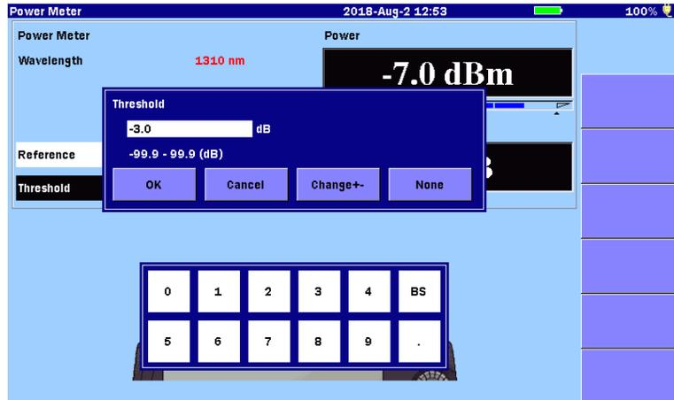
Figure 10.3.3-1 Entering Threshold
