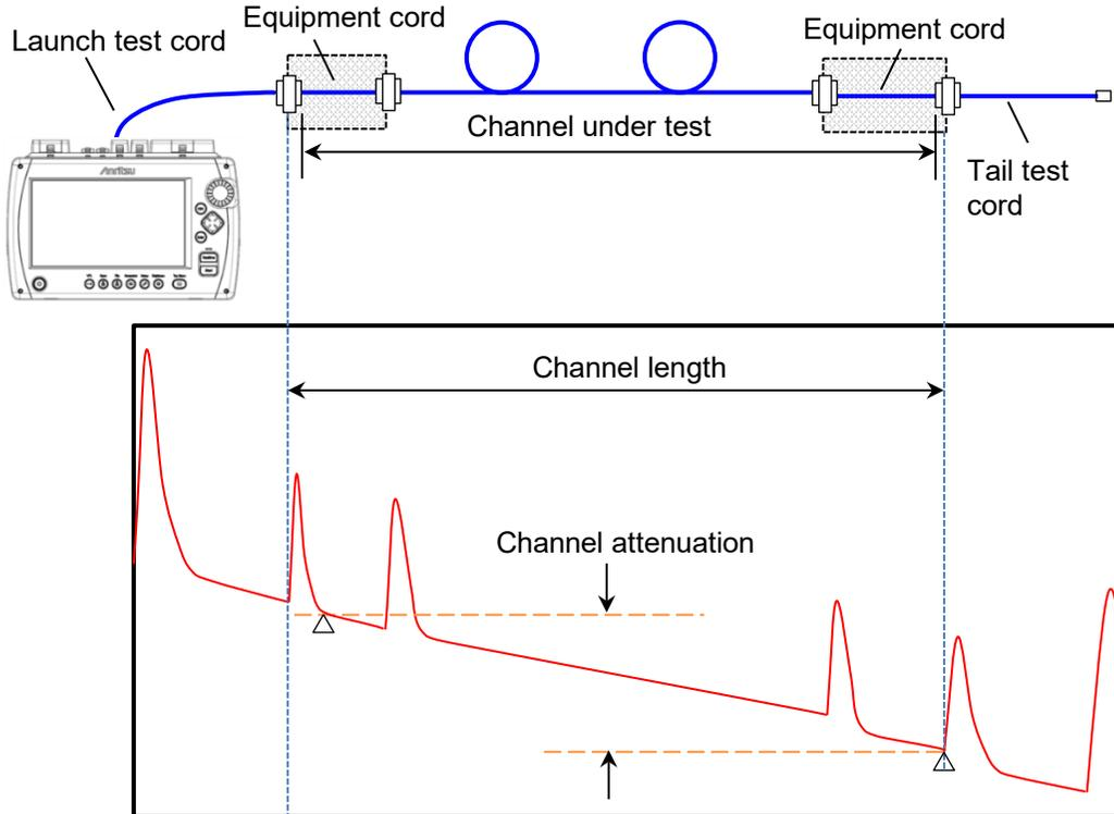
Figure 7.3.2-2 Channel Attenuation
