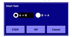
5. For **OTDR**, connect the fiber to the displayed port and touch **Continue** or press Start.
