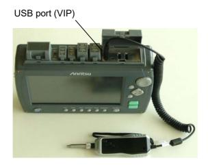
When the VIP is connected to the ACCESS Master, touching **VIP** on Top Menu displays the VIP screen.
