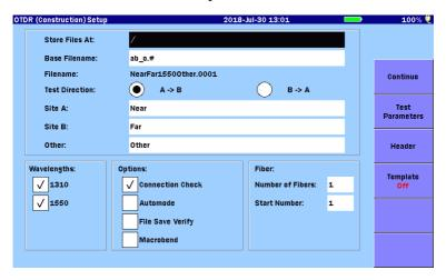
1. Set wavelengths and number of fibers. Select File Save Verify if you confirm filename(s) and a destination folder before saving measurement results.
