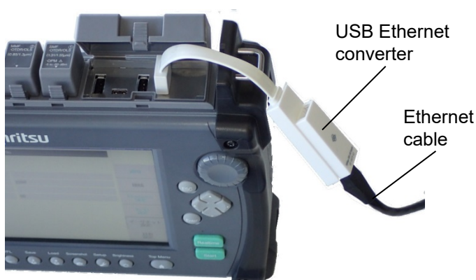
Figure 2.2.1-1 Ethernet Cable Connection
