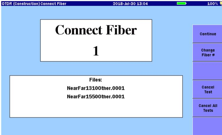
3. Connect the fiber under test to the ACCESS Master and touch **Continue** to start a measurement. To confirm test results when the measurement finishes, touch **Preview** to turn it On.
