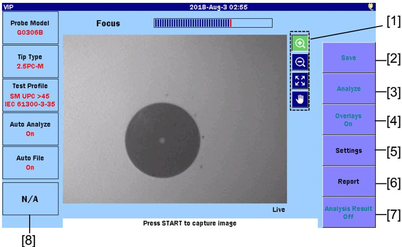
The **Focus** bar indicates the degree of the focus adjustment.
