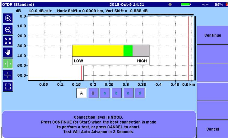
4. If the connection is not good (the gauge is displayed in red or yellow), disconnect the optical fiber from the measurement port and clean its connector.
