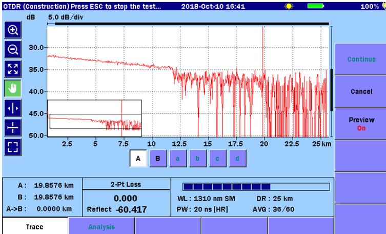
4. When **Preview** is On, after the analysis after measurement is completed, the Summary dialog box is displayed. Touch **Close** to check waveform.
