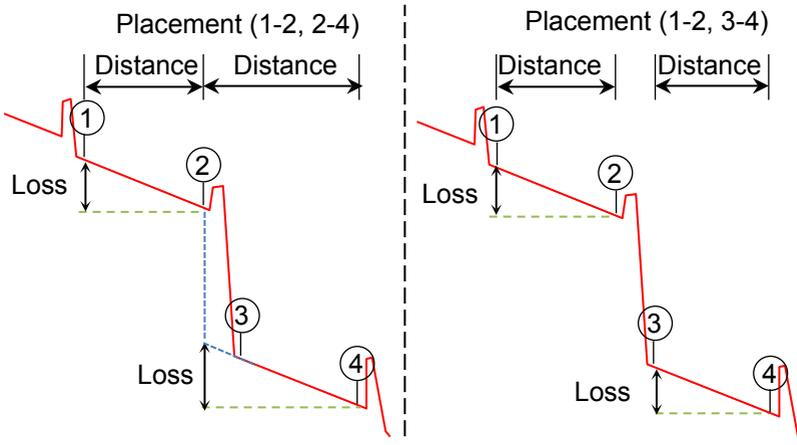
(2PA) The loss is obtained from the level difference between the two markers.
