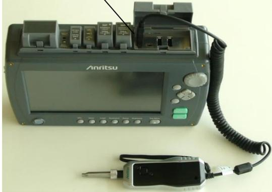
When the VIP is connected to the ACCESS Master, touching **VIP** on Top Menu displays the VIP screen.
