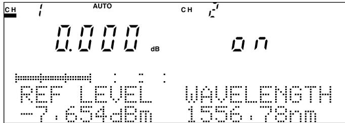
Change the magnitude of attenuation of the optical attenuator in this status. The same value as that of the magnitude of attenuation changed will be indicated.
