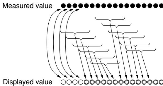
Fig. 4-11 Operations when Averaging Frequency is Set at Five Times
