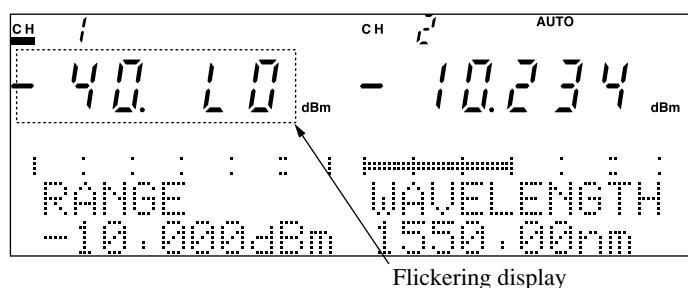
When the minimum range of -90 dBm is set in the AUTO RANGE or MANUAL RANGE mode, if light that falls below -100 dBm is input, the measured value (numerical value) remains displayed and the dBm representation that constitutes the unit flickers to signify the underrange. Moreover, when light that falls below -120 dBm is input, indications of “-130,” the value that is the range display minus 40 dB, and “LO” flicker to signify the underrange.
