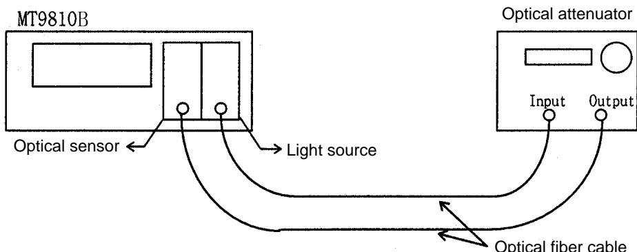
Fig. 4-1 MT9810B Connection Diagram
