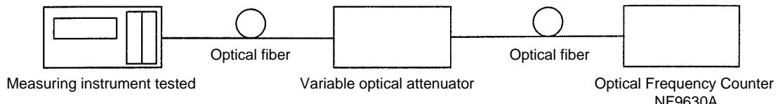
1. Set up a measurement system like that shown in the figure.
