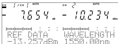
[Display when the mode is in the relative measurement]
