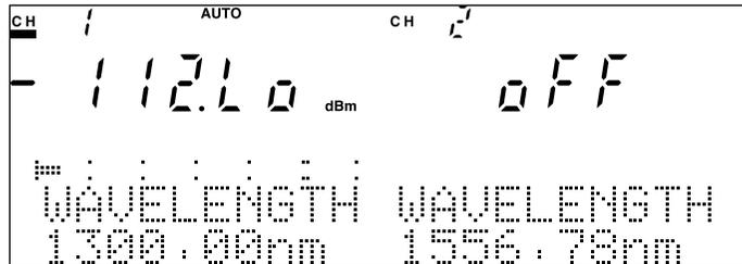
**Fig. 4-2 Display upon Completion of Self-Check**
