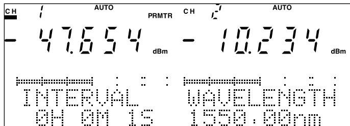
Fig. 4-15 Interval (Optional Value) Setting Screen
