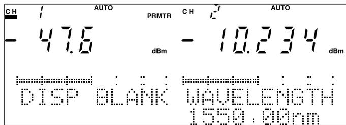
Fig. 4-18 Display Resolution (Blank) Setting Screen
