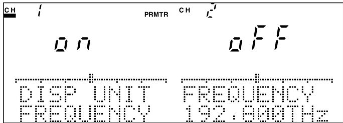
Fig. 4-47 Optical Frequency Display Setting Display
