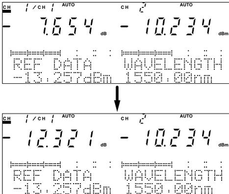
[Display when the mode is in the relative measurement]
