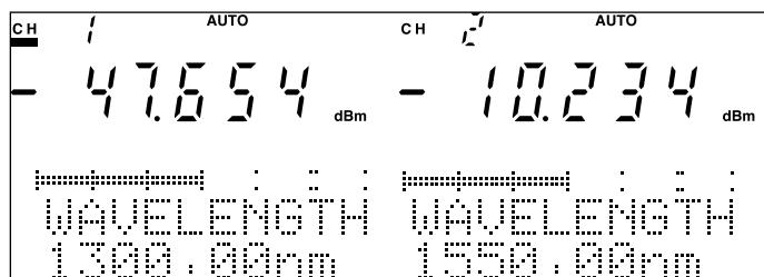
Fig. 4-8 Preset Calibrated Wavelength Setting Screen
