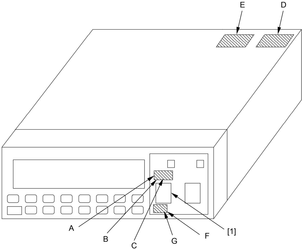
Fig. 1 Locations of Laser Beam Apertures and Affixed Labels
