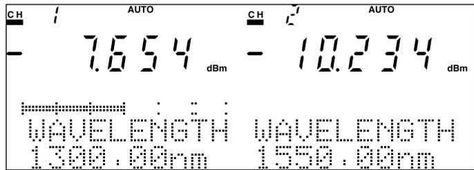
Fig. 4-3 CH1 & CH2 Setting Screen
