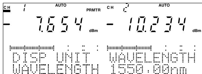
Fig. 4-16 Wavelength Display Setting Screen
