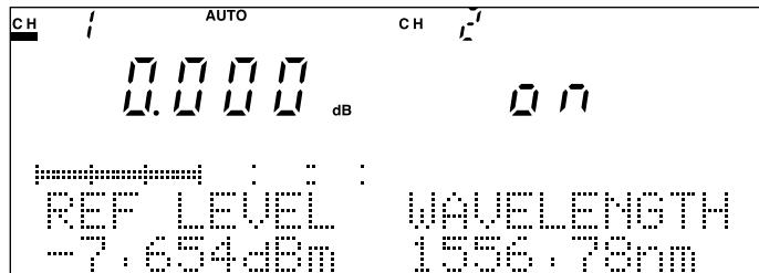
Change the magnitude of attenuation of the optical attenuator in this status. The same value as that of the magnitude of attenuation changed will be indicated.
