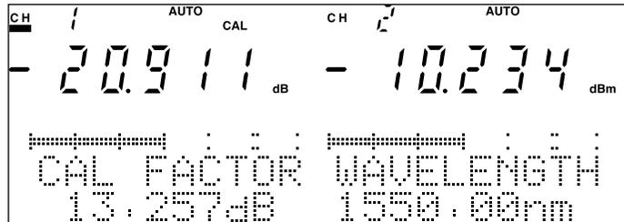
Fig. 4-25 Calibration Measurement Screen
