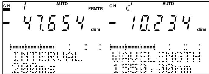
Fig. 4-14 Interval (Fixed Value) Setting Screen
