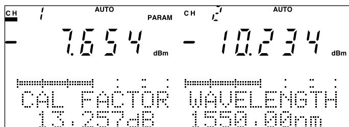
Fig. 4-24 Correction Value (CAL FACTOR) Setting Screen
