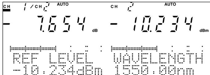
Fig. 4-23 Reference Measurement Screen
