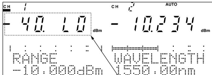
When the minimum range of -90 dBm is set in the AUTO RANGE or MANUAL RANGE mode, if light that falls below -100 dBm is input, the measured value (numerical value) remains displayed and the dBm representation that constitutes the unit flickers to signify the underrange. Moreover, when light that falls below -120 dBm is input, indications of “-130,” the value that is the range display minus 40 dB, and “LO” flicker to signify the underrange.
