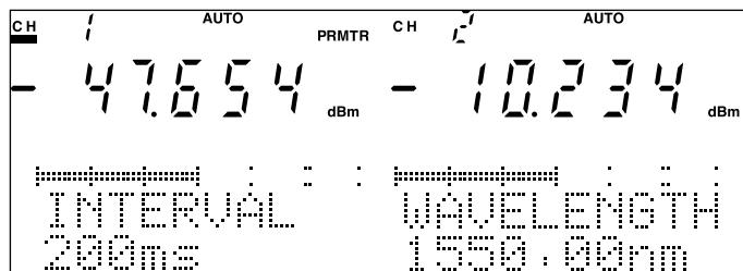
Fig. 4-14 Interval (Fixed Value) Setting Screen
