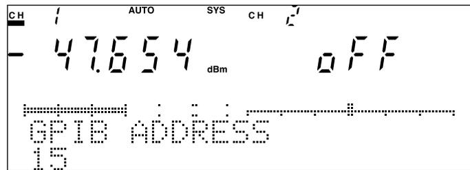
Fig. 4-50 GPIB Address Setting Screen
