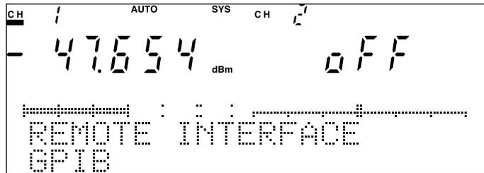
Fig. 4-49 Remote Interface Setting Screen
