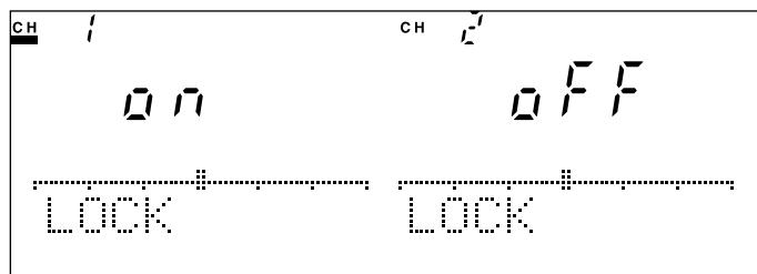
Message Display when Optical Output Modifier Key Switch is OFF
