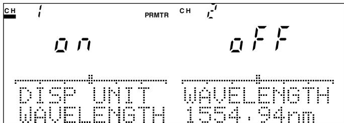
Fig. 4-48 Wavelength Display Setting Screen
