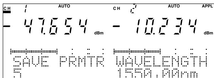
Fig. 4-28 Measurement Condition Recording Screen
