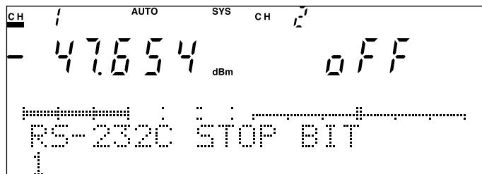
Fig. 4-52 RS-232C Stop Bit Setting Screen
