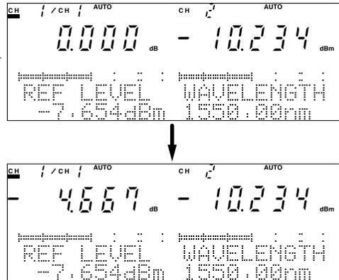
Fig. 4-20 Shift from Reference Measurement to Relative Measurement
