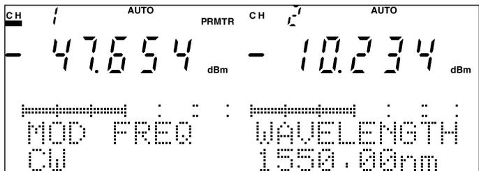
Fig. 4-13 Modulated Radiation Measurement OFF Setting Screen
