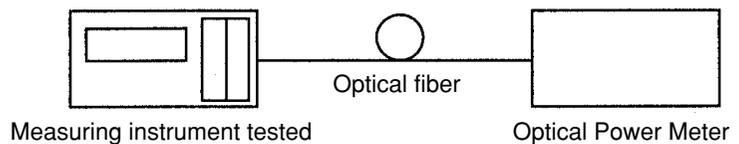
1. Set up a measurement system like that shown in the figure.
