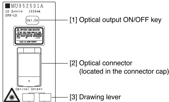
[1] Optical output ON/OFF key
