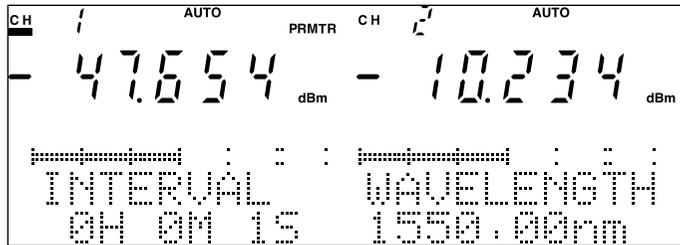
Fig. 4-15 Interval (Optional Value) Setting Screen
