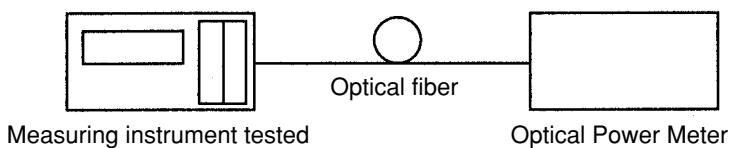
1. Set up a measurement system like that shown in the figure.
