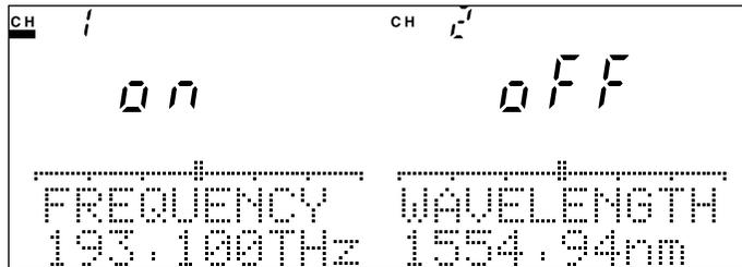
Fig. 4-40 Center Optical Frequency Representation Screen
