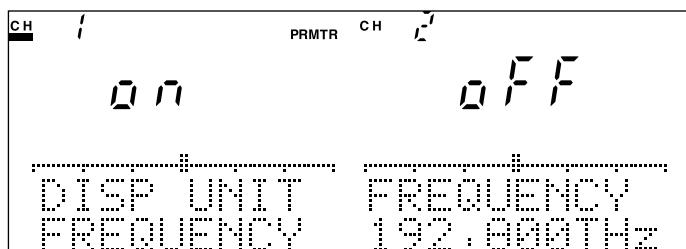
Fig. 4-47 Optical Frequency Display Setting Display
