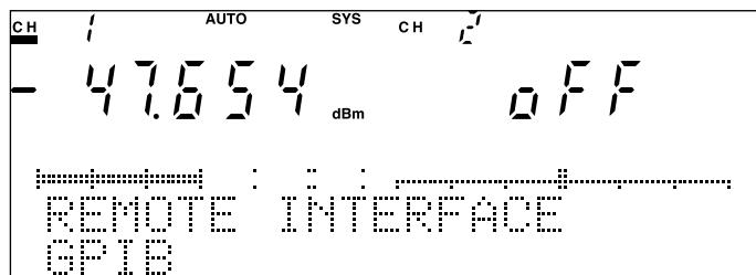
Fig. 4-49 Remote Interface Setting Screen
