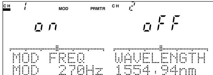
Fig. 4-41 Modulation Mode ON Screen
