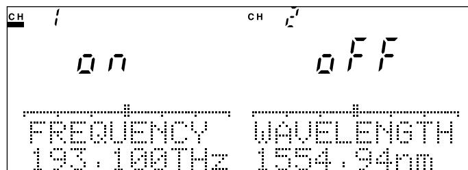
Fig. 4-40 Center Optical Frequency Representation Screen
