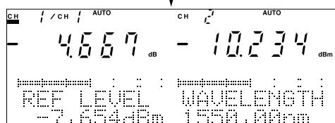
**Fig. 4-20 Shift from Reference Measurement to Relative Measurement**
