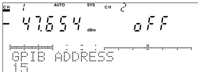
Fig. 4-50 GPIB Address Setting Screen
