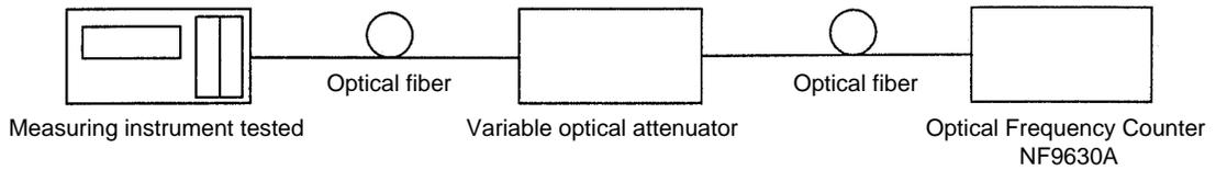
1. Set up a measurement system like that shown in the figure.
