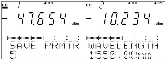
Fig. 4-28 Measurement Condition Recording Screen
