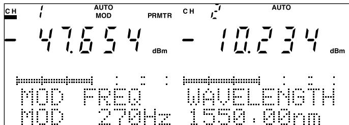
Fig. 4-12 Modulated Radiation Measurement ON Setting Screen
