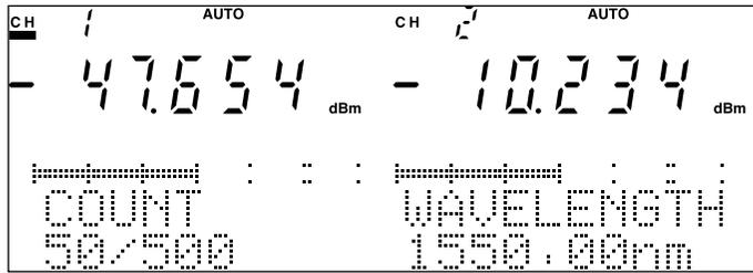
**Fig. 4-32 Screen to Set Number of Data to be Recorded (When the Interval is 500 ms or Greater)**
