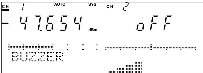
Fig. 4-56 Screen to Set Sound Volume of Buzzer
