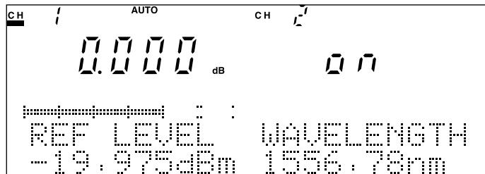
The display immediately before the Rel key is pressed shows a value 12.321 dB lower than the reference value of -7.654 dBm. Therefore, it means that a measured value of -19.975 dBm was obtained in that state. If the Rel key is pressed, the relative measurement is performed by using -19.975 dBm as a new reference value.
