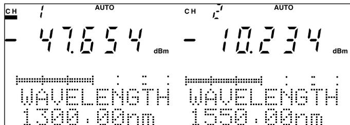
Fig. 4-8 Preset Calibrated Wavelength Setting Screen
