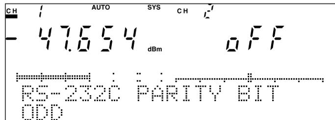
Fig. 4-53 RS-232C Parity Bit Setting Screen
