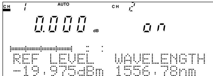
The display immediately before the Rel key is pressed shows a value 12.321 dB lower than the reference value of -7.654 dBm. Therefore, it means that a measured value of -19.975 dBm was obtained in that state. If the Rel key is pressed, the relative measurement is performed by using -19.975 dBm as a new reference value.
