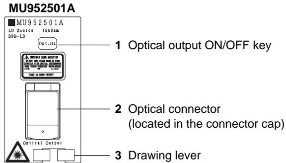
1 Optical output ON/OFF key Used to switch the optical output ON and OFF.
