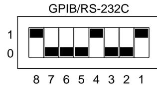
Fig. 5-2 GPIB Address 01001 Setting Example
