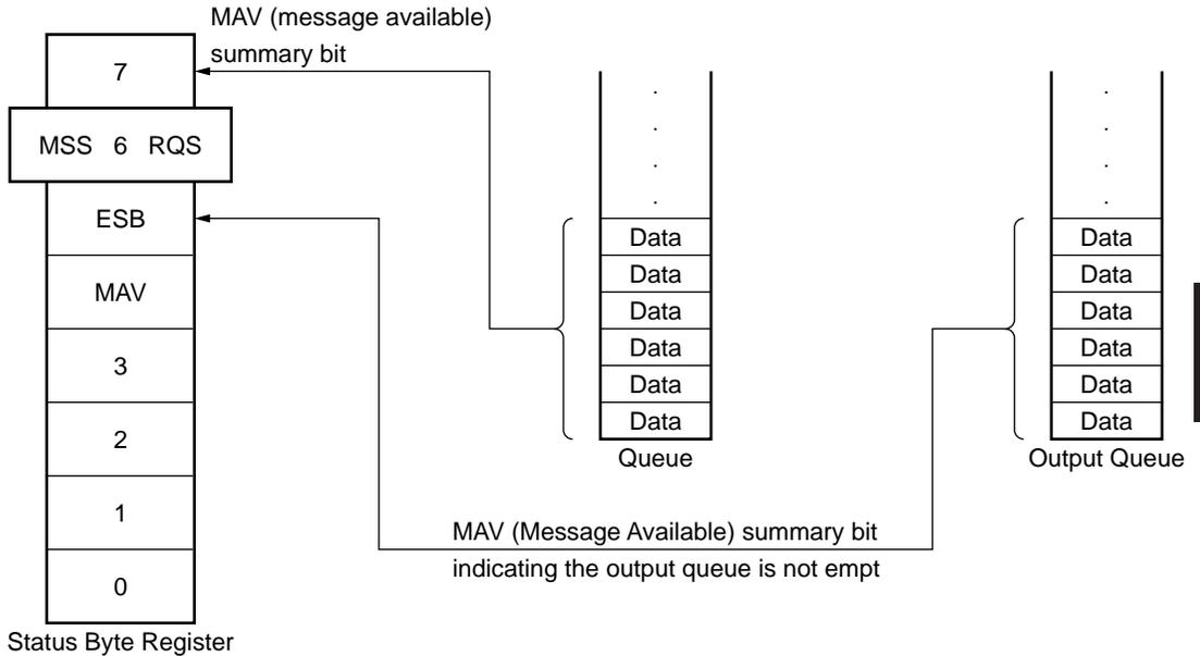
The queue that outputs an MAV summary bit to status byte register bit 4 is called an "output queue." This queue is mandatory. The queue that can output an MAV summary message to one of status byte register bits 0 to 3 and 7 is simply called a "queue." It is optional. A summary message from the register model can also be output to status byte register bits 0 to 3 and 7, so the summary message type depends on the device type.
