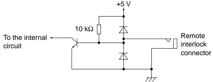
Unless the following three conditions are met, no optical output will be made from the light source.
