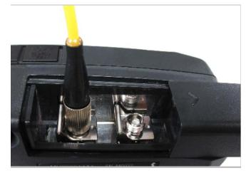
Figure 2.6-1 Connecting Fiber to Measurement Port
