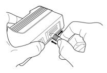
Figure 2.7-6 Cleaning of ferrule end surface of optical fiber - 2
