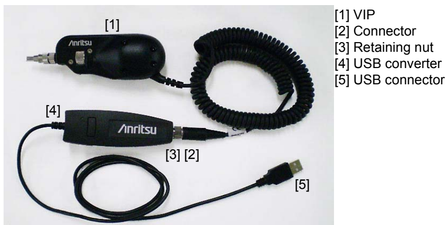
Figure 9.2-3 VIP Connected to USB Converter
