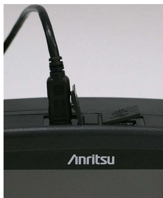
Figure 2.10.2-1 USB Cable Connection
