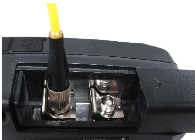
Figure 2.6-1 Connecting Fiber to Measurement Port
