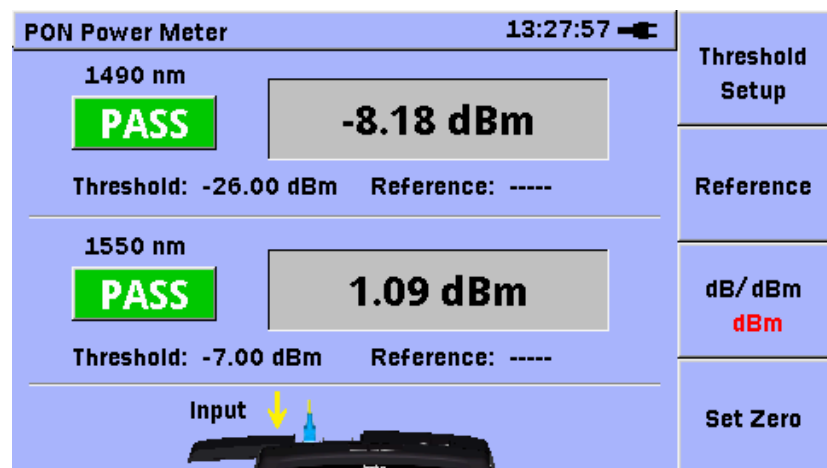
Figure 1.1.5-1 PON Power Meter Screen
