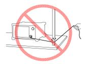
Doing so may break the optical fiber inside the cable. Keep the bend radius of an optical fiber cable at 30 mm or more. If the radius is less, optical fiber cable loss will increase.
