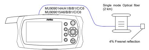
Figure 11.1.5-1 Distance Measurement Accuracy Test - Connection Diagram
