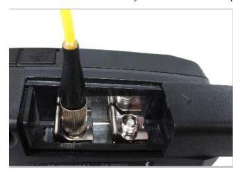
Figure 2.6-1 Connecting Fiber to Measurement Port
