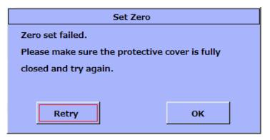
When the set zero is re-executed, confirm the slide cover is firmly closed, and then select **Retry**. Press to start the set zero.
