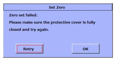
When the set zero is re-executed, confirm the slide cover is firmly closed, and then select **Retry**. Pressing set executes the set zero.
