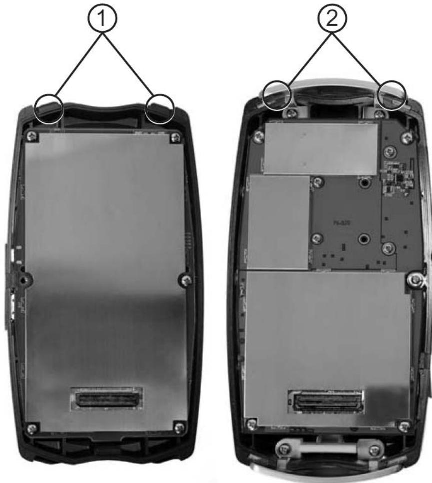
**Figure 1.6-1 Alignment Tabs and Slots**
