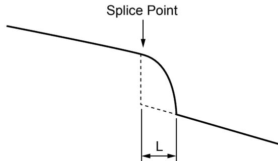
Therefore, the splice loss cannot be measured correctly in the Loss mode. In the Splice & Return Loss mode, two markers are set on each side of the splice point. The splice loss is calculated as shown below.
