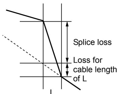
In this measurement, the distance between the x1 and x2 markers and that between the x3 and x4 markers, as well as the fiber loss (loss per unit length) are also displayed.
