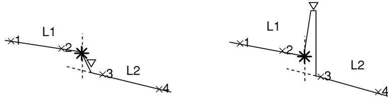
There are two methods for determining these lines: the LSA and 2PA methods. Of these methods, this section explains the LSA (Least Square Approximation) method.
