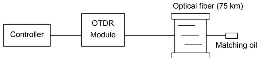
(b) When MW9077A-01 (Opt 01, 1550 nm filter) is installed and measuring pulse width is 20  $\mu$ s.
