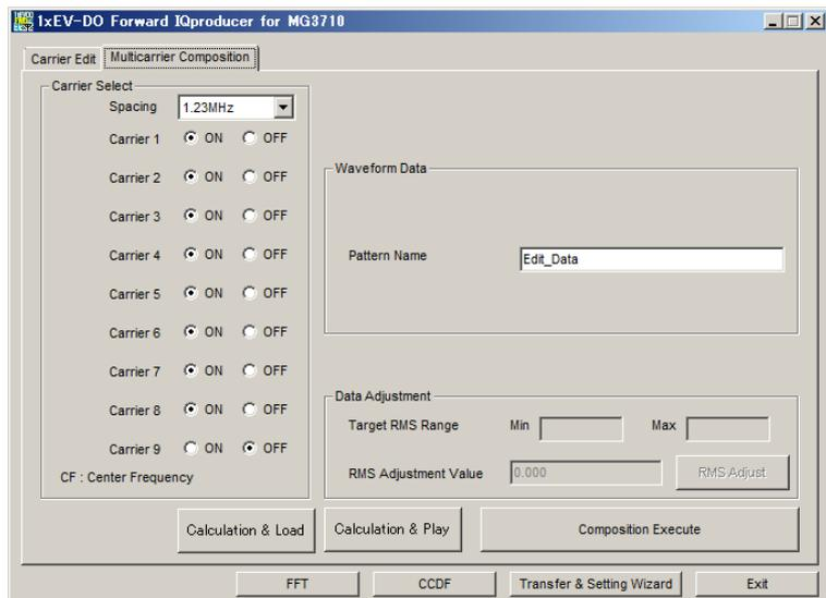
Figure 3.1.1.3-2 Multicarrier Composition sheet (When running on MG3710A)
