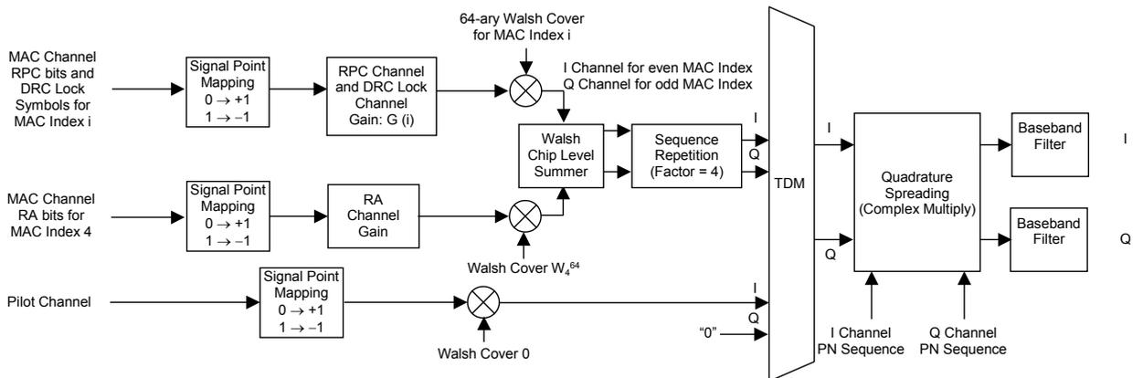
**Figure 3.1.5.1-5 Block diagram of 1xEV-DO forward idle slot**
