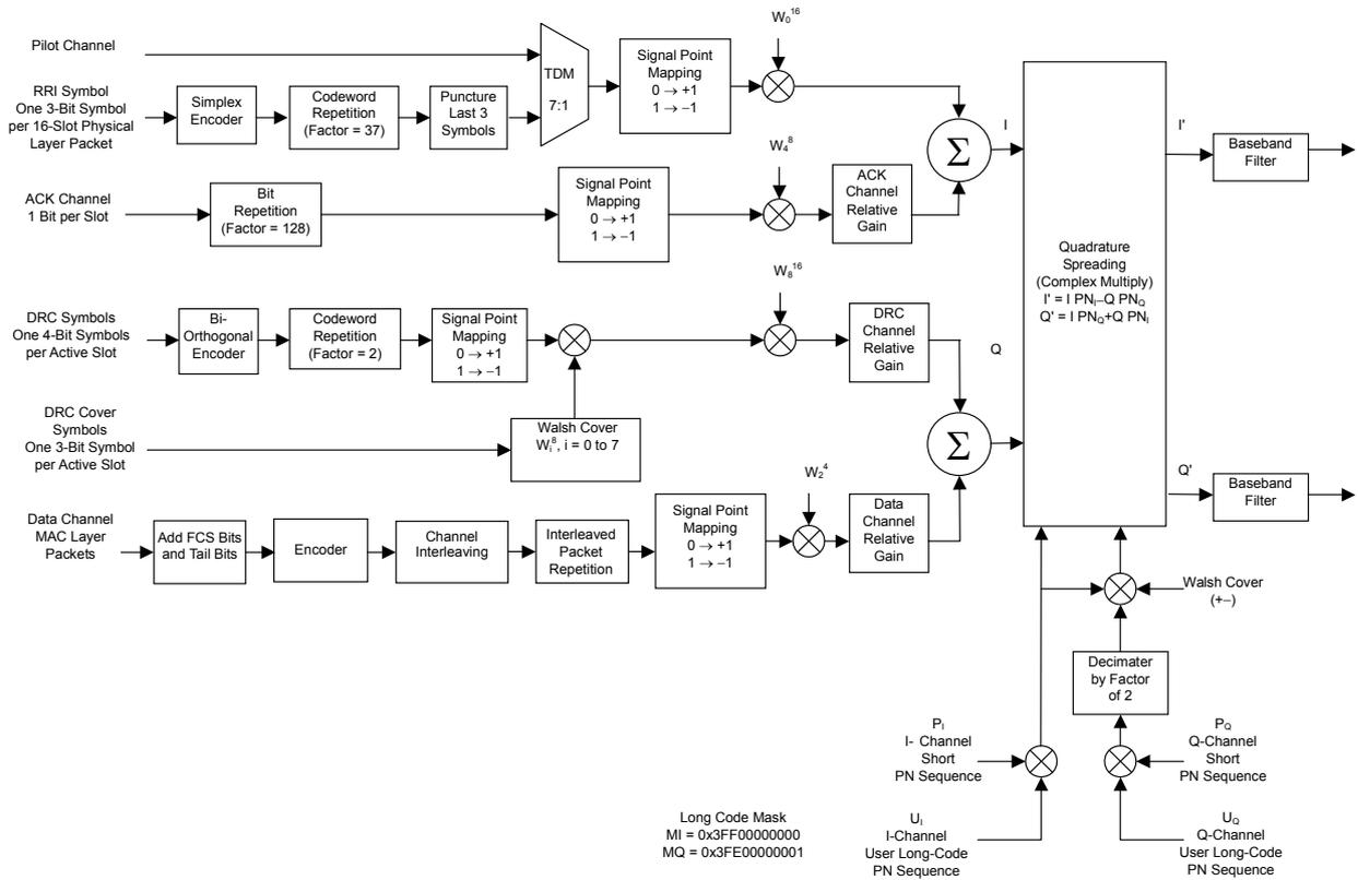
Figure 3.2.5.1-2 Block diagram of 1xEV-DO Reverse
