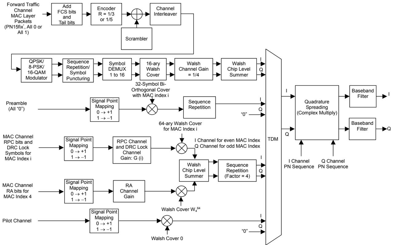
Figure 3.1.5.1-2 Block diagram of 1xEV-DO forward active slot
