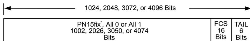
Figure 3.1.5.1-1 Forward packet format before coding
