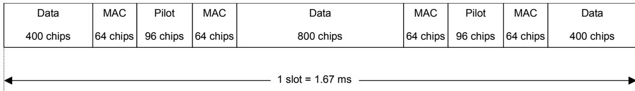
Figure 3.1.5.1-4 1xEV-DO forward active slot format after TDM
