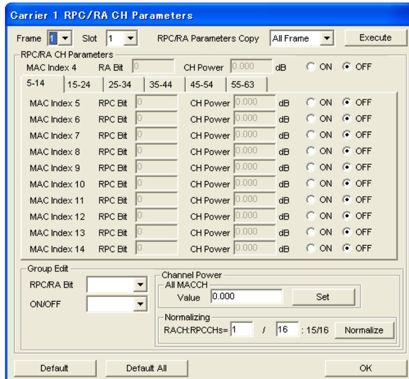
Figure 3.1.1.2-1 RPC/RA CH Parameters screen
