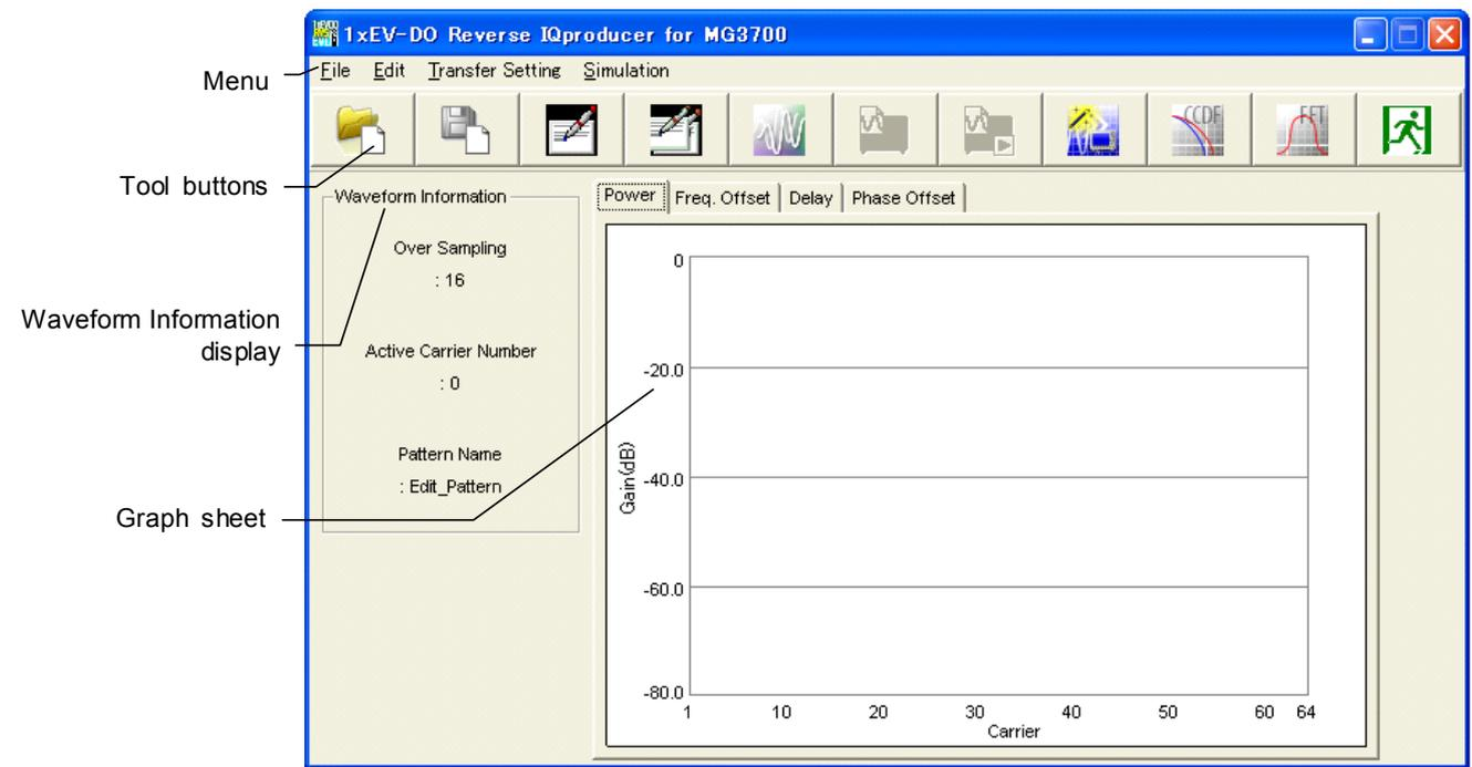
Figure 3.2.1.1-1 1xEV-DO Reverse IQproducer main screen
