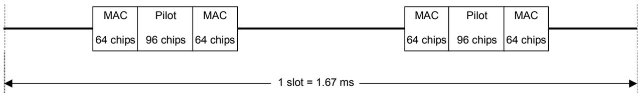
**Figure 3.1.5.1-6 1xEV-DO forward idle slot format after TDM**
