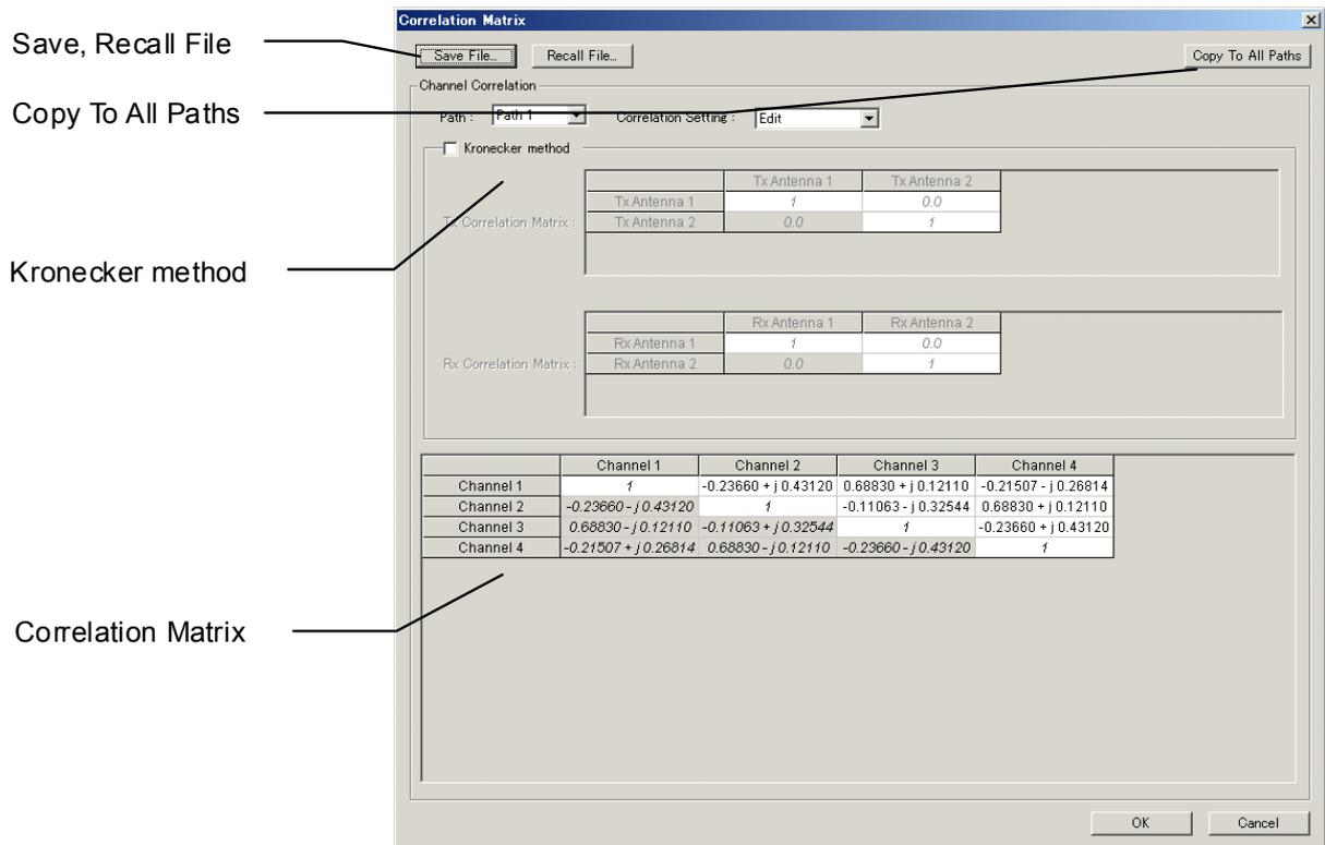
Figure 3.1.3-4 Correlation Matrix setting window (2 × 2 MIMO configuration)
