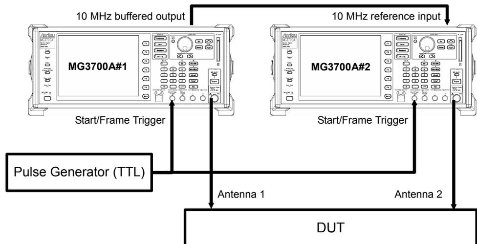
Figure C.1-1 Multiple MG3700A connection (external Start/Frame Trigger)
