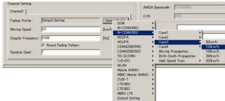
Figure 3.3.1-4 Selecting fading profile
