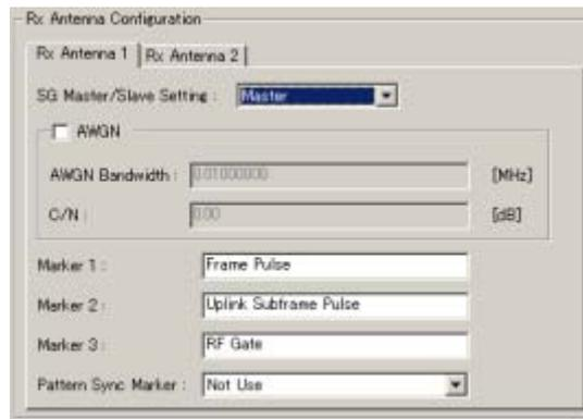
Figure 3.3.5-7 Settings on Rx Antenna1 tab window
