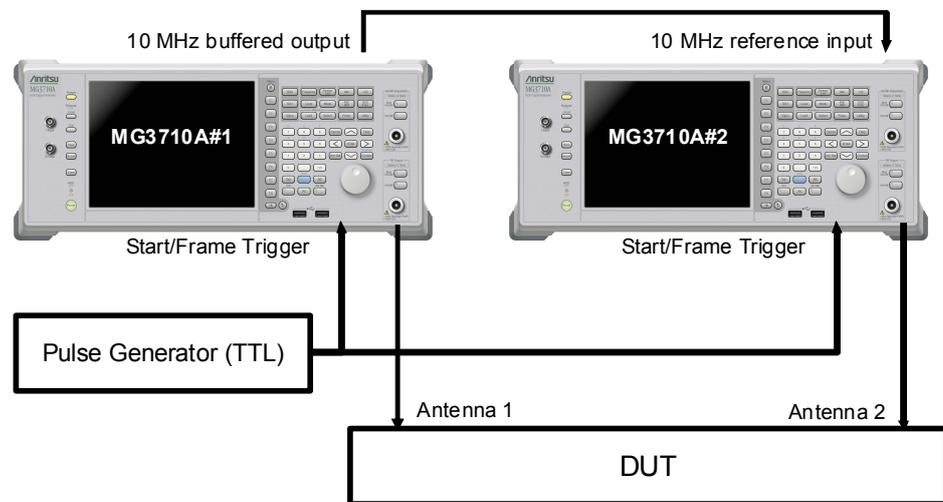
Figure C.2-1 Multiple MG3710A connection (external Start/Frame Trigger)
