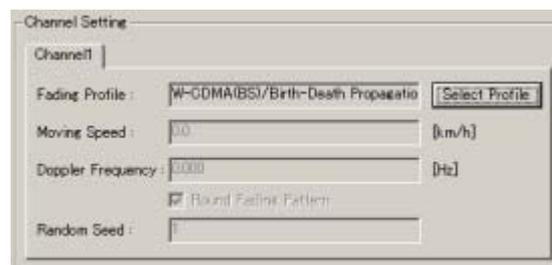
Figure 3.3.3-5 Settings in Channel Setting field (Birth-Death Propagation)
