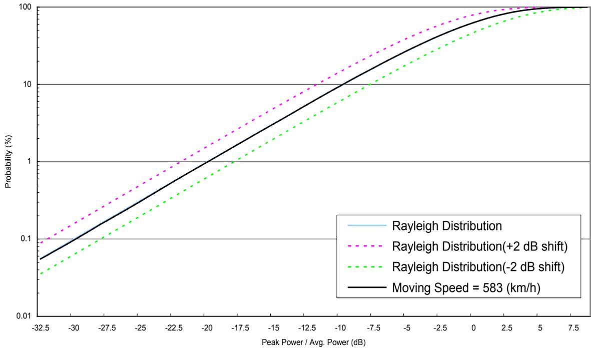
**Figure D.2-9 Accumulated probability distribution (Moving Speed = 583 km/h)**
