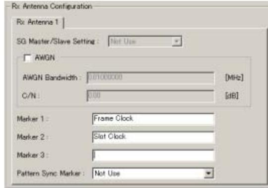
Figure 3.3.3-6 Settings in Rx Antenna Configuration field
