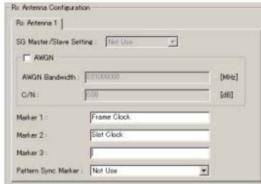
Figure 3.3.2-6 Settings in Rx Antenna Configuration field
