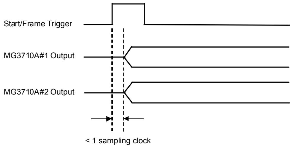
**Figure C.2-2 Synchronization-baseband signals when using external Start/Frame Trigger**
