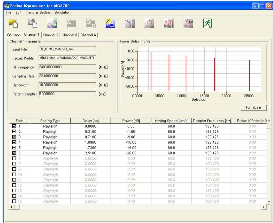
Figure 3.3.5-9 Channel parameter setting screen (2 × 2 MIMO)
