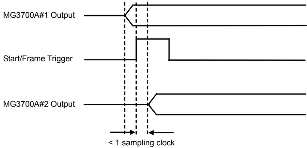
Figure C.1-5 Synchronization relationship of baseband signals when using Master/Slave
