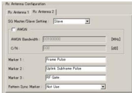
Figure 3.3.5-8 Settings on Rx Antenna2 tab window
