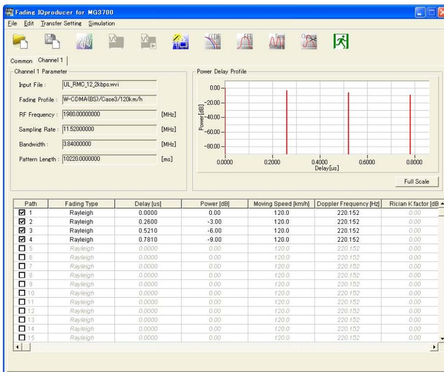
Figure 3.3.1-7 Channel parameter setting screen (1 × 1 SISO)
