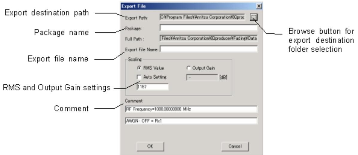
Figure 3.1.7-1 Export File window (when generating one waveform pattern)
