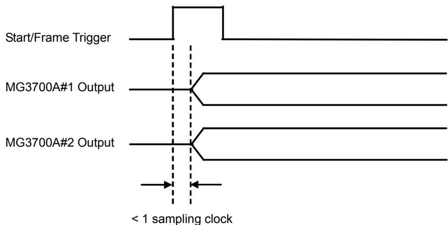
**Figure C.1-2 Synchronization-baseband signals when using external Start/Frame Trigger**
