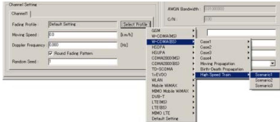
Figure 3.3.4-4 Selecting fading profile
