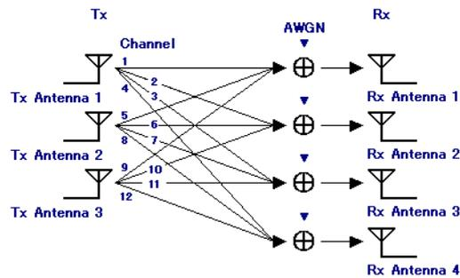
Figure 3.1.2.2-12  $3 \times 4$  MIMO configuration
