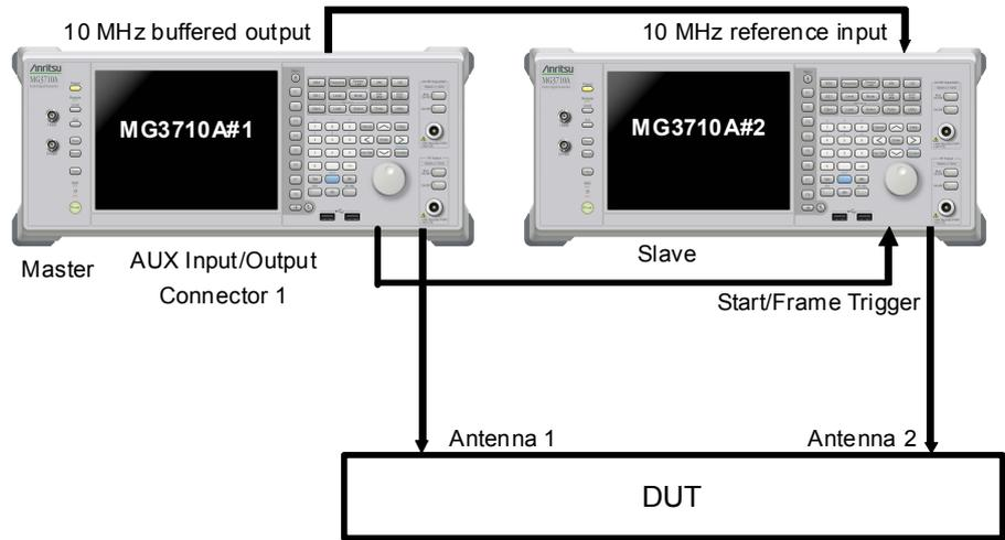
Figure C.2-4 Multiple MG3710A connection (Master/Slave)
