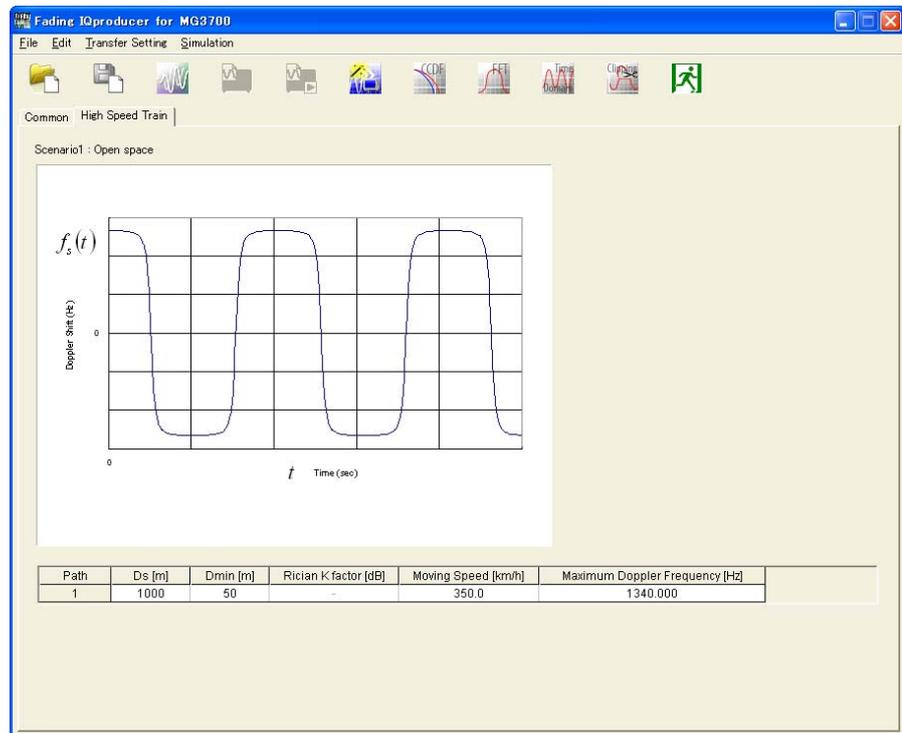
Figure 3.1.6-1 High Speed Train tab window (Scenario1)
