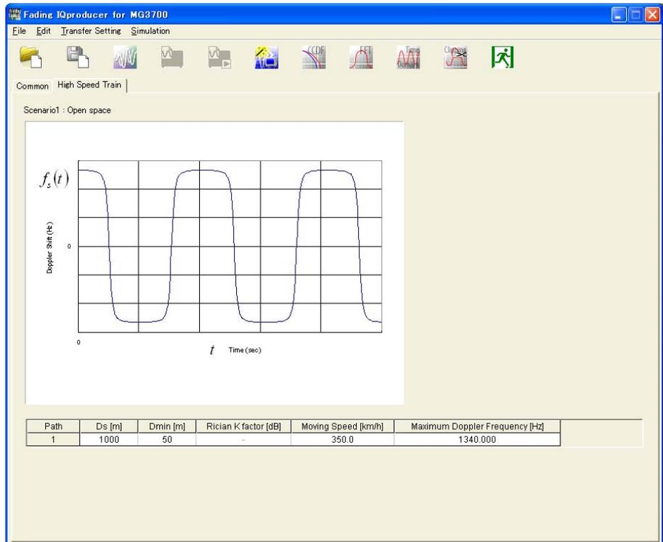
Figure 3.3.4-7 High Speed Train tab window (Scenario1)
