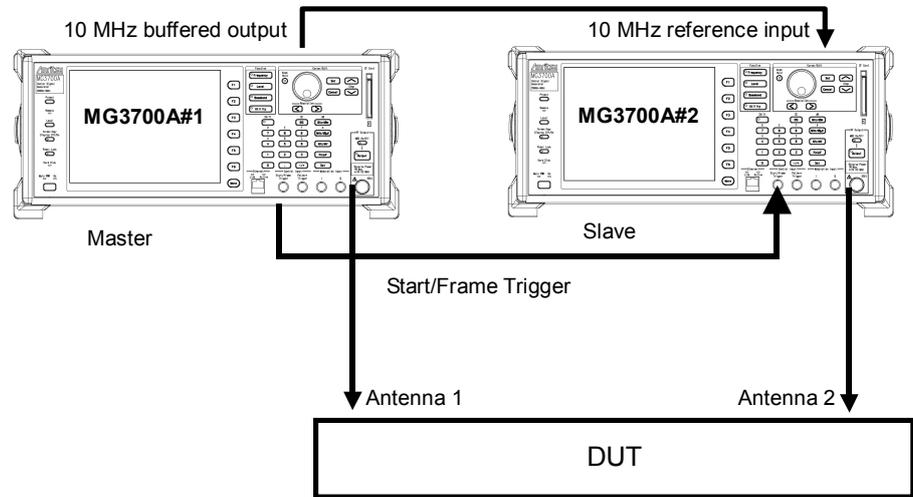
Figure C.1-4 Multiple MG3700A connection (Master/Slave)
