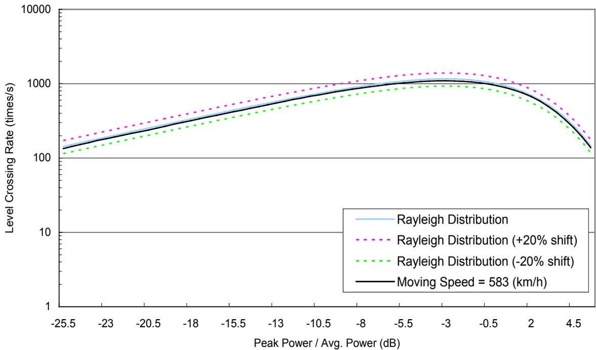
**Figure D.2-10 Level crossing rate (Moving Speed = 583 km/h)**
