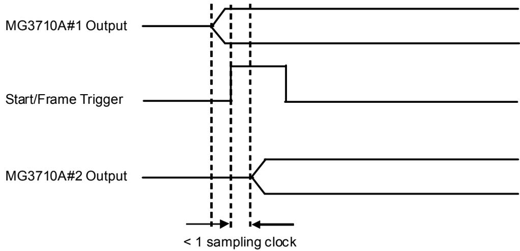
Figure C.2-5 Synchronization relationship of baseband signals when using Master/Slave
