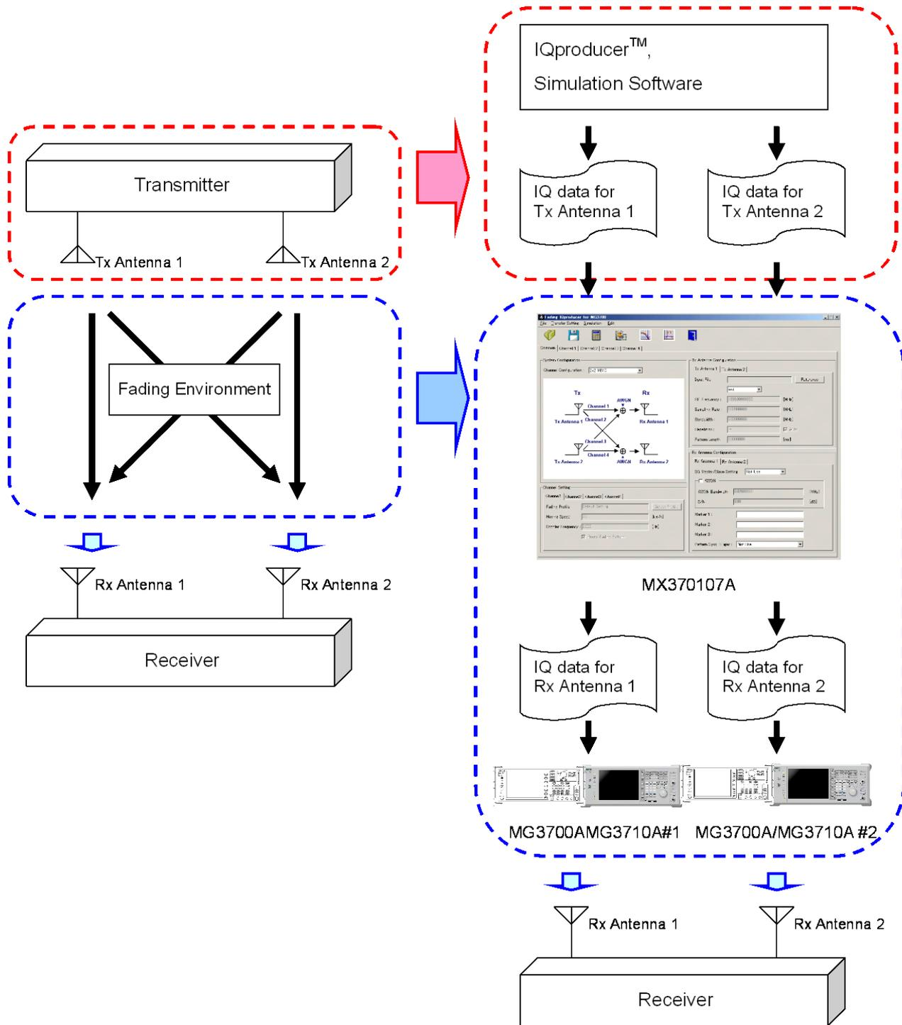
Fig. 1.1-2 2 x 2 MIMO configuration example
