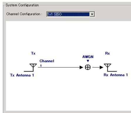
Figure 3.3.1-1 System Configuration (1 × 1 SISO)
