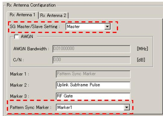
Figure C.2-3 Setting example of Master side
