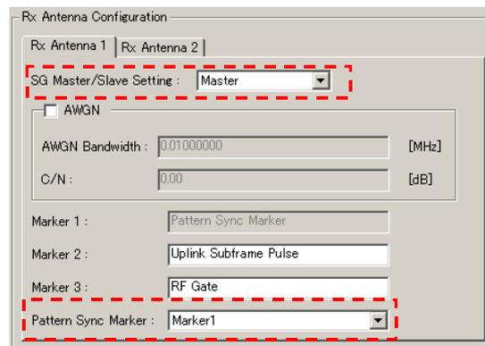
Figure C.1-3 Setting example of Master side
