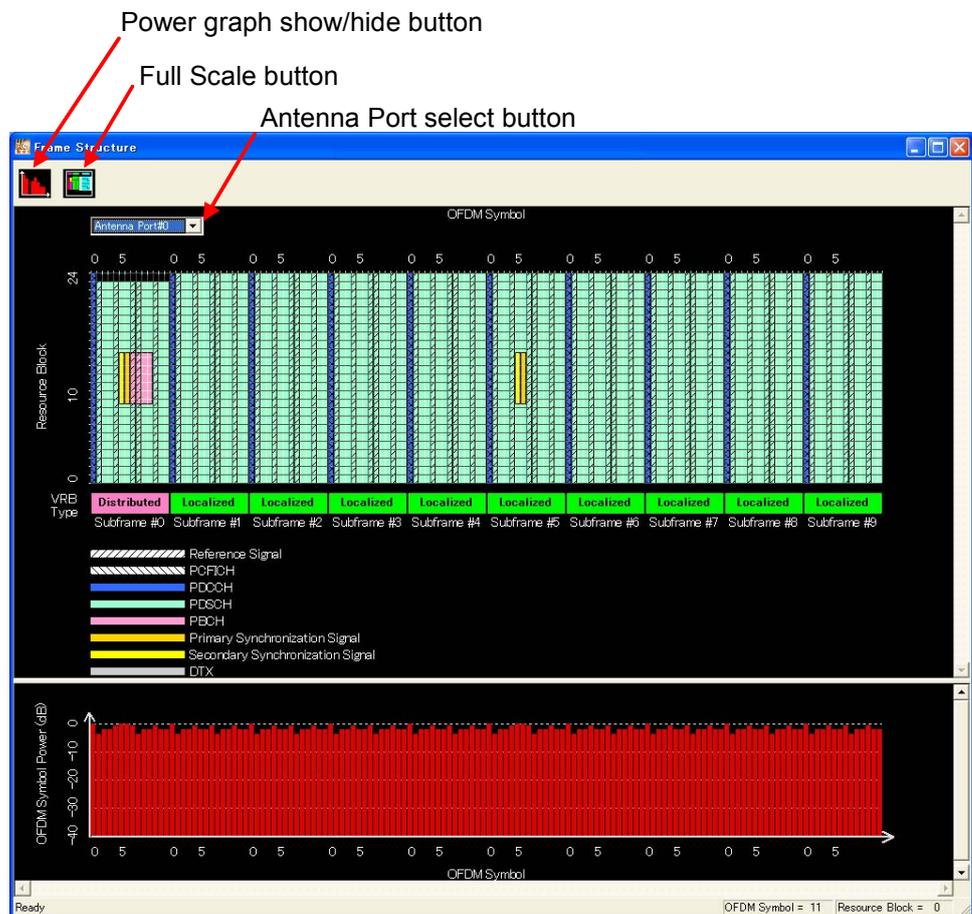
Figure 3.1.7-1 Frame Structure Screen and Power Graph
