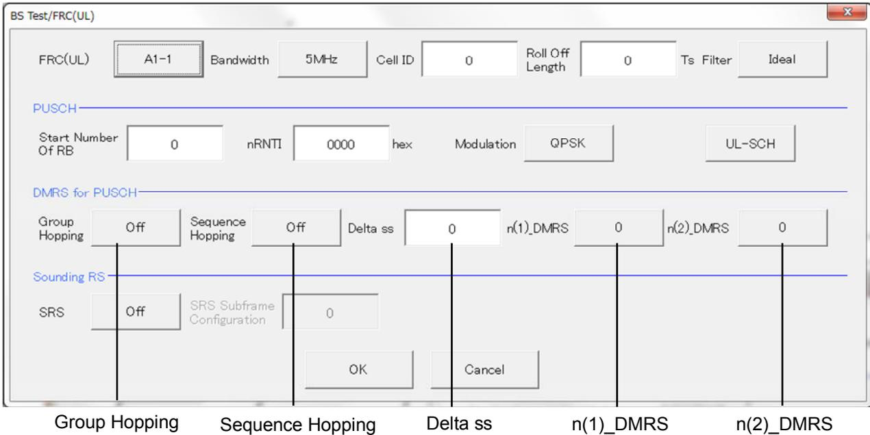
Figure 4.4.3.3-1 DMRS for PUSCH Parameters Setting Screen
