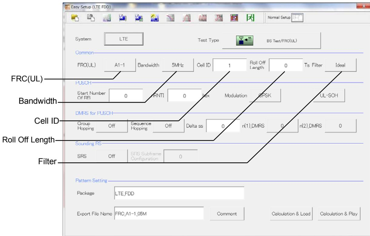
Figure 4.3.3.1-1 BS Test/FRC (UL) Common Parameter Setting Section
