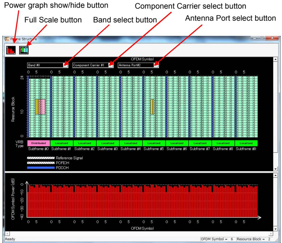
Figure 3.1.7-2 Frame Structure Screen and Power Graph (LTE-Advanced)
