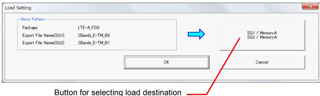
Figure 4.4.6-2 Load Setting Screen (Carrier Aggregation Mode = Inter-band)
