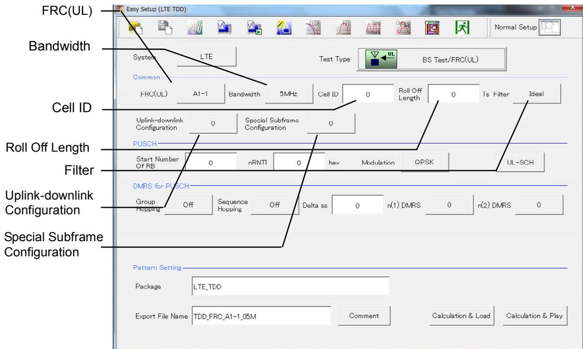
Figure 4.3.3.1-1 BS Test/FRC (UL) Common Setting Screen
