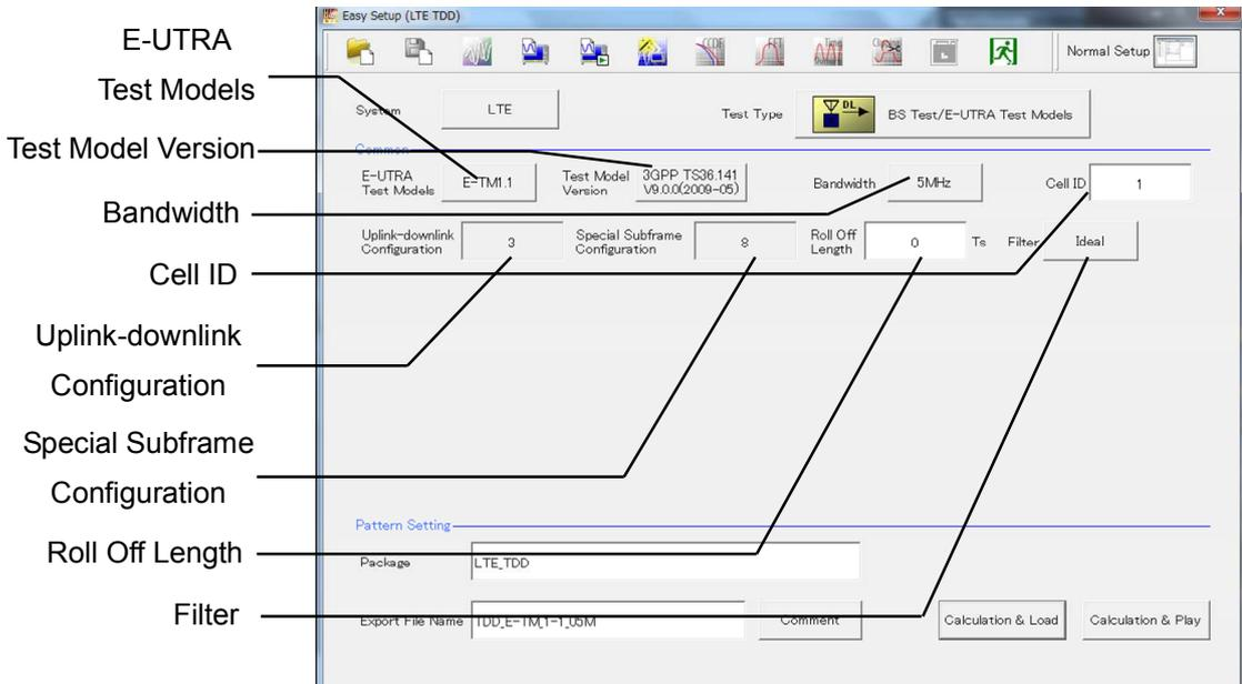
Figure 4.3.2.1-1 BS Test/E-UTRA Test Models Common Setting Screen
