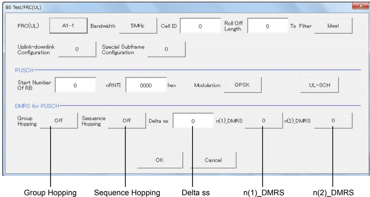
Figure 4.4.3.3-1 DMRS for PUSCH Parameters Setting Screen
