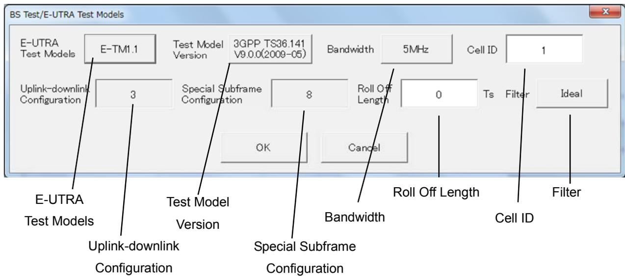
Figure 4.4.2-1 BS Test/E-UTRA Test Models Setting Screen
