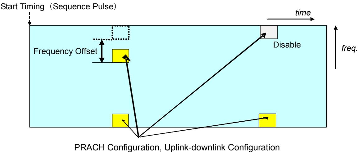
Figure 3.2-1 Parameters for PRACH in 1 Frame
