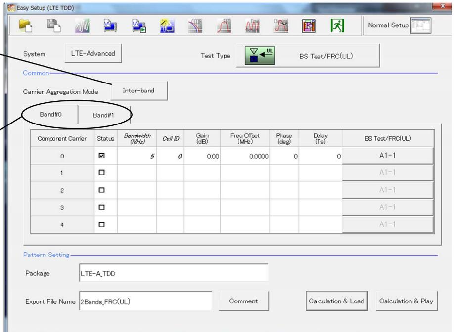
Carrier Aggregation Mode=Inter-band setting screen
