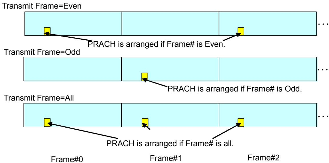
Figure 3.2-2 PRACH Frame Arrangement by Transmit Frame
