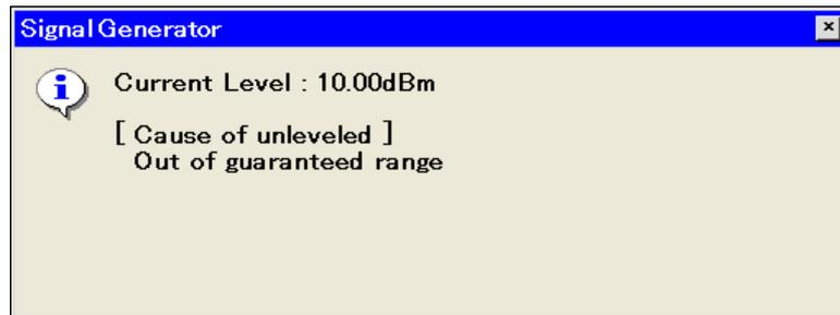
Figure 2.3.12-1 Output level display window
