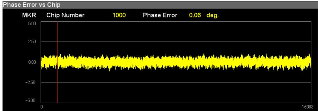
Figure 3.14-1 Phase Error vs Chip Display
