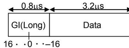
Figure 3.6-1 FFT Window Start Position When Guard Interval = Long
