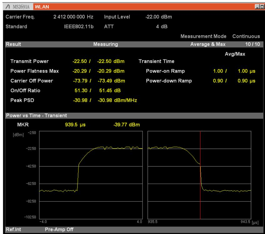
Figure 3.18-1 Power vs Time Setting Screen (Transient)
