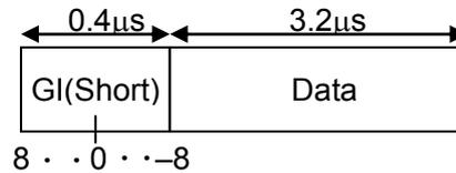
Figure 3.6-2 FFT Window Start Position When Guard Interval = Short
