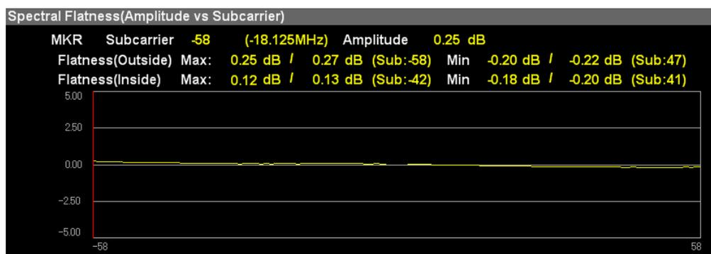
Figure 3.15-1 Amplitude of Spectral Flatness Display
