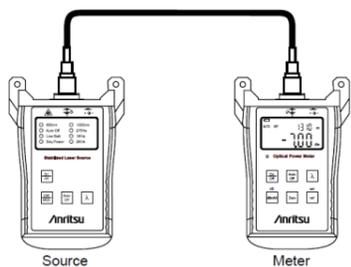
**Figure 3 Checking Output Power**
