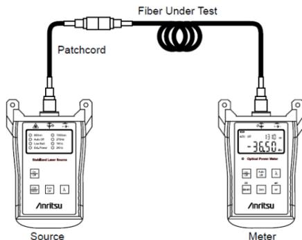
**Figure 4 Optical Loss Measurement Setup**
