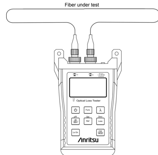
Figure 4 Connection when optical loop loss testing
