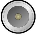
RF output connector (when Option 020 installed)
