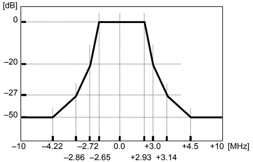
Figure 2.5.1-3 Transmission Spectrum Mask (Equipment Standard: Type A)
