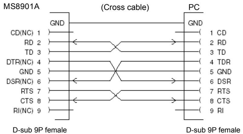
Figure 3.1.2-2 RS-232C cross cable connection
