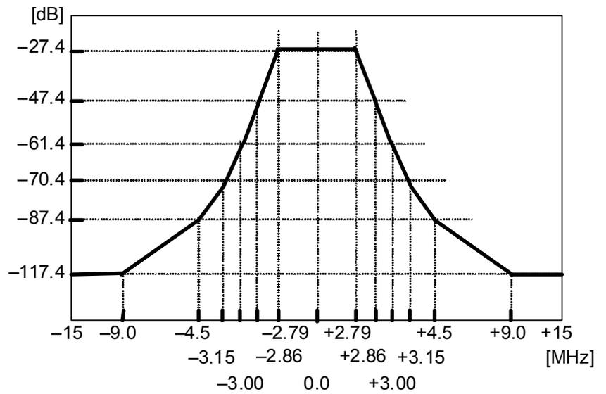
**Figure 2.5.1-6 Transmission Spectrum Mask**
