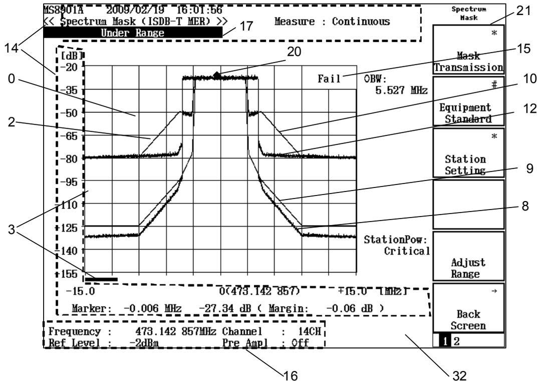
Figure 2.14.2-10 Spectrum Mask screen color layout (Brazil)
