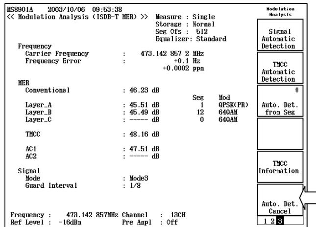
Figure 2.10.4-2 Canceling automatic detection of signal parameters
