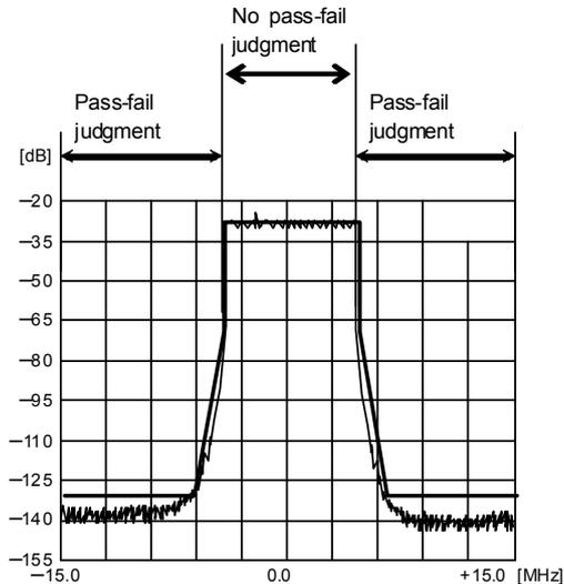
**Figure 2.5.1-11 Spectrum mask pass fail judgment range
