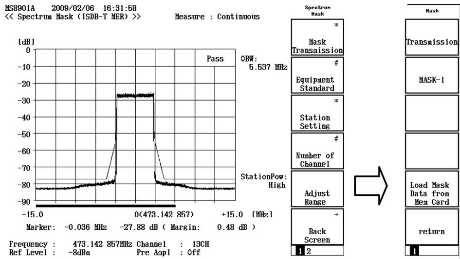
Figure 2.5.2-11 Loading spectrum mask data
