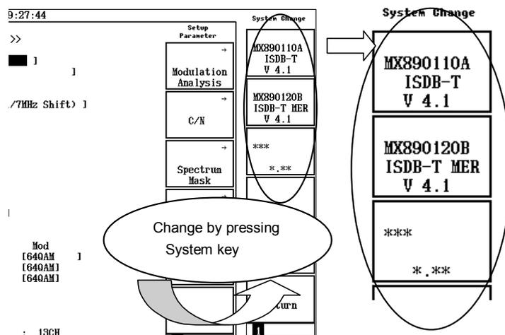
Figure 2.1.4-2 Soft key menu for system selection
