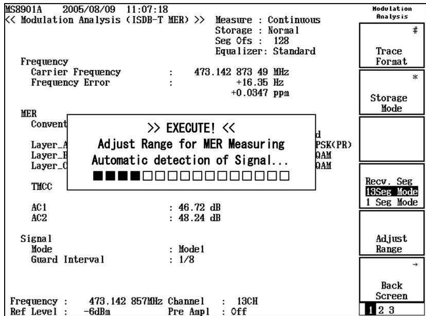
Figure 2.2.6-7 Automatic detection (auto range adjustment by the modulation error ratio)
