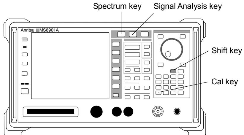
Figure 2.1.3-1 Front panel keys used in calibration
