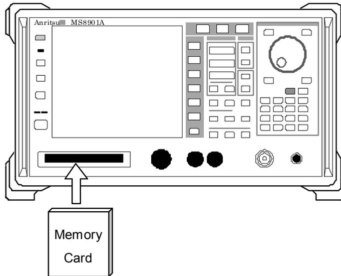
**Figure 2.5.4-6 Insertion of memory card to the MS8901A**
