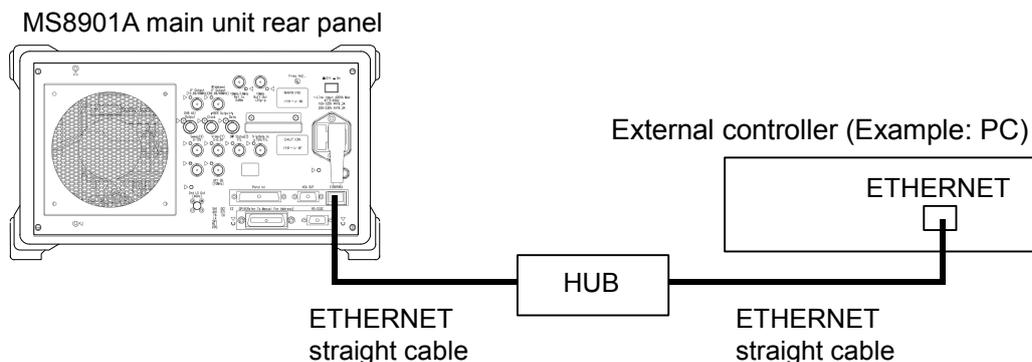
Figure 3.1.3-1 ETHERNET connection example (using straight cable)
