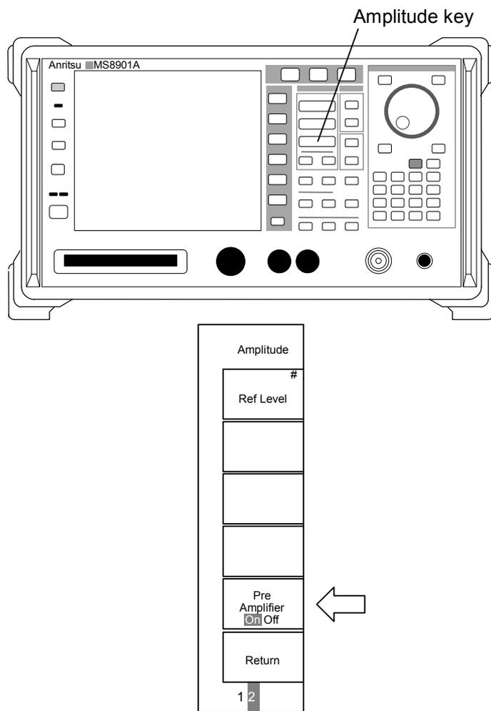
Figure 2.2.10-1 Preamplifier control
