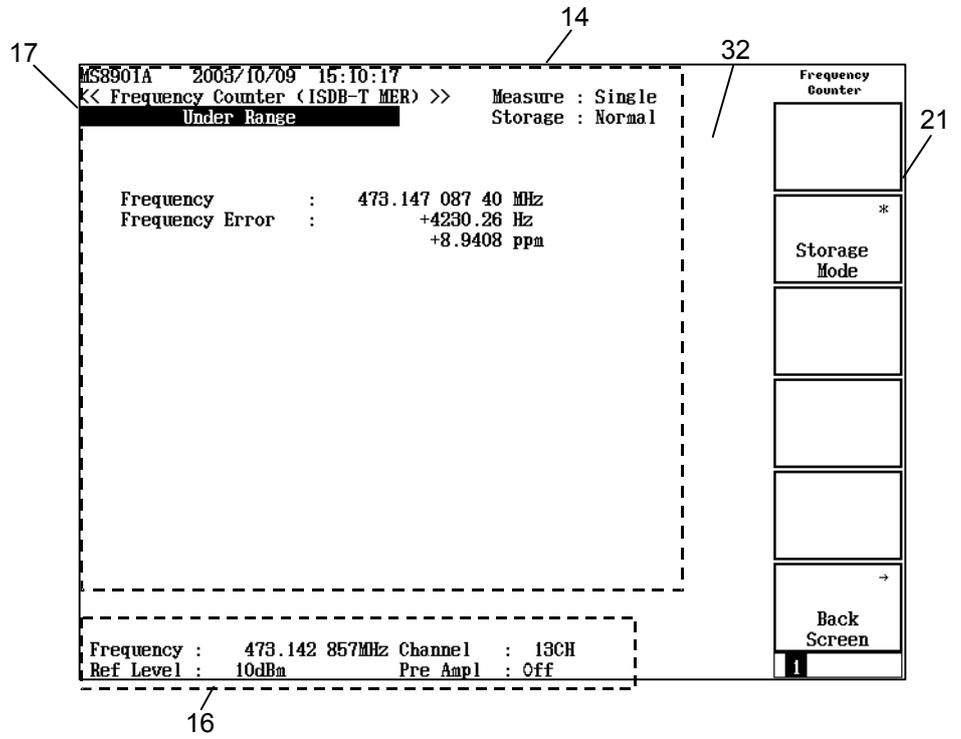
Figure 2.14.2-11 Frequency Counter screen color layout
