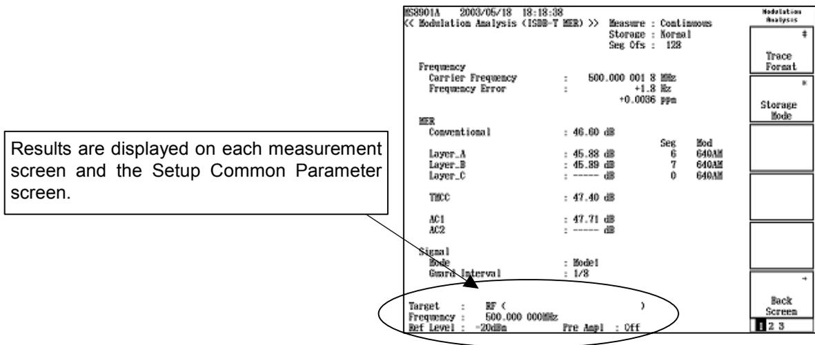
Figure 2.8.14-1 Measured results display on Modulation Analysis screen
