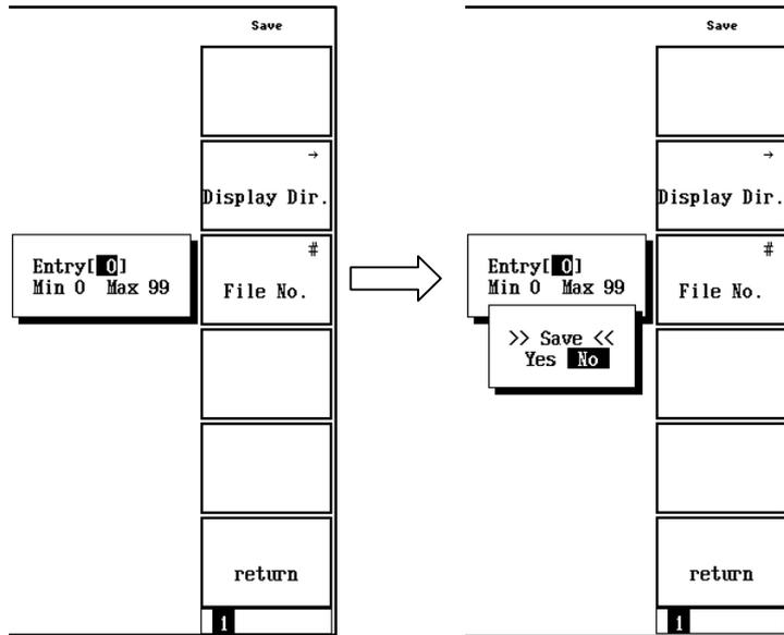
Figure 2.13.1-3 Inputting file numbers directly and saving
