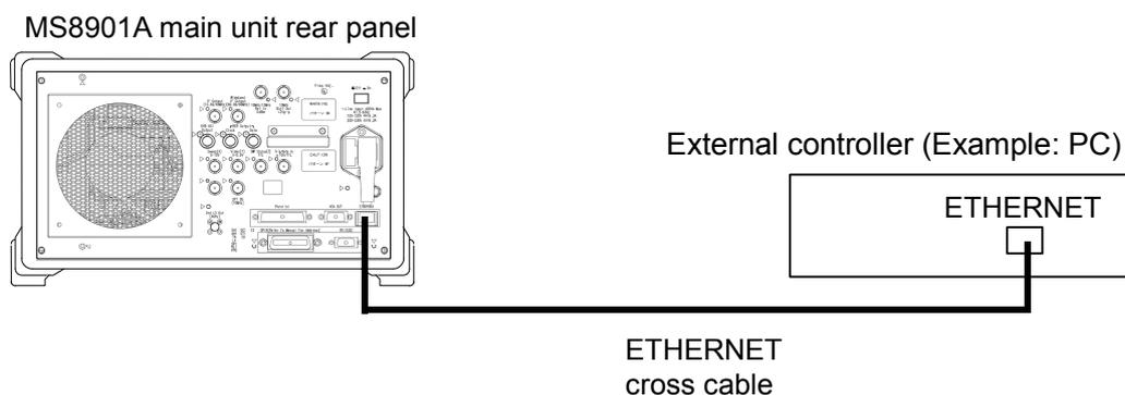
Figure 3.1.3-2 ETHERNET connection example (using cross cable)
