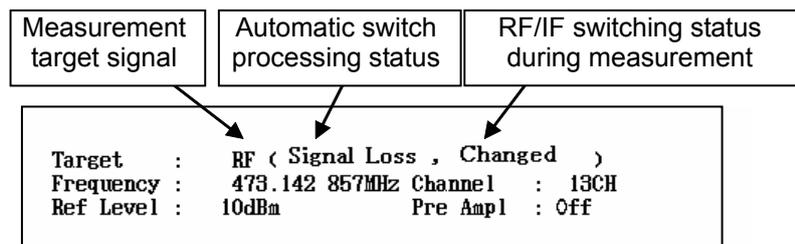
Figure 2.8.14-2 RF/IF measured results display
