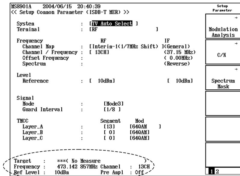
Figure 2.8.1-1 Setup Common Parameter screen (RF/IF switch function enabled)
