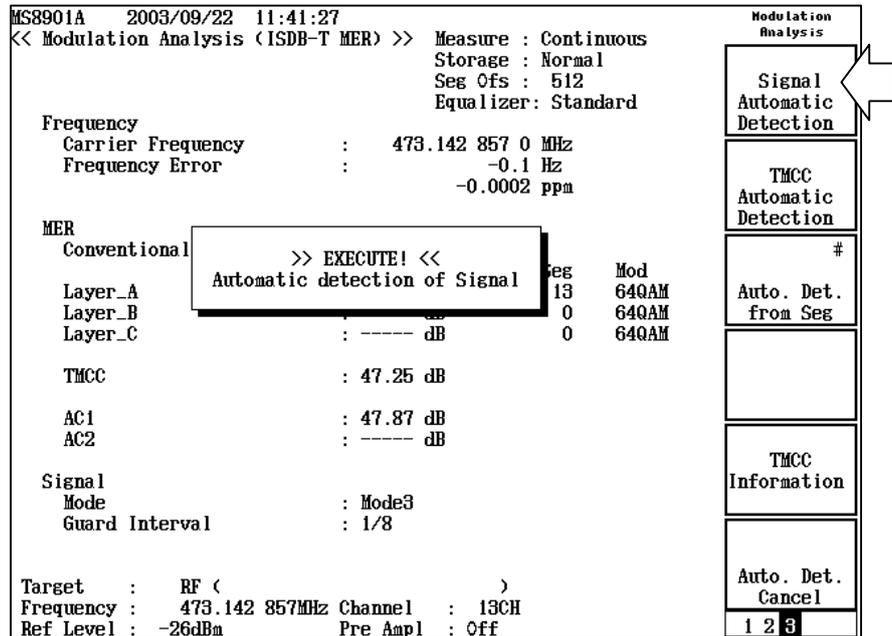
Figure 2.10.1-1 Executing automatic detection of signal parameters
