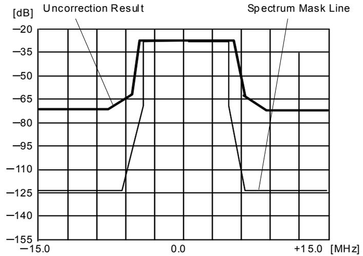
**Table 2.5.5-2** Displayed waveform when Last Result is hidden, Un-correction Result is displayed, and Filter Data is hidden
