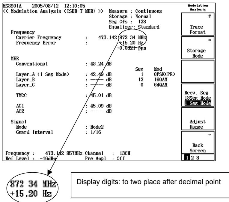
Figure 1.2.2-2 When the Option for the Modulation Frequency Measurement Accuracy is Installed
