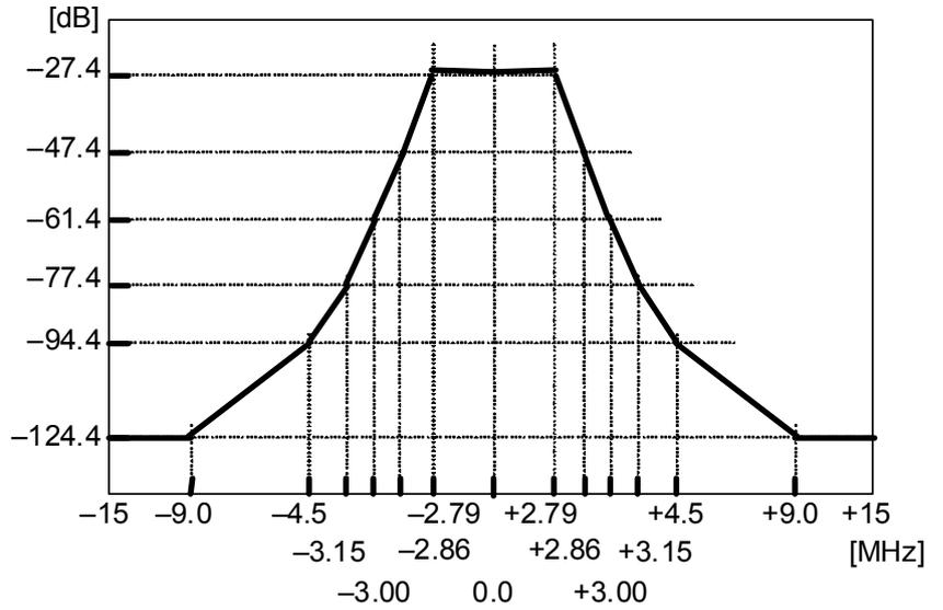
**Figure 2.5.1-5 Transmission Spectrum Mask**
