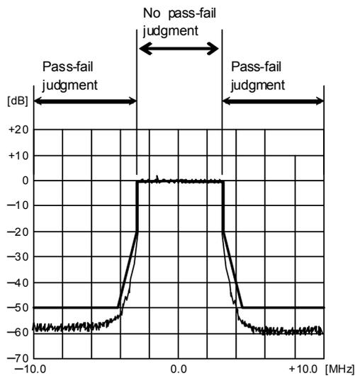
Figure 2.5.1-9 Spectrum mask pass fail judgment range (Equipment Standard: Type A)
