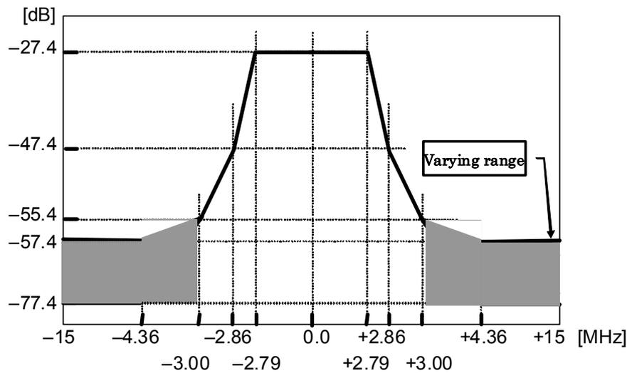
Figure 2.5.1-4 Transmission Spectrum Mask (Equipment Standard: Type B)
