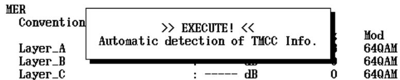
Figure 2.10.1-4 Display during automatic detection of TMCC
