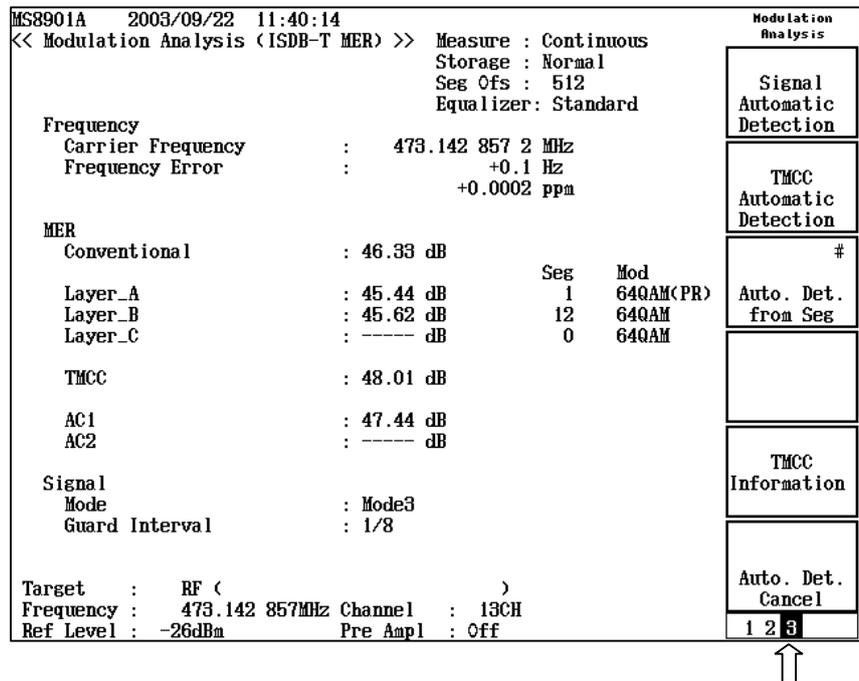
Figure 2.10-1 Modulation Analysis screen (when third menu page open)
