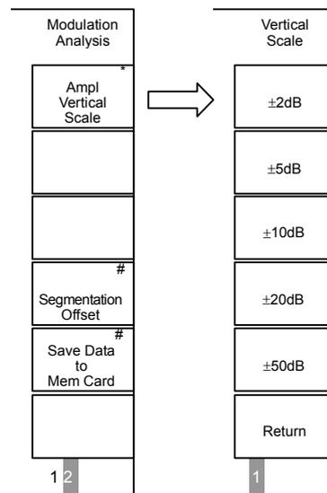
Figure 2.3.3-2 Relative level axis settings
