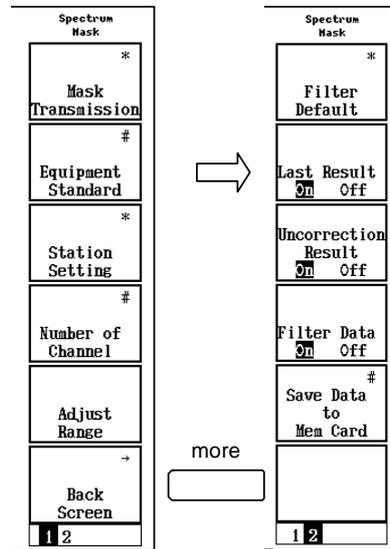
Figure 2.5.4-1 Filter setting selection
