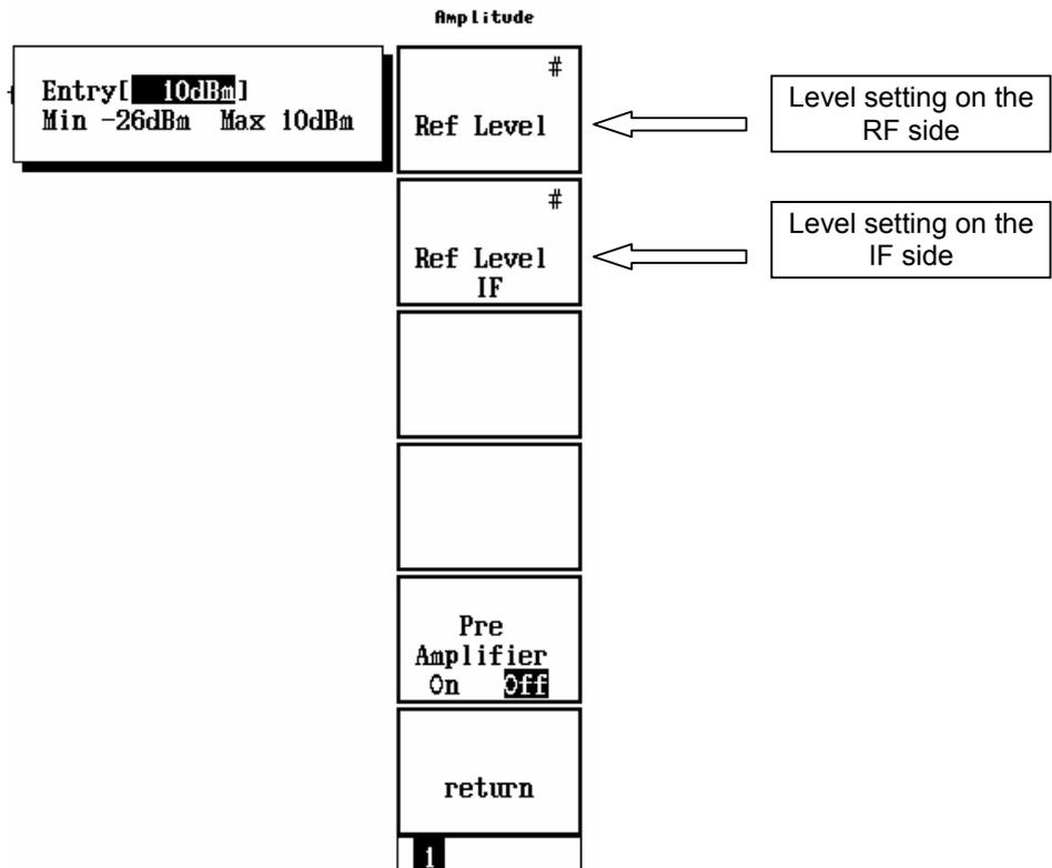
**Figure 2.8.7-2 Settings using Amplitude key (when RF/IF switch function enabled)**
