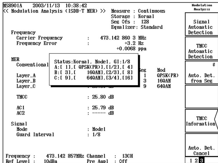
Figure 2.10.2-2 Detection results window on the Constellation screen
