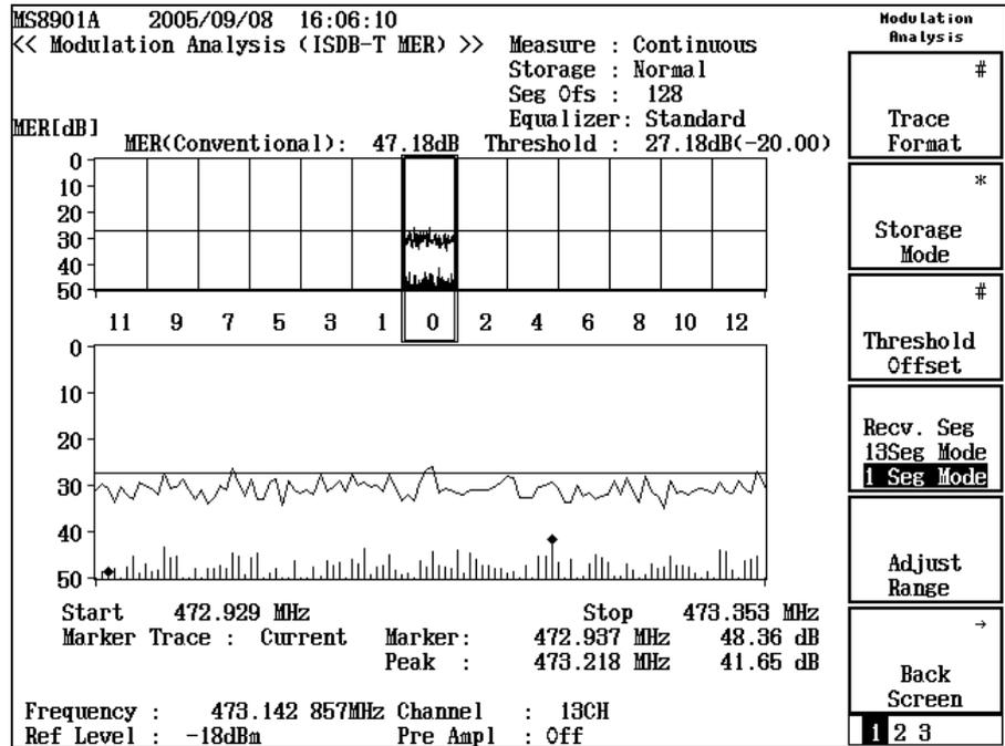
Figure 2.3.5-5 Sub-carrier MER screen at the partial reception
