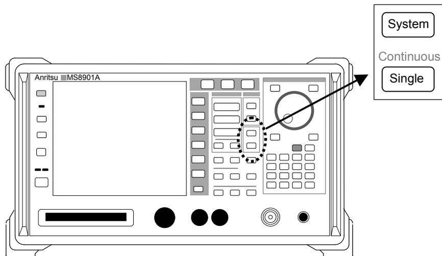
Figure 2.2.11-1 Single key and Continuous key
