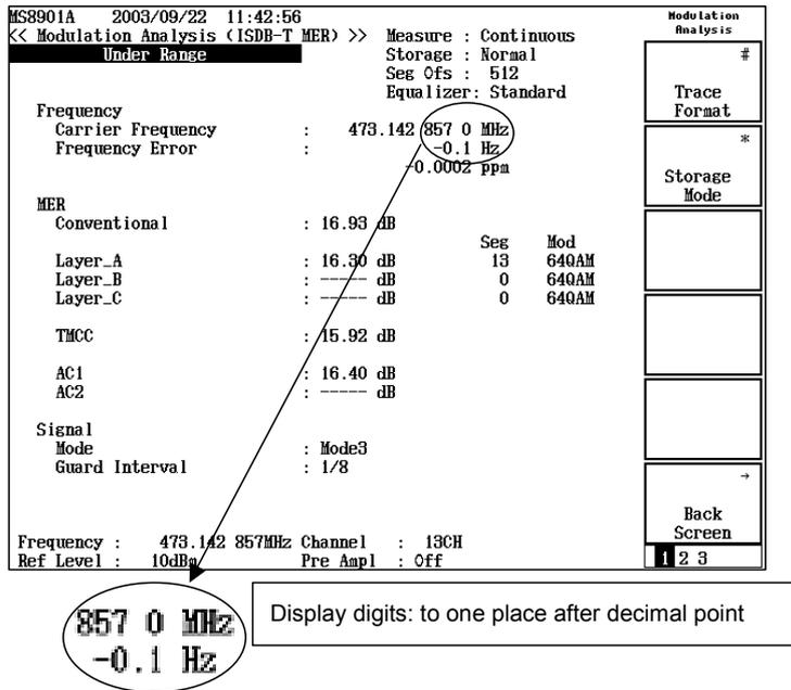
Figure 1.2.2-1 When the Option for Modulation Frequency Measurement Accuracy is not Installed
