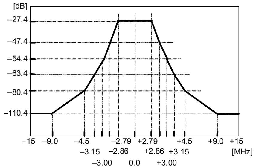
**Figure 2.5.1-7 Transmission Spectrum Mask
