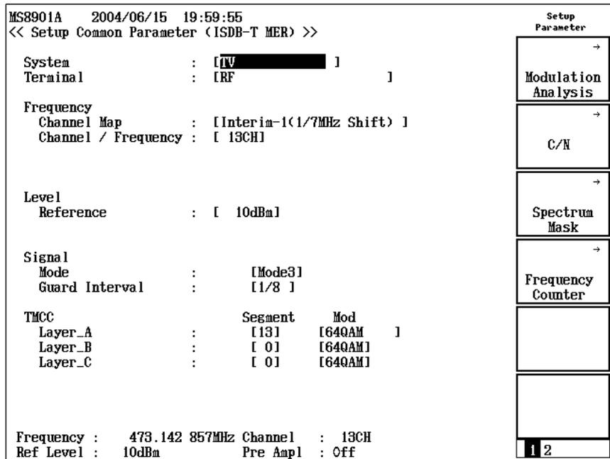
Figure 2.1.2-1 Setup Common Parameter screen as example
