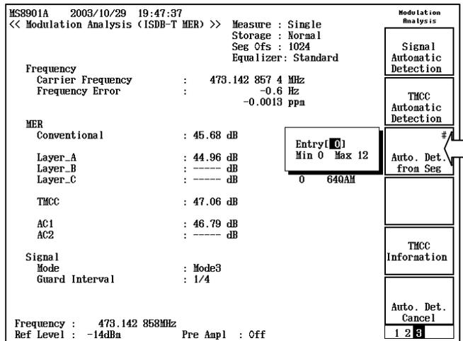
Figure 2.10.3-1 Specifying automatic detection segment on NoTrace screen
