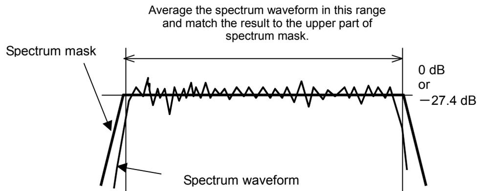
Figure 2.5.1-8 Spectrum mask and spectrum waveform alignment
