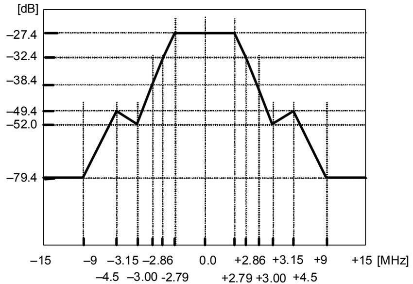
**Figure 2.5.1-16 Example of the Filter Characteristics Waveform Data**
