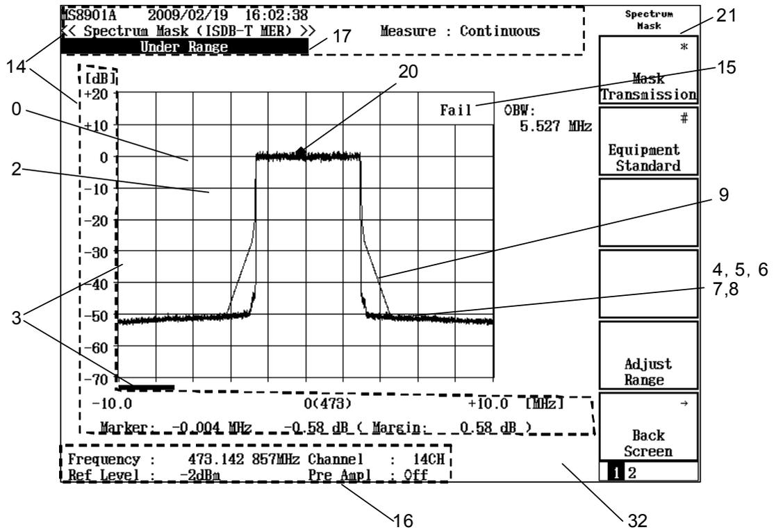
Figure 2.14.2-9 Spectrum Mask screen color layout (Type A, Type B)
