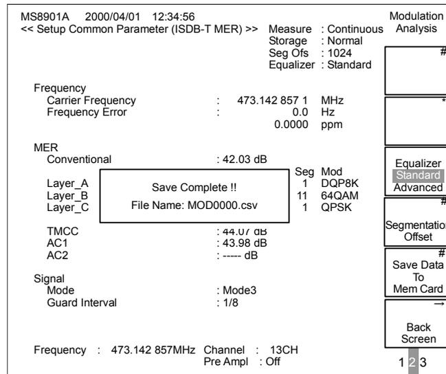
Figure 2.12.2-2 End of numerical value data save
