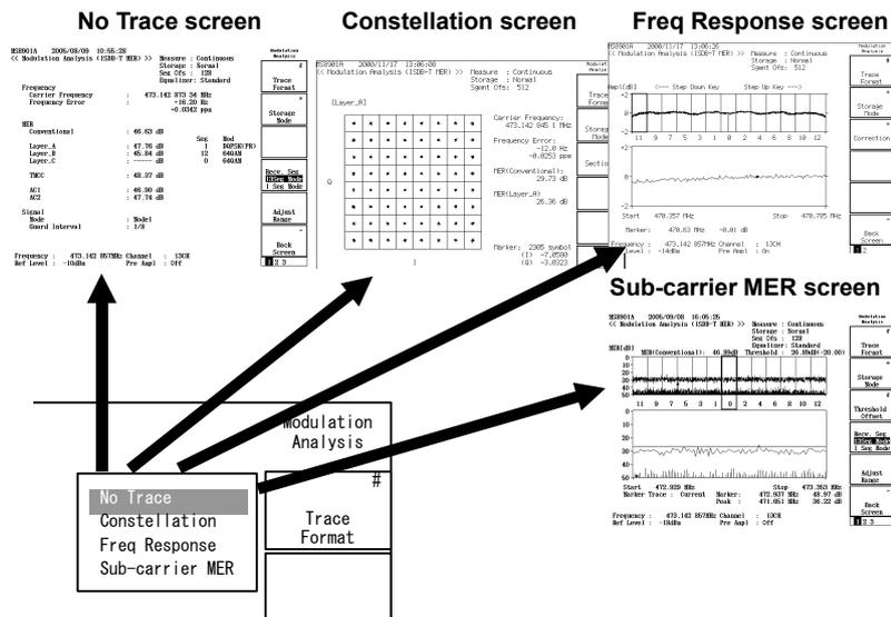
Figure 2.3-2 Switching to the Signal Analysis screen
