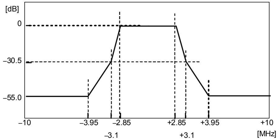
Figure 2.5.2-1 Example of spectrum mask (Equipment Standard: Type A)
