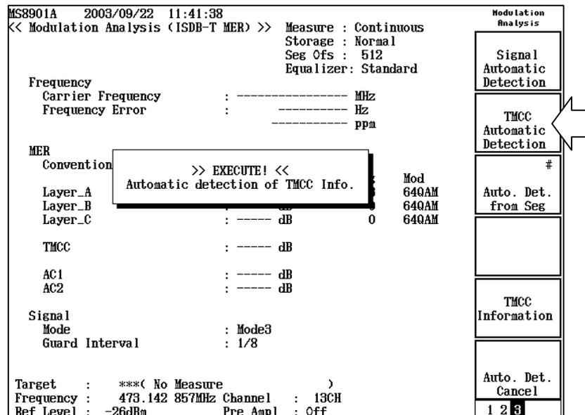
Figure 2.10.1-2 Executing automatic detection of TMCC
