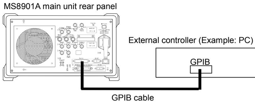
Figure 3.1.1-1 GPIB connection configuration
