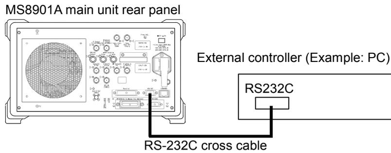
Figure 3.1.2-1 RS-232C connection configuration
