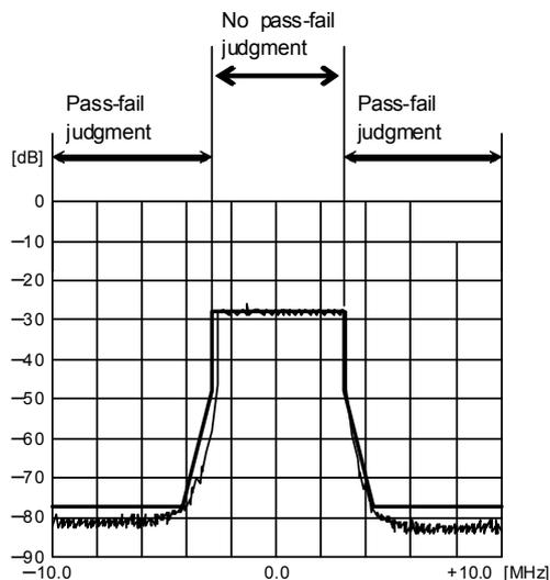
Figure 2.5.1-10 Spectrum mask pass fail judgment range
