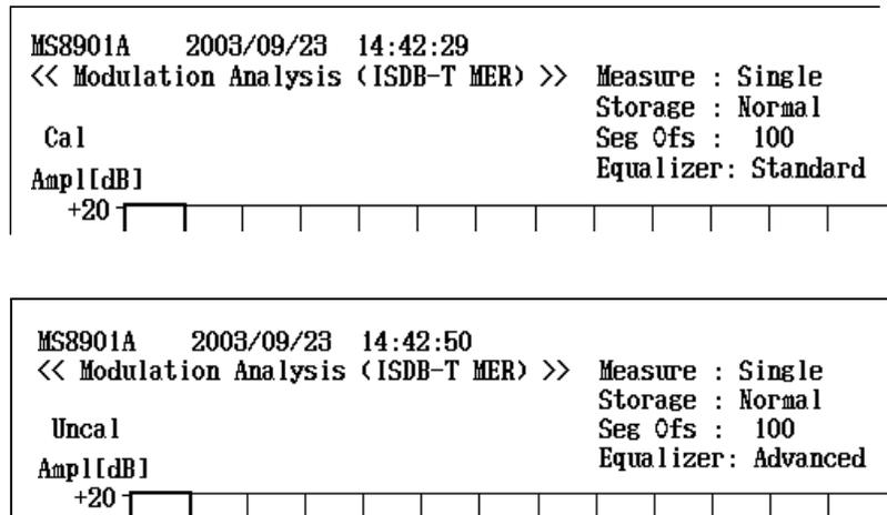
Figure 2.3.3-4 Valid (Cal)/invalid (Uncal) display for correction
