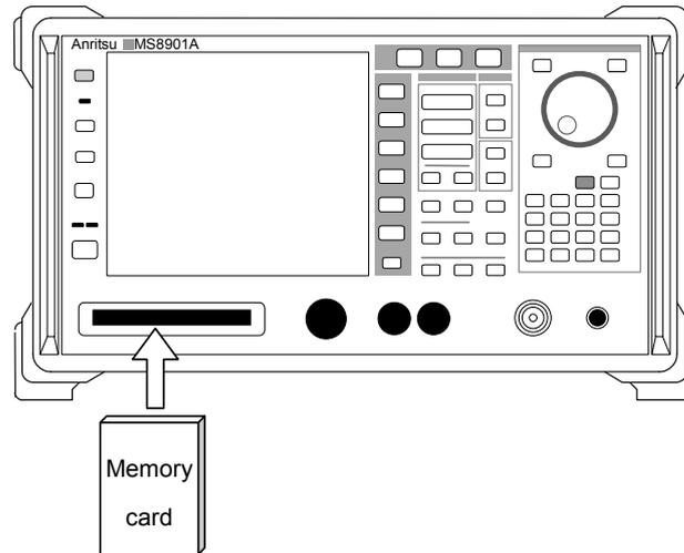
Figure 2.5.2-10 Insertion of memory card to the MS8901A
