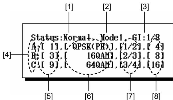
Figure 2.10.2-3 Detection results window details
