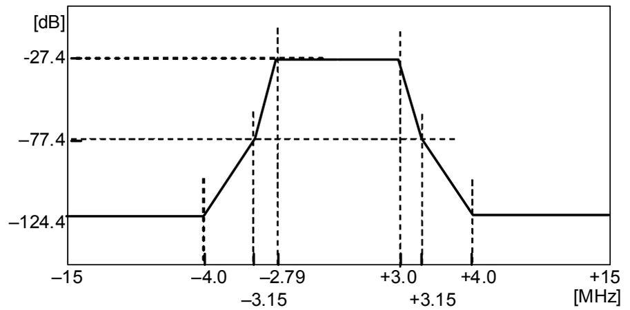
Figure 2.5.2-7 Example of spectrum mask (Equipment Standard: Brazil)
