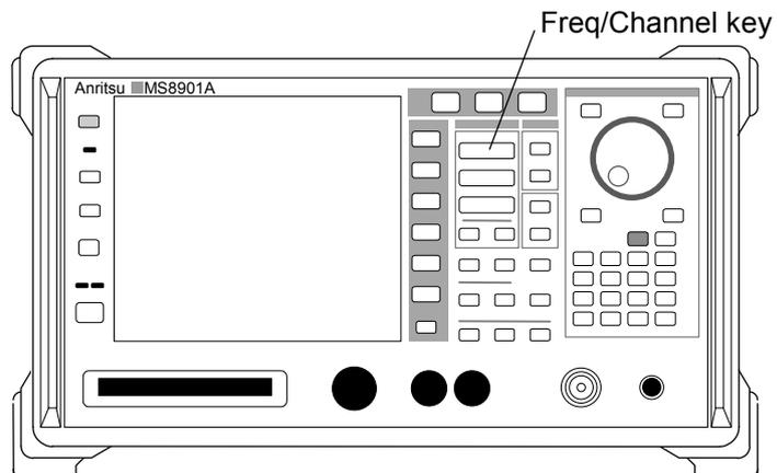
Figure 2.2.3-3 Freq/Channel key
