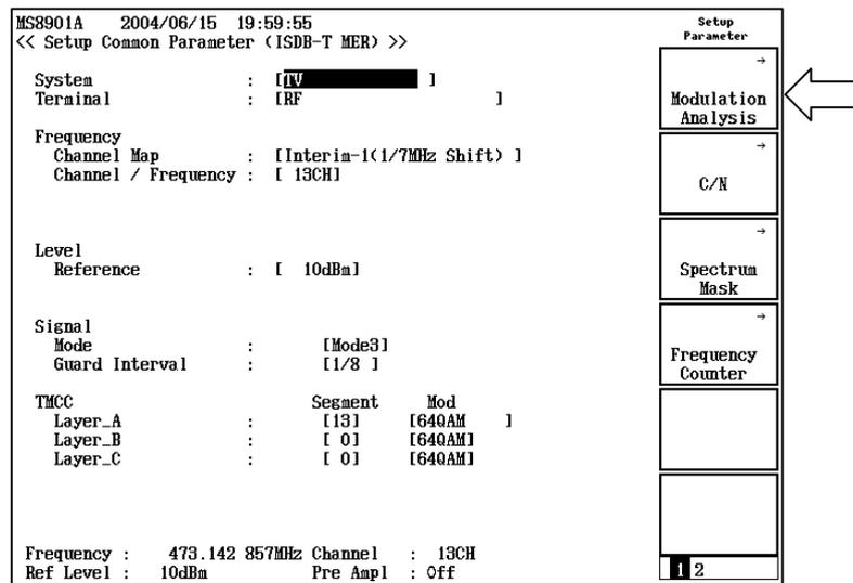
Figure 2.3-1 Setup Common Parameter screen
