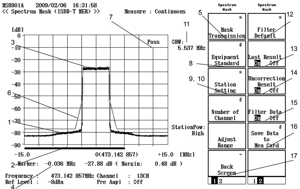
Figure 2.5.1-1 Spectrum Mask screen
