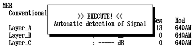
Figure 2.10.4-1 Display during automatic detection of signal parameters
