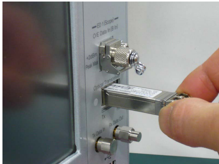
Figure 2.8.1-1 Installing Optical Transceiver
