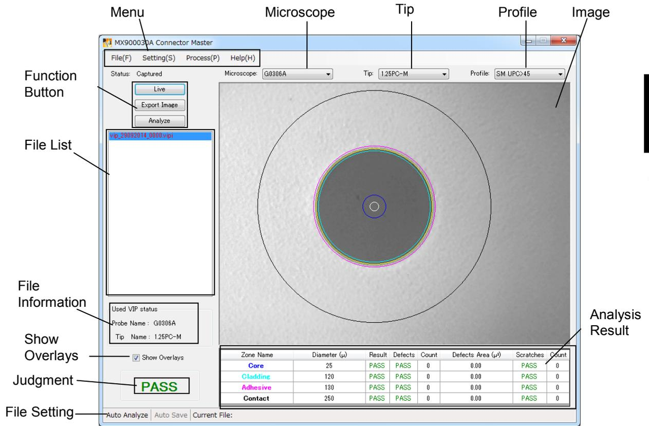
Figure 3.2-1 Components of the Main Window
