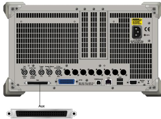
Fig. 2.6.4-1 Output connector location
