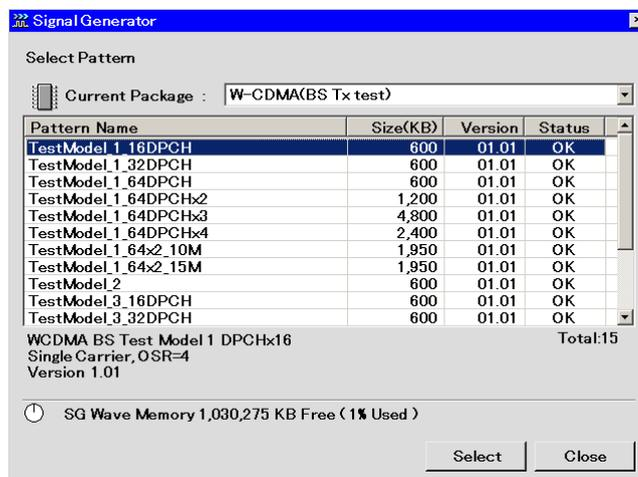
Fig. 2.4.3-1 Selecting waveform pattern to be deleted
