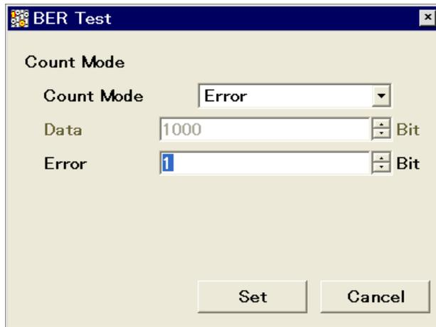
Fig. 3.5-7 Measurement error bit count setup window
