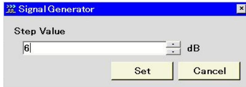
Fig. 2.3.4-1 Output level step setup window
