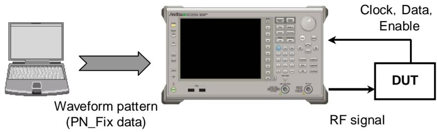
**Fig. 3.8-6 BER measurement using PN\_Fix data**
