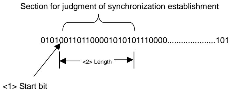
**Fig. 3.9-6 Setting method for section judged for synchronization establishment**
