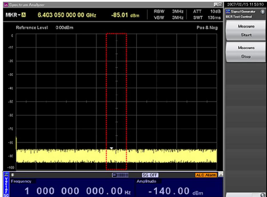
Fig. 2.7.1-1 BER measurement control screen
