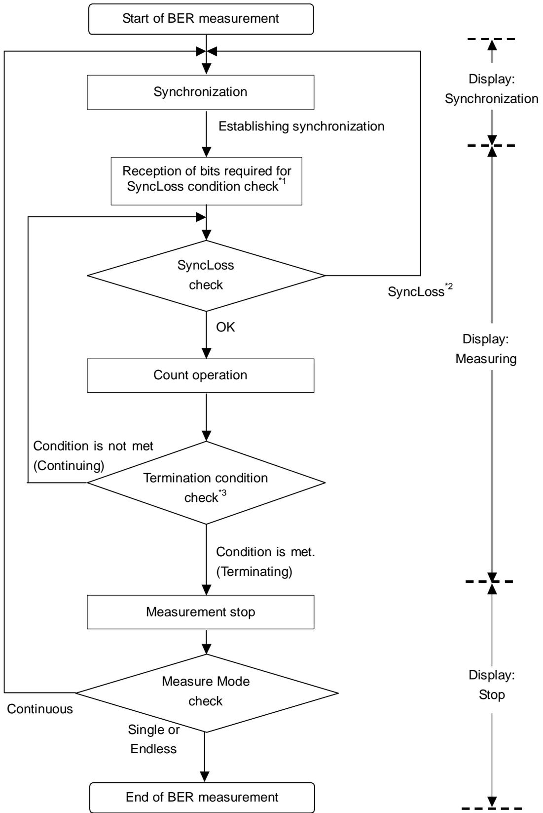
Fig. 3.10-2 When Auto Resync is set to On
