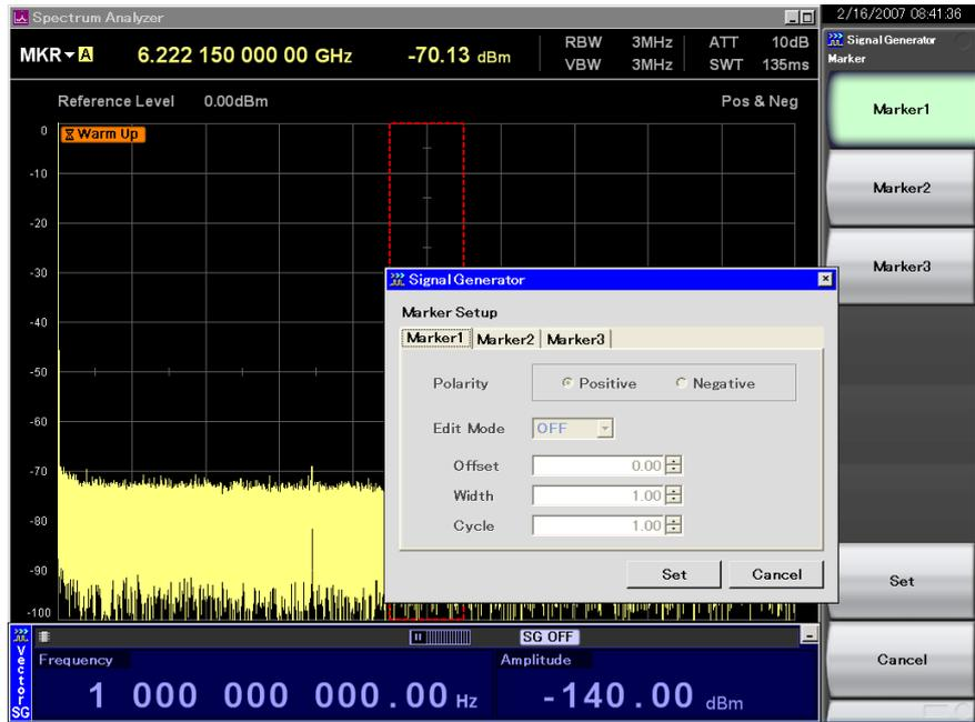
Fig. 2.6.4-2 Marker output setup screen
