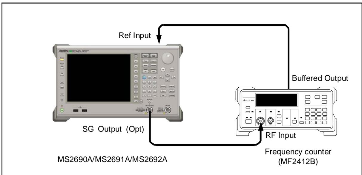
Fig. 4.2.1-1 Frequency test
