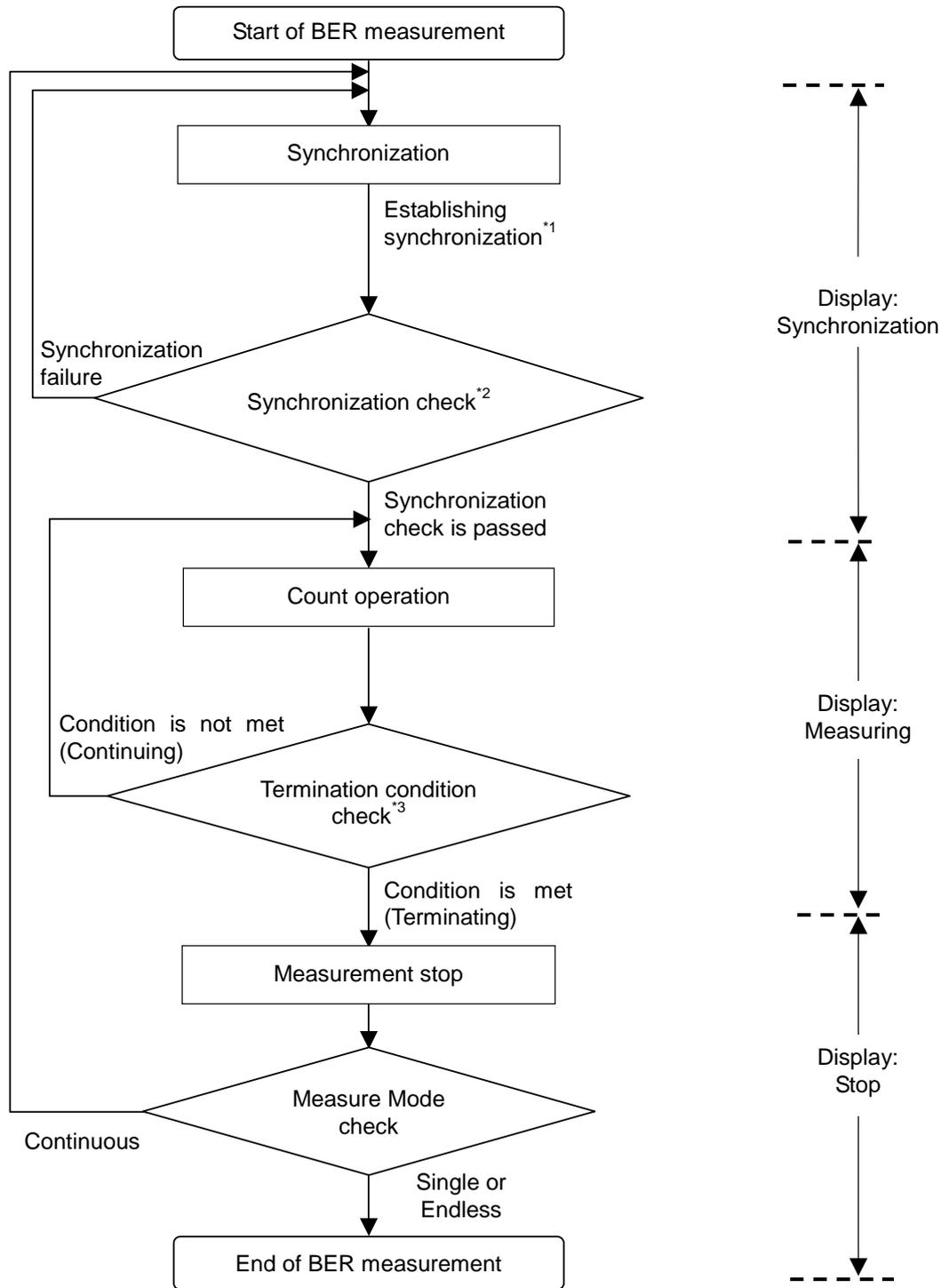
Fig. 3.10-1 When Auto Resync is set to Off
