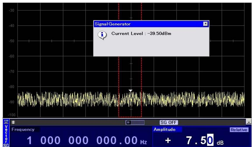
Fig. 2.3.6-2 Output level confirmation window
