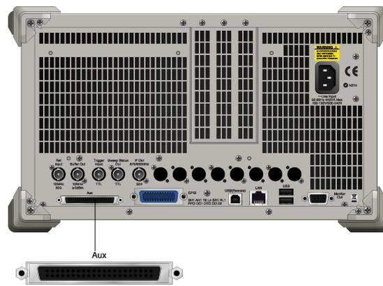
Fig. 2.6.4-1 Output connector location
