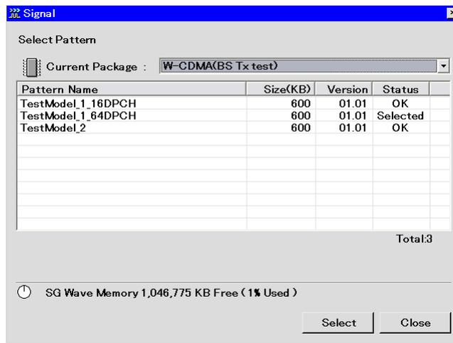
Fig. 2.4.2-2 Status display of selected waveform patterns
