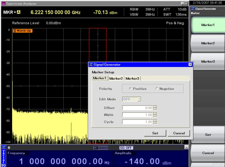
Fig. 2.6.4-2 Marker output setup screen
