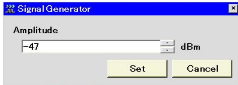
Fig. 2.3.2-1 Output level setup window
