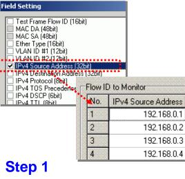
Extract each ONU signal from received upstream signal using IP address as ID.
