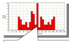
In addition to normal Delay measurement, measurement of Delay distribution is also built-in for statistical verification of network randomness.
