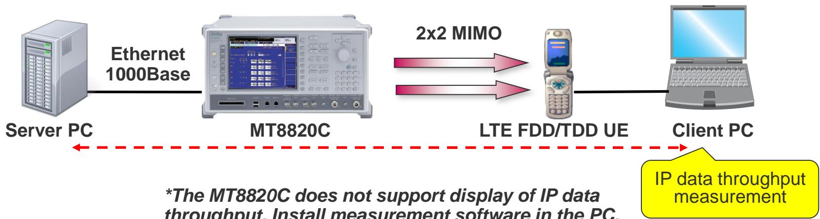
*\*The MT8820C does not support display of IP data throughput. Install measurement software in the PC.*
