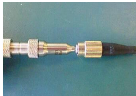
Connected to OTDR output port ferrule endface
