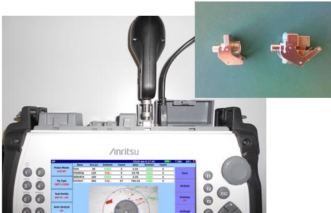
Connected to OTDR output port ferrule endface
