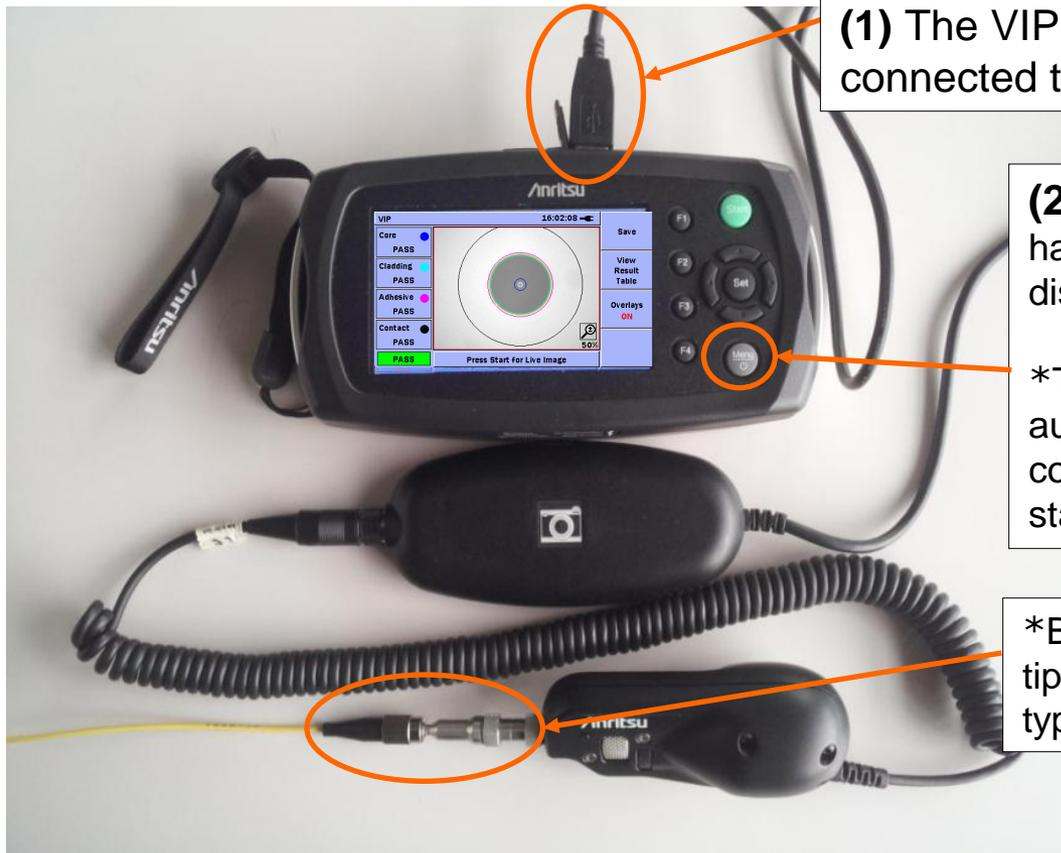
**(1)** The VIP USB terminal is connected to the MT9090A's USB port.
