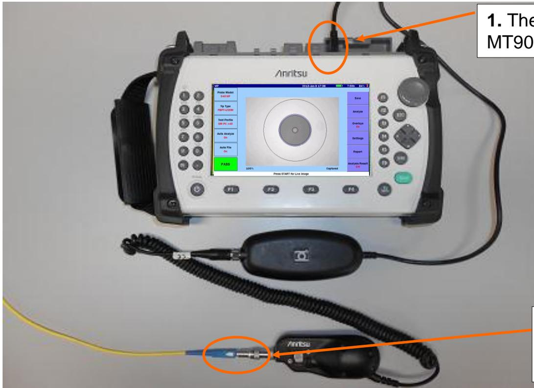
1. The VIP USB terminal is connected to the MT908x series instrument's USB port.
