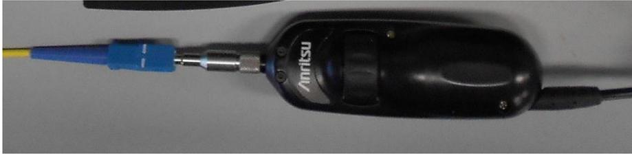
Tips are connected to the end of the VIP based on the shape of connector (adapter) to be connected. This unit comes standard with 8 types of tips.
