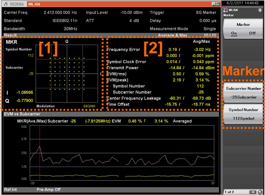
The dispersion of characteristics is measured easily using simultaneous display of maximum and average values.
