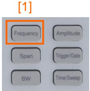
Front-panel function keys switch to setting screens.
