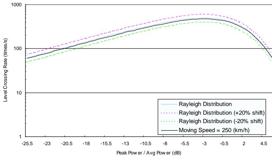
**Level Crossing Rate (Moving Speed = 250 km/h)**
