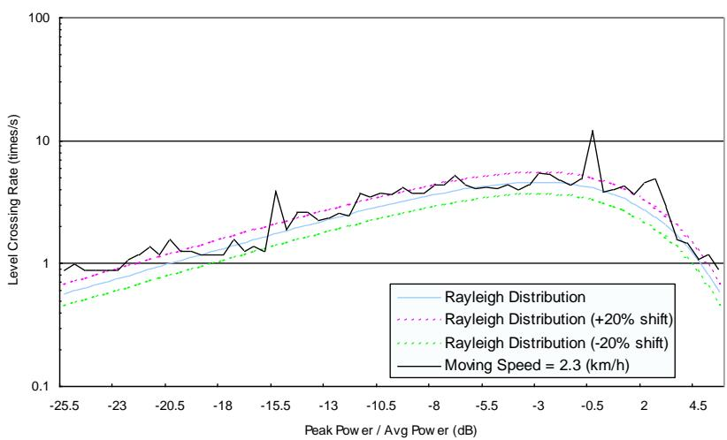
**Level Crossing Rate (Moving Speed = 2.3 km/h)**
