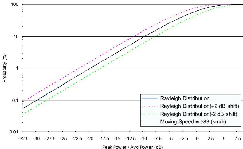
Cumulative Distribution (Moving Speed = 583 km/h)
