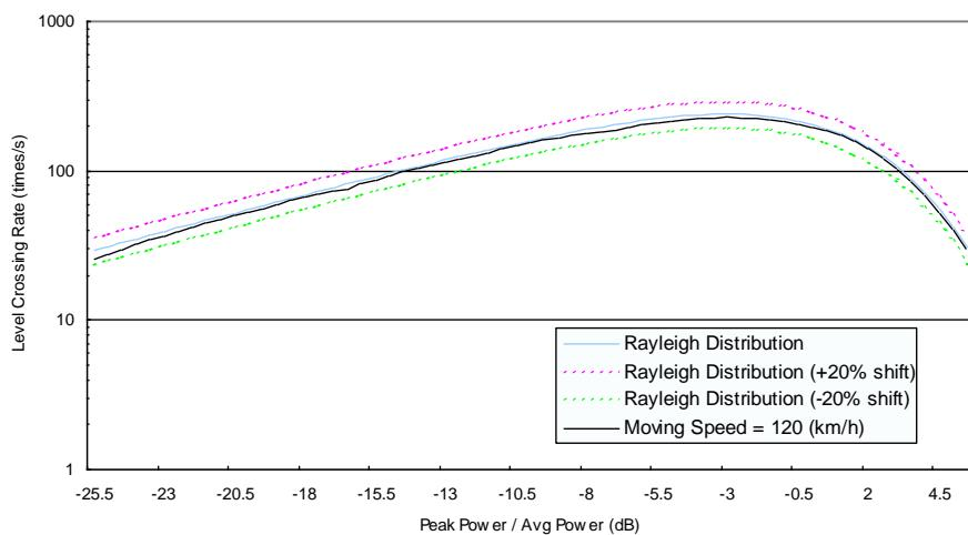
**Level Crossing Rate (Moving Speed = 120 km/h)**
