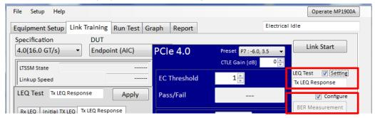
b. Set **CTLE Gain** to **0** (zero) on the BER Measurement panel.
