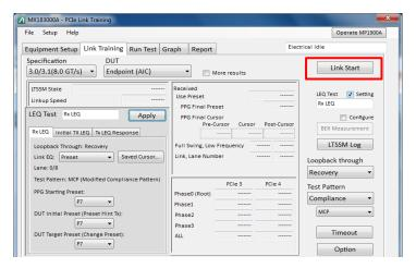
When LTSSM State is Loopback.Active.Lead, click on Saved Cursor button on LEQ Test window.
