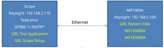
\* TCP/IP cannot be used when the GRL software is installed on a Tektronix scope. Set the GPIB address as "GPIB8::1::INSTR".
