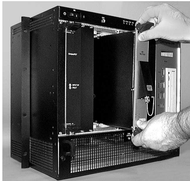
Figure 2-9: cPCI Module Installation
