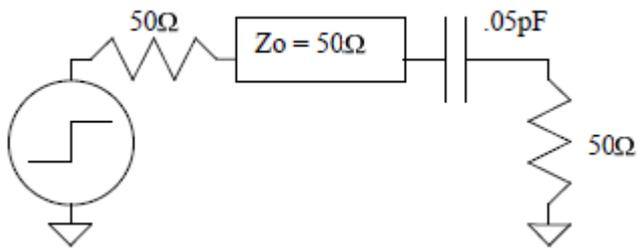
This is a serious impairment that can be modeled as a very small series capacitance or shunt inductance. Only the high frequency content of the data pattern will pass through the impairment, producing pulses where the crossing point of the eye diagram used to be. The center of the eye pattern is completely closed. Damaged connectors and cables can often cause this effect.
