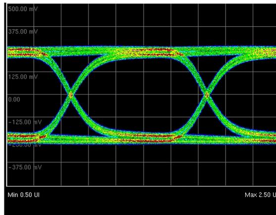
It is easy to see this effect looking at the pulse pattern. The peak-to-peak amplitude of 1010 sequences is less than that of a 111000 sequence, because the 1010 pattern has more high frequency content than the 111000 pattern and is therefore attenuated more by the cable.
