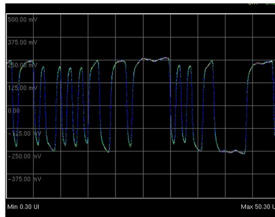
In conclusion, the eye pattern is a useful tool for troubleshooting signal impairments. Careful inspection of the shape of the eye pattern can reveal the cause of the signal distortion in a transmission line. Removal of the impairments can be an eye opening experience.
