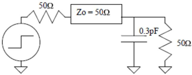
Shunt capacitance or series inductance can cause a distortion of the eye diagram as shown below.
