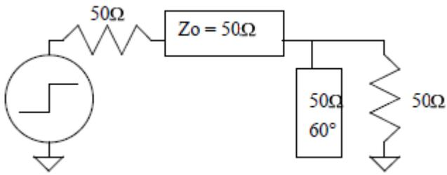
The eye pattern below is caused by a shunt open stub that is 60 degrees long at the bit rate. The stub can cause overshoot, ringing and oddities in the crossing point of the eye. The amount of distortion increases with the length of the stub.
