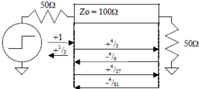
Because of the reflection at the  $100\ \Omega$  transmission line and  $50\ \Omega$  load interface, only
