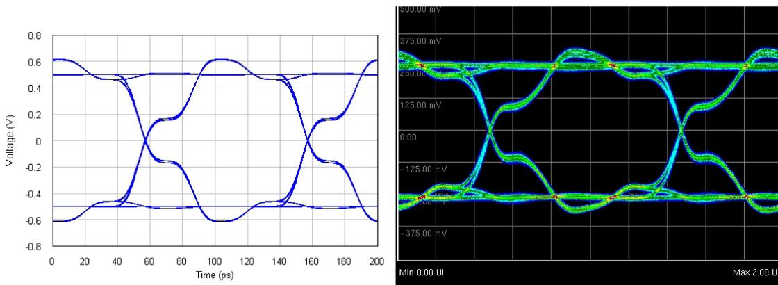
Transmission line stubs can be caused by poorly designed shunt bias circuits. If a shunt bias element such as an inductor is not placed directly on the transmission line, there will be an unwanted stub in the circuit.
