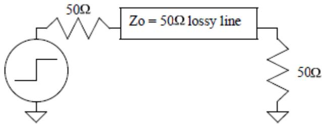
Lossy transmission lines distort the eye pattern because there is more loss at high frequencies than low frequency. Alternating zeroes and ones will be attenuated more than long stretches of consecutive bits. The eye will close up and the zero and one levels will appear thicker and may even split.
