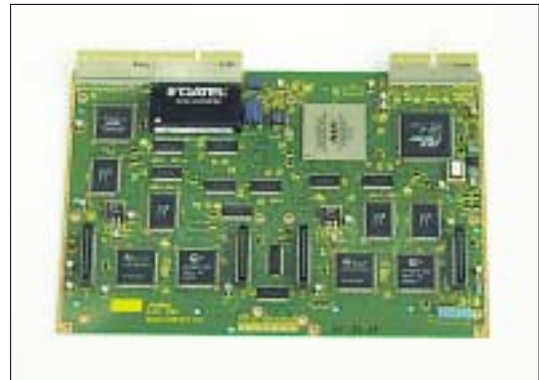
Printed circuit board with lead-free soldering
