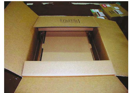
3. The box is closed, creating tension that holds the product, protecting it from shock and vibration.
