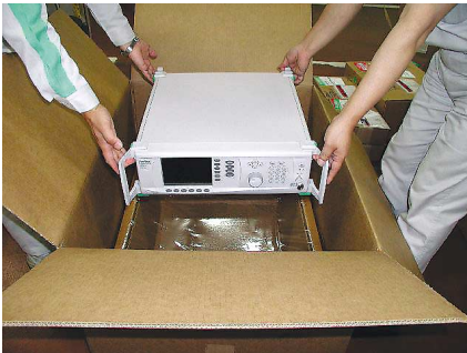
1. Inner cardboard placed in the box to suspend the product in the center of the container.
