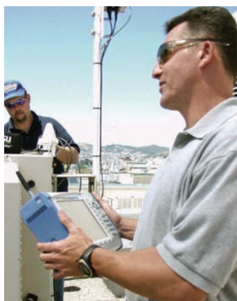
Handheld measuring instruments in use for maintaining wireless base stations
