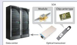
Anritsu's SOA-equipped optical transceiver enables longdistance communication between data centers without degradation of optical signals. New product of chip carrier type SOA smaller than module type assists miniaturization of optical transceivers.
