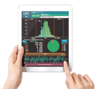
Comprehensive quality management and control system capable of centrally managing the recording of measurement data and the operating history of multiple inspection devices
