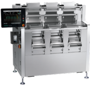
Auto checker (Checkweigher) for capsules for pharmaceutical products. A high accuracy of \pm 0.5 mg makes it suitable for performing full inspection when strict mass control is required, such as for anticancer drugs and immunosuppressive drugs.
