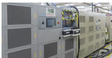
Regenerative power supply test equipment
