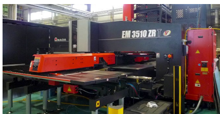
Sheet metal FMC system
