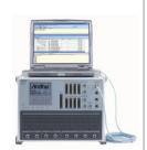
LTE-capable MD8430A Signaling Tester
