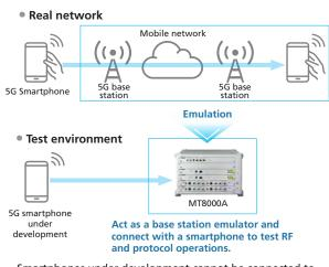
Smartphones under development cannot be connected to the base stations in real network. Anritsu's MT8000A emulates a base station and network, connecting to smartphones under development to help engineers debug.
