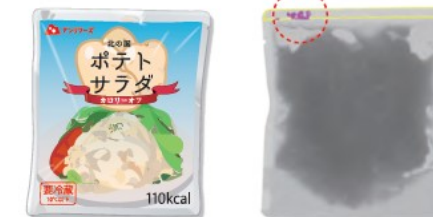
Check for perforation Food packages are inspected to ensure that the contents have not pierced through the sealing area.
