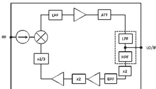
Figure 3 High Performance Waveguide Mixer Block Diagram
