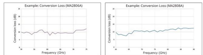
Figure 4 MA2806A/MA2808A Conversion Loss Characteristics
