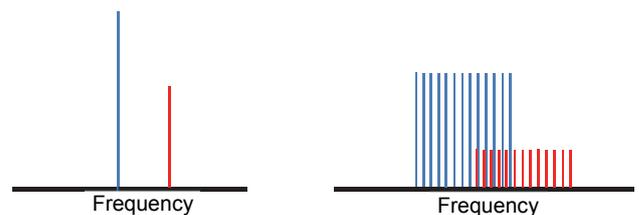
Figure 5 CW Signal and Modulated Signal Spurious
