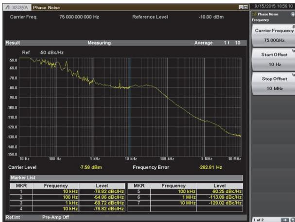
Figure 16 Measured Phase Noise for Input CW 75 GHz Signal
