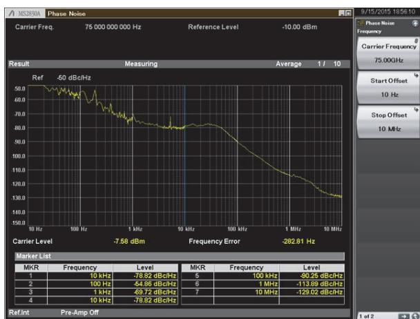
Figure 16 Measured Phase Noise for Input CW 75 GHz Signal
