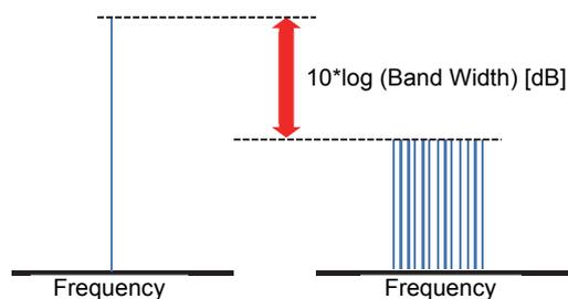
Figure 2 CW and Wideband Signal Spectrum Density
