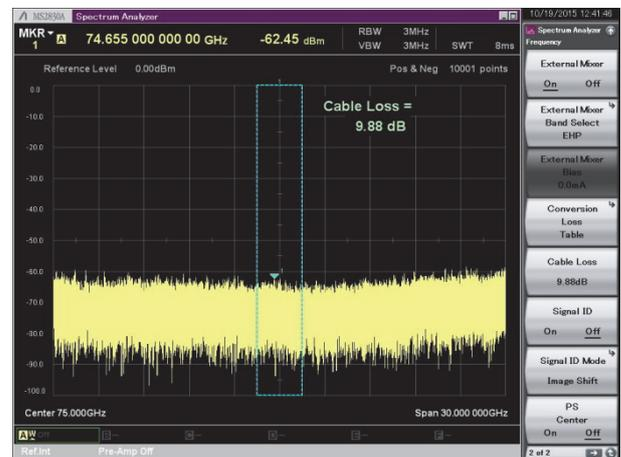
Figure 8 Setting Cable Loss
